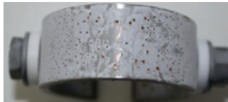
As-received, 45°C, 1.5% strain, 10 g/m 2 salt
