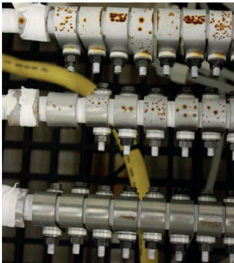
Pitting on specimens at 10 g/m 2 (top), 1 g/m 2 (middle), and 0.1 g/m 2 (bottom)
