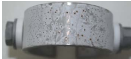
As-received, 45°C, 1.5% strain, 10 g/m 2 salt
