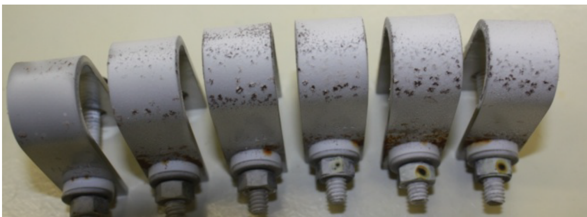
Figure 3-22. Photograph of 10 \text{ g/m}^2 Exposed Type 304 U-Bend Specimens Held at 60 \text{ }^\circ\text{C} [ 140 \text{ }^\circ\text{F} ] for 6.5 Months
