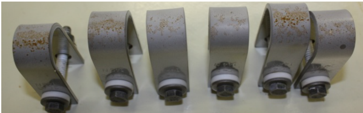
Figure 3-28. Photograph of 1 g/m 2 Exposed Type 304 U-Bend Specimens Held at 52 °C [136 °F] for 8 Months
