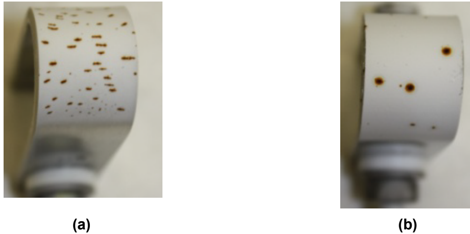
Figure 3-34. Photographs of 10 g/m 2 Type 304 U-Bend Specimens Held at 45 °C [113 °F] and 44 Percent Relative Humidity for (a) Sensitized and (b) As-Received Conditions
