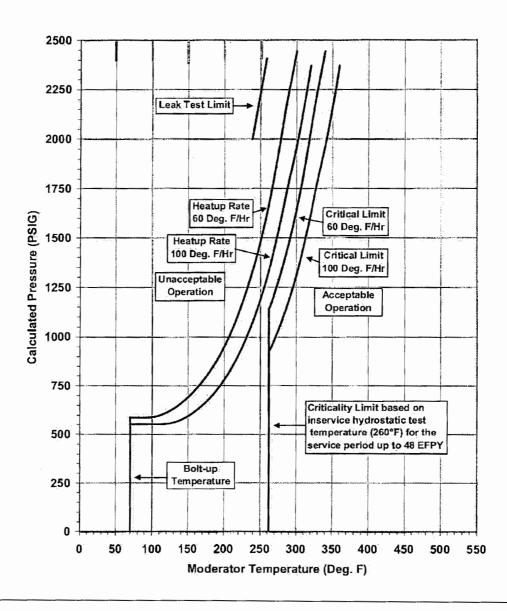
FIGURE 3.4-2 Turkey Point Units 3 & 4 Reactor Coolant System Heatup Limitations (Heatup Rates of 60 and 100°F/hr) Applicable for 48 EFPY (Without Margins for Instrumentation Errors)
