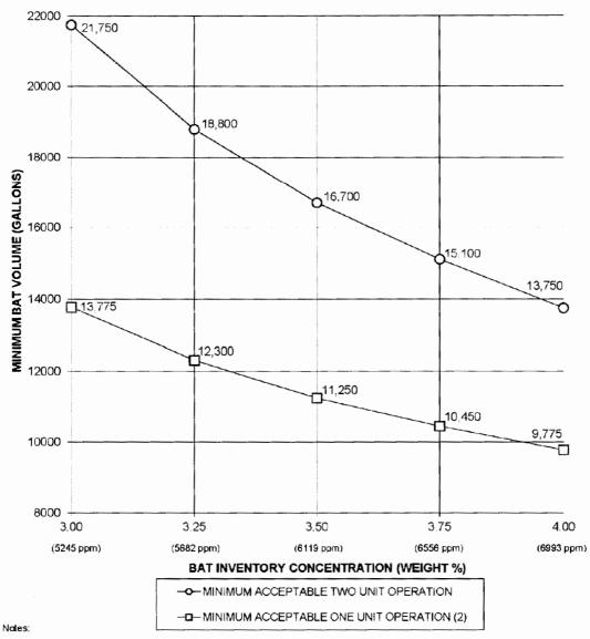
Figure 3.1-2 BORIC ACID TANK MINIMUM VOLUME (1) Modes 1, 2, 3 and 4
