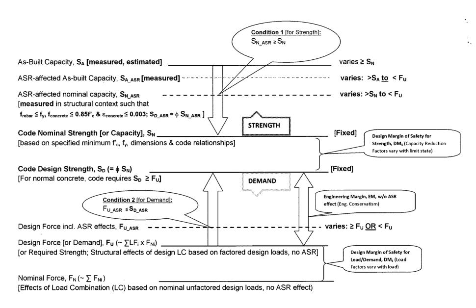
Conceptual Application of Intent of ACI 318-71 Strength Design to ASR-Affected Structures
