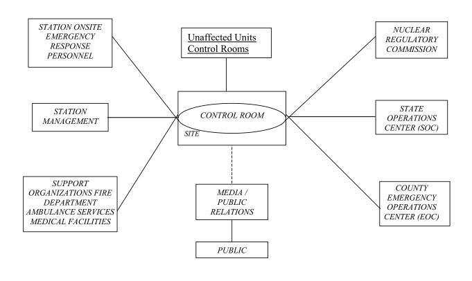
Figure F-1 Emergency Response Facilities Communications Pathway Typical Functional Diagram Unusual Event
