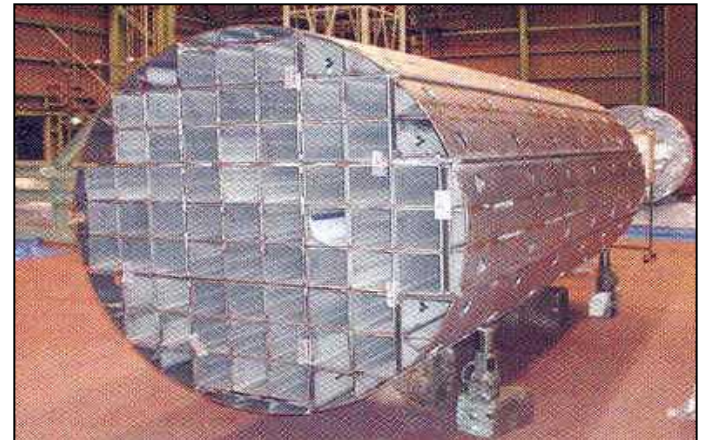
basket made of Al-B 4 C extruded plates for neutron shielding
