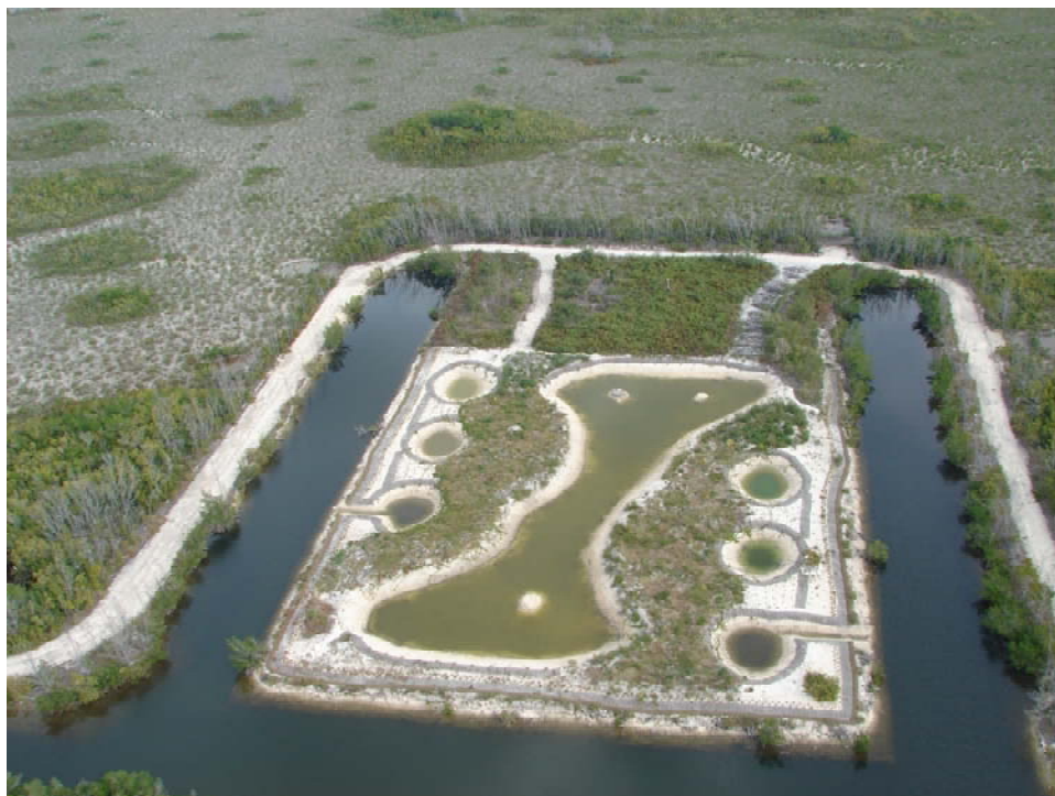
Photograph 12. Aerial view of Everglades Mitigation Bank crocodile sanctuary area following creation of crocodile habitat. Exotic species of vegetation replaced with natives, freshwater ponds excavated and perimeter of peat/marl/sand nesting substrate installed.
