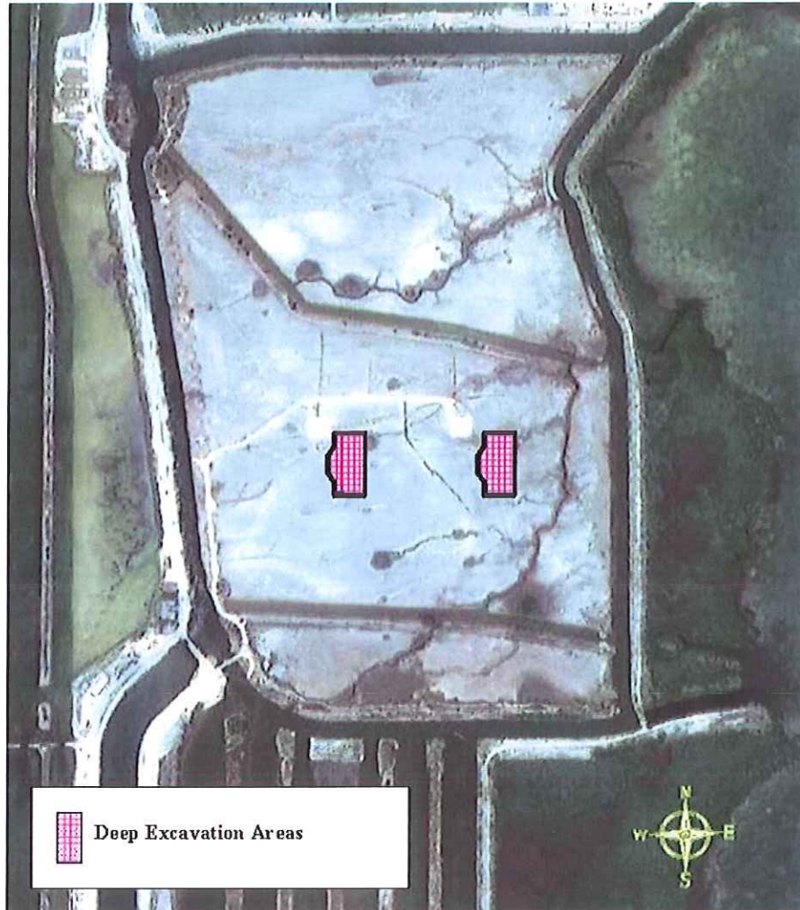
Figure 4 – 1: Turkey Point Units 6 & 7 Deep Excavation Areas
