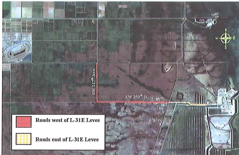
Figure 10 – 1: Turkey Point Units 6 & 7 Temporary Access Roads Improvements and Transmission Structure Pads Along SW 359 th Street
