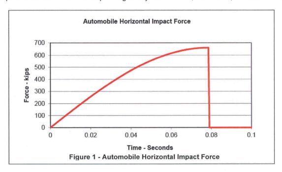
The resistance associated with each of the walls identified in Table 1 is determined, and time history analyses are performed that allow the wall to deform in an elastic-perfectly plastic manner as shown in Figure 2. It was determined that for the walls, the largest ductility factor is 1.10, which is well below the allowable of 10. Further, the ductility factors are adjusted for the added deflection due to the hurricane induced pressures. The ductility factors are shown in Table 2.
