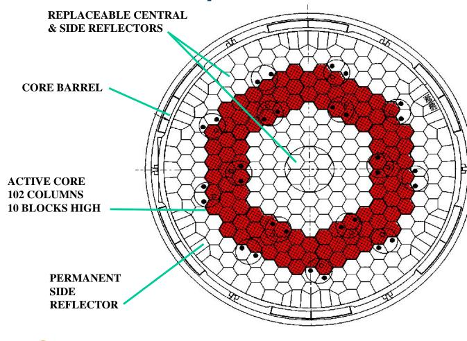
Next Generation Nuclear Plant Modular HTGR utilizes annular core geometry to 1) shorten conduction path 2) enhance surface to volume ratio
