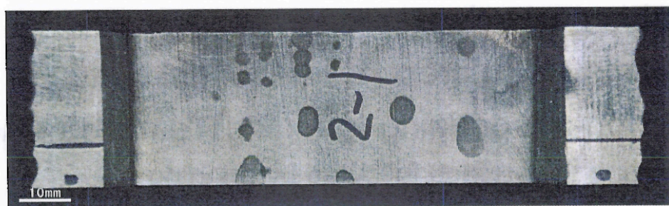
Mockup - gouging showing case hardening locations
