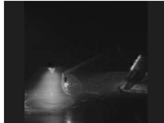
Bad wire position – too high
