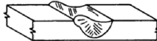
Lateral weld (1/19 slope)
