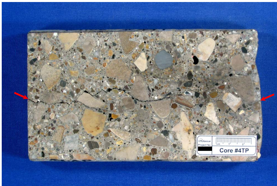
4b. Core #4TP. Note crack (arrows) extends through full length of core.
