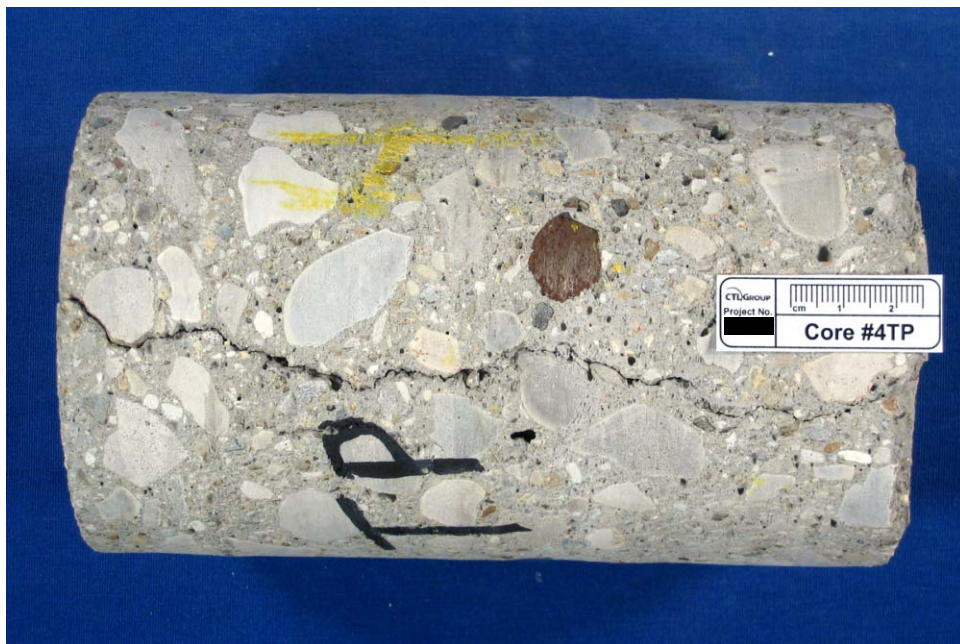
2b. Side view, top surface at left. Note crack extends through full length of core.
