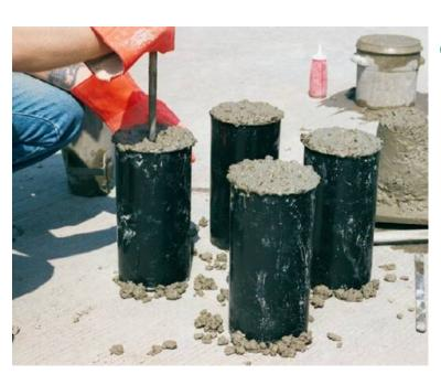
Purpose of Test: To check for adequacy of mix proportions for strength.
