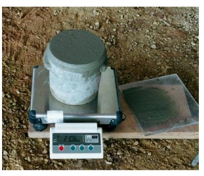
Purpose of Test: To find the weight per cubic foot of fresh concrete, which is used for determining yield and cement factor.
