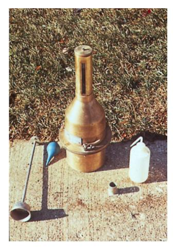
Volumetric Method – ASTM C173 (suitable for all types of aggregate)
