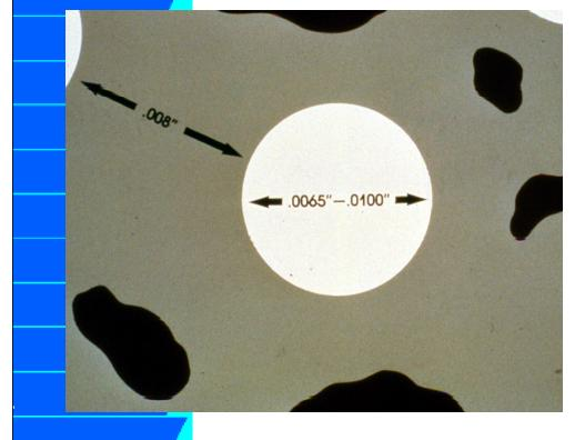
Spacing Factor and Specific Surface are More Important than Total Volume (%) of Air
