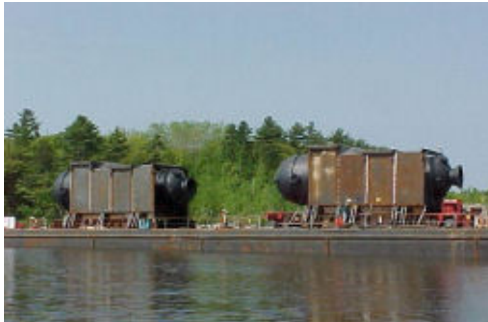
Steam generators en route to Memphis for segmentation prior to disposal.
