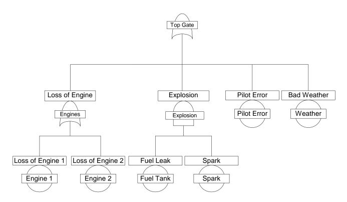
Figure 5-20 Fault Tree Example
