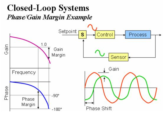
Figure 5-31 Phase/Gain Margin Example
