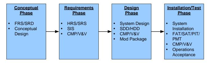
Figure 5-14: Life Cycle Overview of a Digital Upgrade Project
