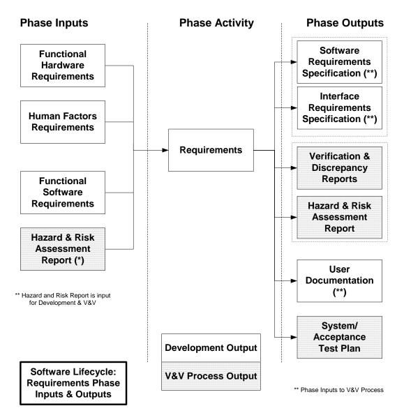
Figure 5-16 IEEE Std 1012 Requirements Phase Activity Inputs and Outputs
