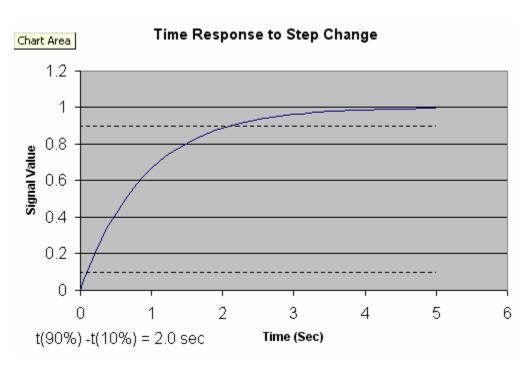
Figure 5-30 Rise Time Sampling Rate Selection Example
