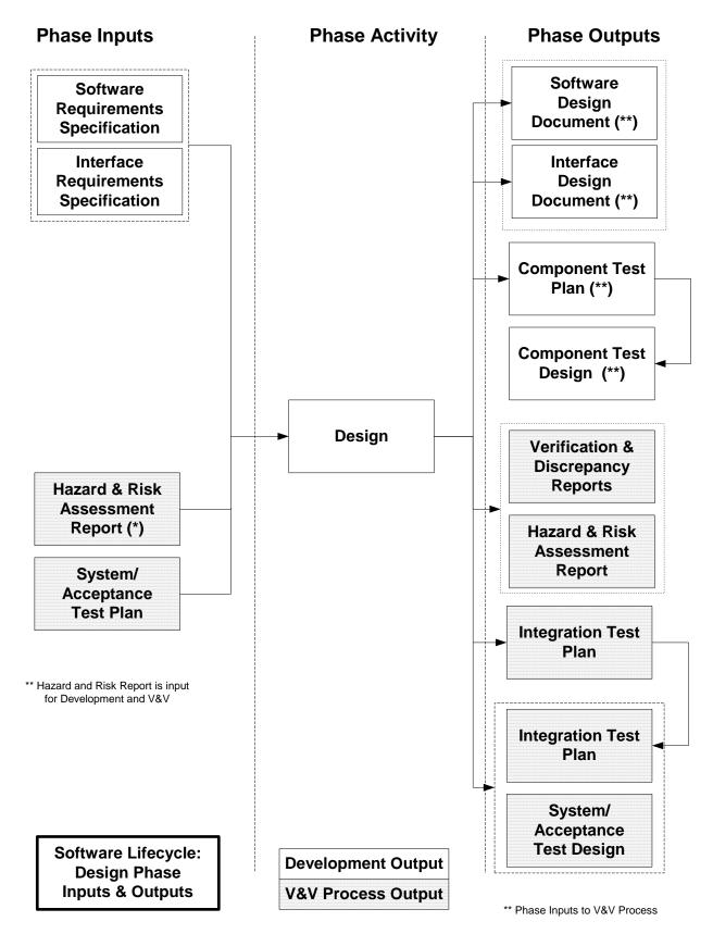
Figure 5-19 IEEE Std 1012 Design Phase Activity Inputs and Outputs
