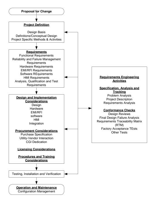
Figure 5-15 Digital Upgrade Life Cycle (Adapted from EPRI TR-102348)
