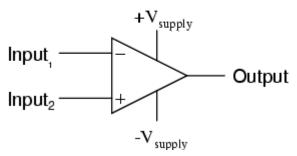
The two input leads can be seen on the left-hand side of the triangular amplifier symbol, the output lead on the right-hand side, and the +V and -V power supply leads on top and bottom. As with the other example, all voltages are referenced to the circuit's ground point.
