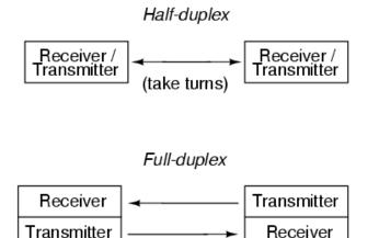
Half-duplex communication is analogous to two tin cans on the ends of a single taut string: Either can be used to transmit or receive, but not at the same time.
