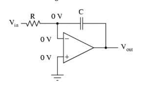
Negative feedback ensures that the inverting input will be held at 0 volts (the virtual ground). If the input voltage is exactly 0 volts, there will be no current through the resistor, therefore no charging of the capacitor, and therefore the output voltage will not change.
