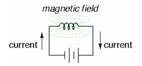
All other factors being equal, the greater the current, the greater will be the strength of the magnetic field. The magnetic field produced by a coil of currentcarrying wire can be used to exert a mechanical force on any magnetic object, just as we can use a permanent magnet to attract magnetic objects, except that this magnet (formed by the coil) can be turned on or off by switching the current on or off through the coil.
