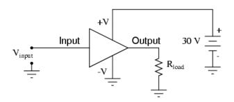
Without having to analyze the actual internal design of the amplifier, the above circuit illustrates that its function is to take an input signal ( $V_{in}$ ), amplify it, and drive a load resistance ( $R_{load}$ ).
