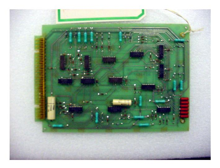
Figure 2-10 Westinghouse SSPS Universal Logic Circuit Card
