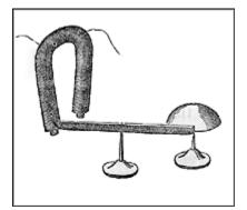
A relay is an electromagnetically operated switch. An electric current through a conductor will produce a magnetic field at right angles to the direction of electron flow. If that conductor is wrapped into a coil shape, the magnetic field produced will be oriented along the length of the coil, as shown below:
