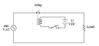
One relay coil/armature assembly may be used to actuate more than one set of contacts. Those contacts may be normally-open, normally-closed, or any combination of the two. As with switches, the "normal" state of a relay's contacts is when the coil is deenergized; that is, when the relay is sitting on a shelf in its box, not connected to any circuit.
