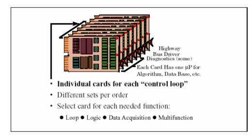
Figure 2-23 Individual Loop Controller
