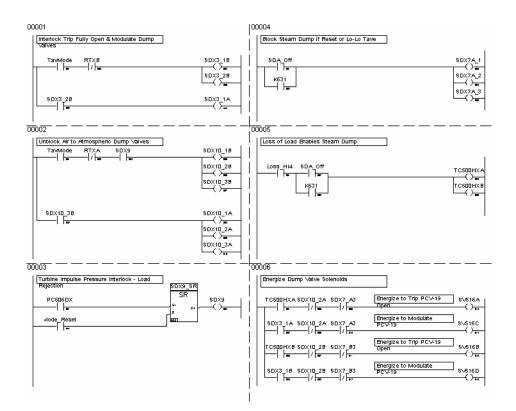
Figure 2-43 Relay Logic Transformation to Ladder Logic Program
