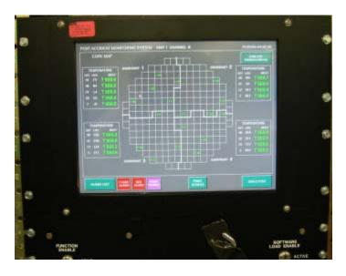
Figure 2-55 Westinghouse Common Q Qualified Flat Panel Display
