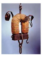
Henry also used an electromagnet to create a remote signaling device (. The device used an electromagnet and a bell, and preceded Samuel F. B. Morse's telegraph. Lawsuits filed at the time indicated that Morse used Henry's ideas but patented them, making them his own.
