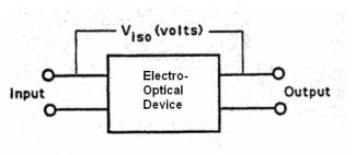
A typical Viso specification is about 1500 Vdc for 60 seconds and 1500 Vac, 47 to 70 Hz, for 60 seconds.
