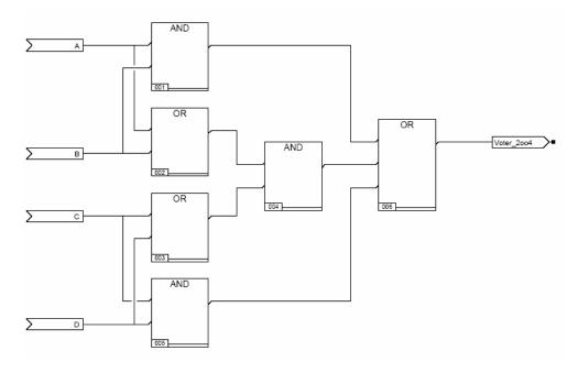
Figure 2-36 Typical Custom Function Block (2004) Coincidence Logic
