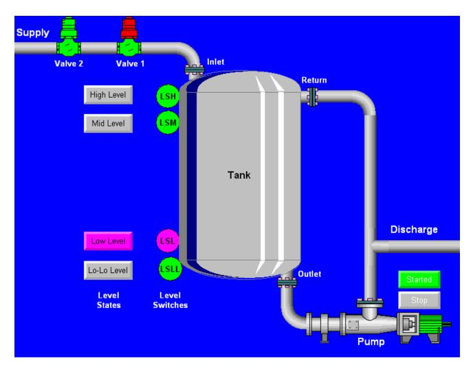
Figure 2-51 Object-Oriented HMI Display
