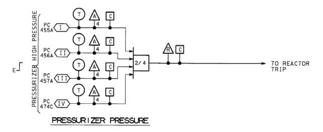
Figure 2-45 Pressurizer Pressure Protection Functional Diagram
