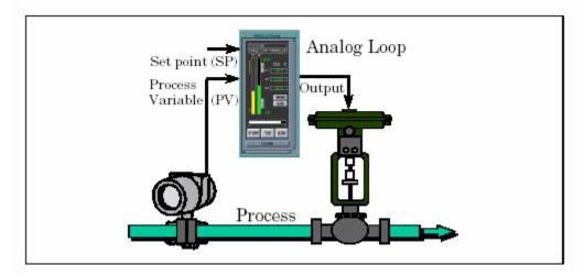
Figure 2-20 Typical Analog Process Loop
