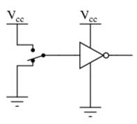
A common way to express the particular function of a gate circuit is called a truth table. Truth tables show all combinations of input conditions in terms of logic level states (either "high" or "low," "1" or "0," for each input terminal of the gate), along with the corresponding output logic level, either "high" or "low." For the inverter, or NOT, circuit just illustrated, the truth table is very simple:
