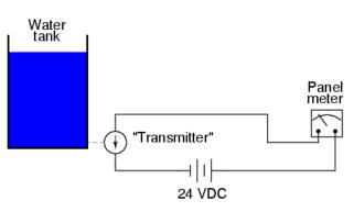
The transmitter outputs 4 mA at zero level and 20 mA at 100% level. The simplest solution is to send the analog signal to the remote location on a pair of copper wires. In most cases, this is a good solution. However, this lesson is about digital communications, so we will explore methods of transmitting the information digitally.
