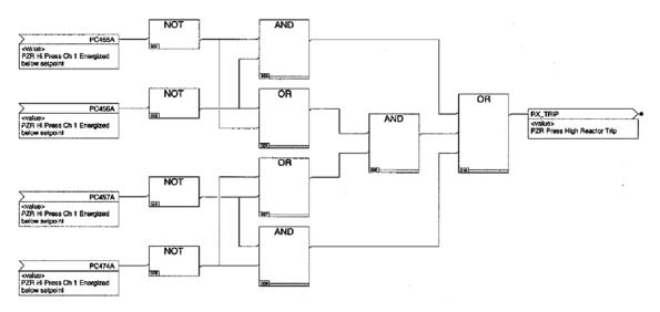
Figure 2-47 Pressurizer Pressure Protection Function Block Diagram Program
