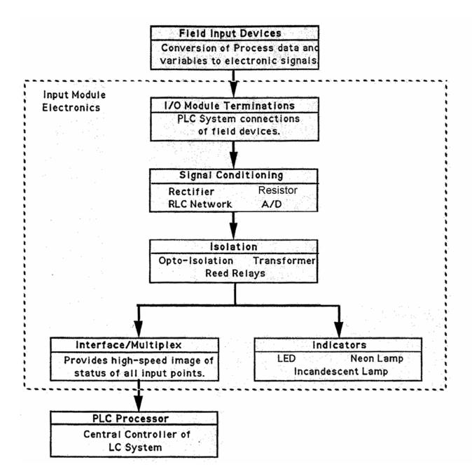
Figure 2-26 PLC Input Structure
