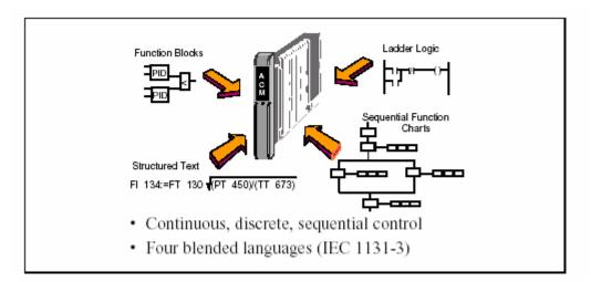
Figure 2-24 Single Control Module
