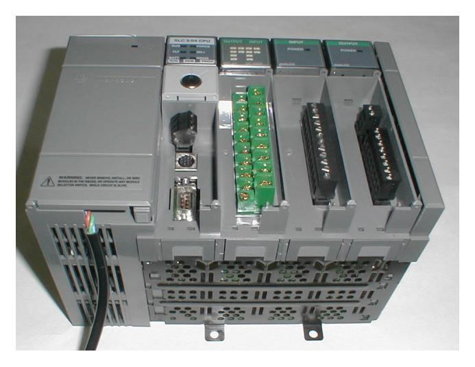
Figure 2-19 Typical Industrial Programmable Controller
