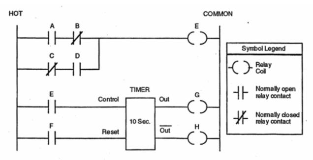
Figure 2-18 Simple Ladder Logic Program
