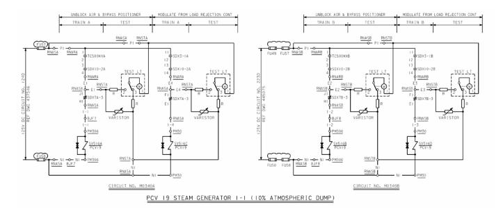
Figure 2-42 Steam Dump Valve Control Schematic Diagram
