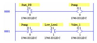
The requirement: "When the PB is released, the pump keeps running" means that we need to "latch" or "seal" the pump. The Stop\_PB is needed to manually shut off the pump. The Low\_Level switch stops the pump on low level:
