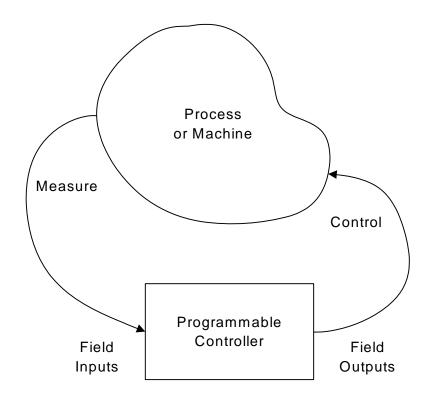
Figure 2-16 Industrial Computer (PLC) Concept
