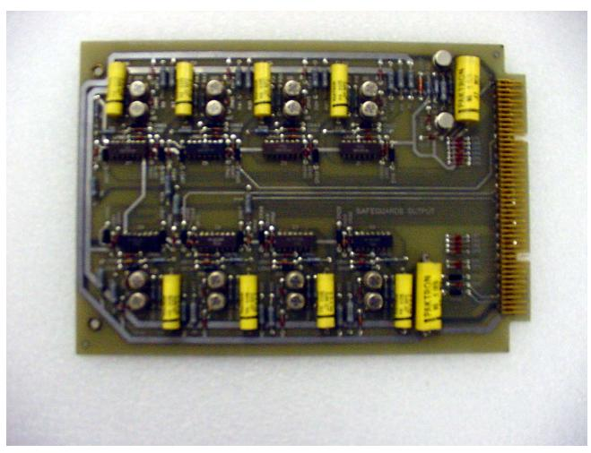
Figure 2-14 Westinghouse SSPS SAF Driver Circuit Card
