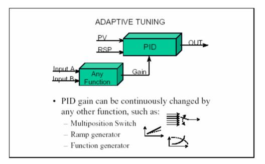
Figure 2-37 Multifunction Control Algorithms
