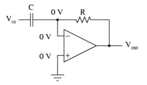
The right-hand side of the capacitor is held to a voltage of 0 volts, due to the "virtual ground" effect. Therefore, current "through" the capacitor is solely due to change in the input voltage. A steady input voltage won't cause a current through C, but a changing input voltage will.
