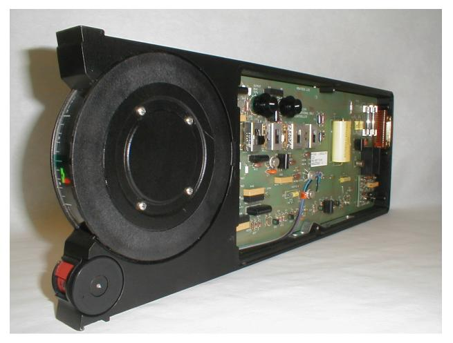
Figure 2-2 Analog Controller – Discrete Component Technology
