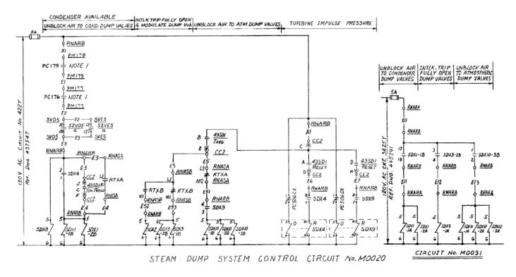
Figure 2-40 Steam Dump Control Schematic Diagram
