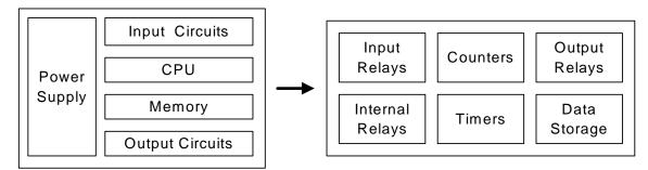
Figure 2-25 Inside the PLC
