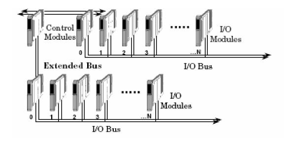
Figure 2-32 Remote I/O Using Peer-to-Peer Communications
