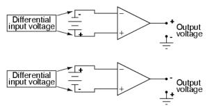
When the polarity of the *differential* voltage matches the markings for inverting and noninverting inputs, the output will be positive. When the polarity of the differential voltage clashes with the input markings, the output will be negative.
