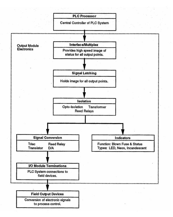
Figure 2-27 PLC Output Structure
