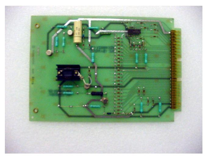
Figure 2-12 Westinghouse SSPS UV Driver Circuit Card
