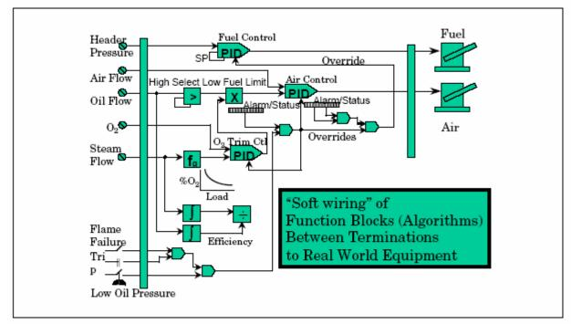
Figure 2-38 Configuration - Connecting the Blocks with "Soft Wiring"
