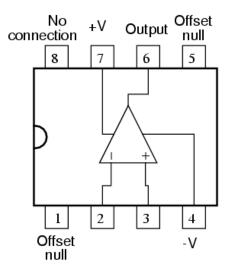
The term "DIP" means "Dual In-line Package" to distinguish it from other package types.
