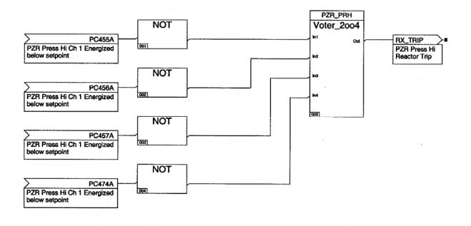
Figure 2-48 Pressurizer Pressure Protection Function Block Diagram Program – Custom Block
