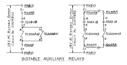
Figure 2-41 Auxiliary Relays Schematic Diagram
