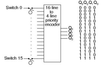
Only four (4) wires, plus any ground and power wires, are required to transmit the same information. This illustrates the concept of *multiplexing*.
