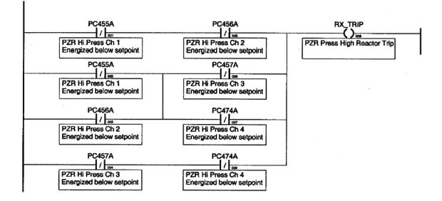
Figure 2-46 Pressurizer Pressure Protection Ladder Logic Program
