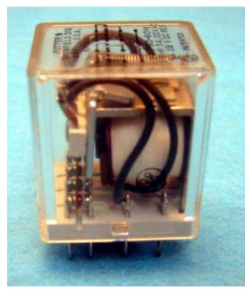
Figure 2-3 Typical Industrial Control Relay
