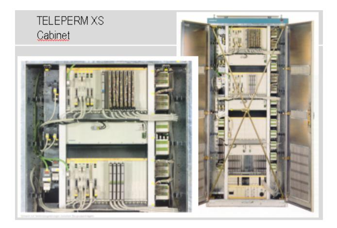
Figure 2-53 Siemens Teleperm XS PLC (with SER)
