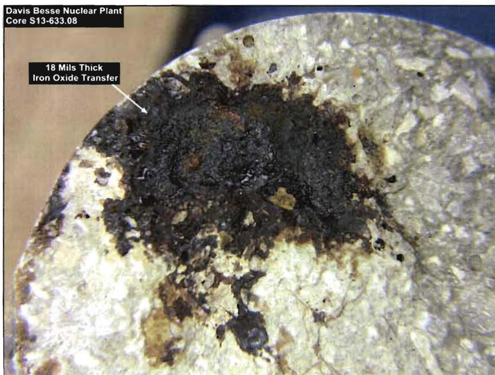
Figure A 9: Iron Oxide Transfer to Concrete (Core S13-633.08)
