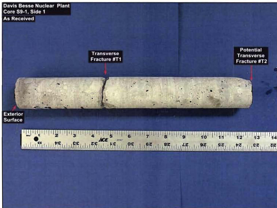
Figure A 2: Example of As Received Core Sample with Transverse Crack (Sample # S9-1)
