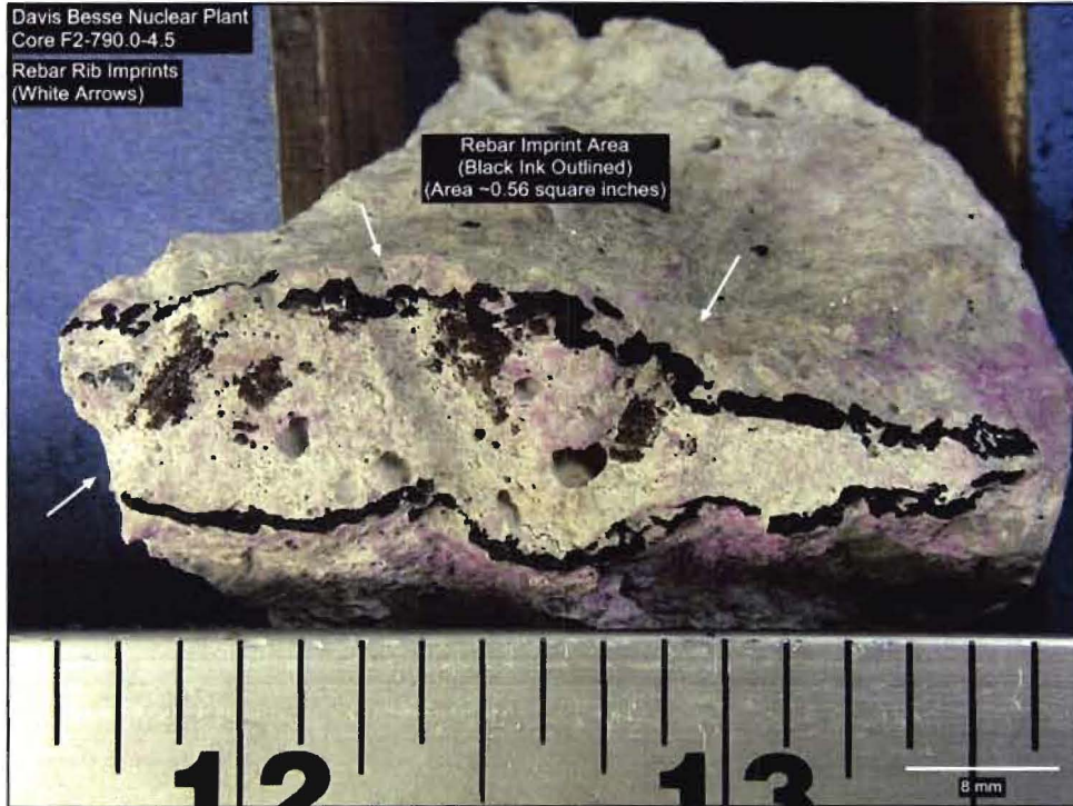
Figure A 4: Rebar Rib Groove Imprints (Core F2-790.0-4.5)
