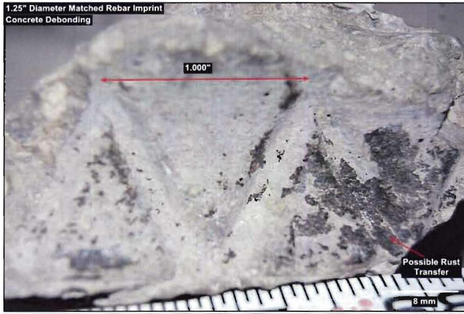
Figure A 1: Shield Building Concrete Sample Illustrating Rebar Imprint
