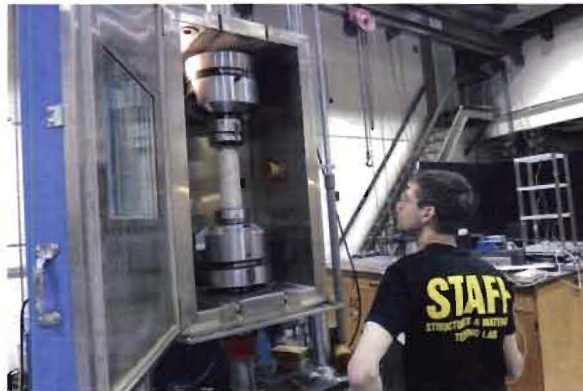
Fig. 6 The MTS machine provides a stable compressive force at 16 kips
