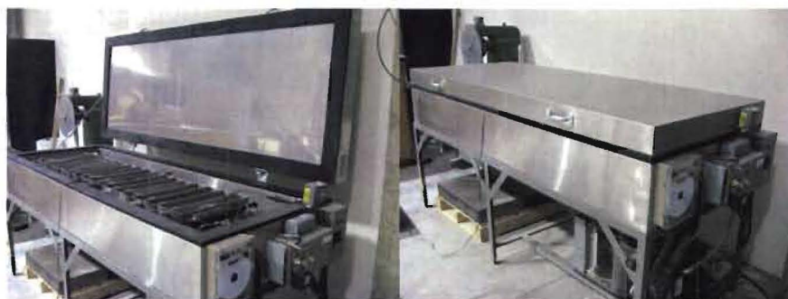
Fig. 12. The rapid freeze-thaw test chest
