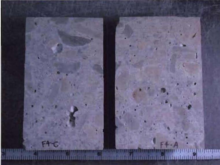
Figure 5. Lapped cross-sections of Core F4 that were analyzed by point-count analysis. The bottom approximate half of the concrete shows significant amounts of entrapped voids, including one larger unconsolidated void in the specimen on the left, while the upper halves show less air voids.
