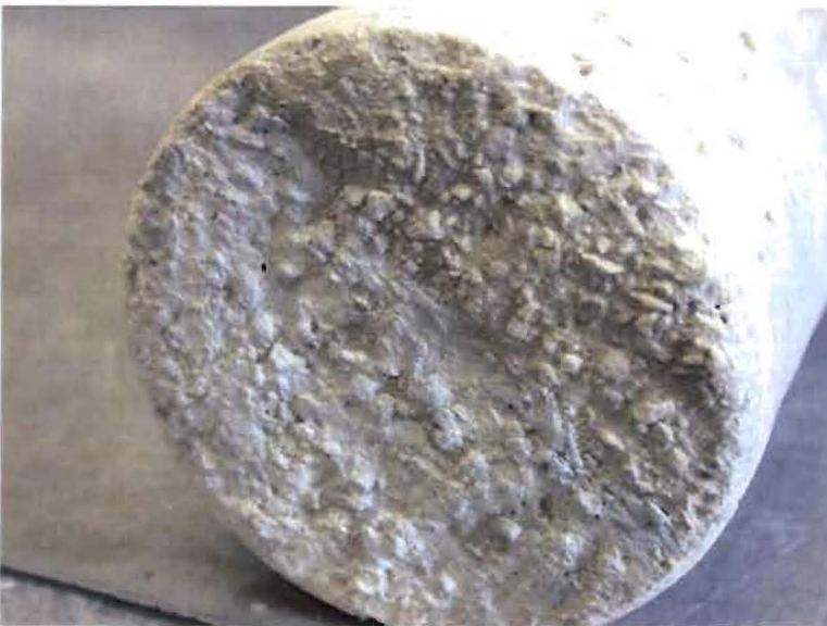
Figure 2. Exposed end of Core F2, showing sand particles elevated slightly in relief above the coating. The gray and tan portions of the surface are readily apparent.
