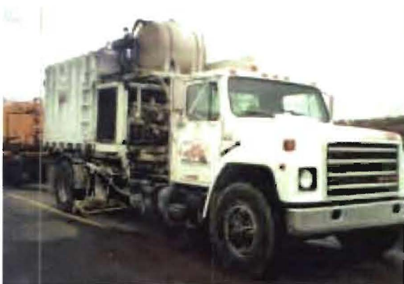
Figure 3: Heavy, self contained vacuum truck . Note: vacuum nozzle located in front of the rear wheel works very well to pick up debris.
