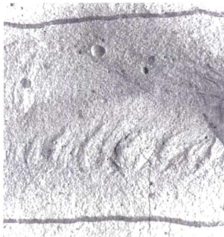
Figure 2.15 Fracture surface of a cement sample cut with a high-speed water jet (Momber and Kovacevic, 1994)
