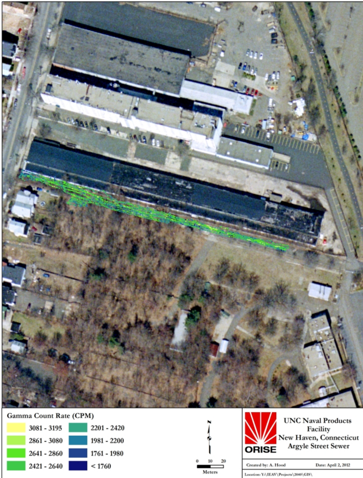
Fig. 3. Argyle Street Sewer - Gamma Walkover Scan
