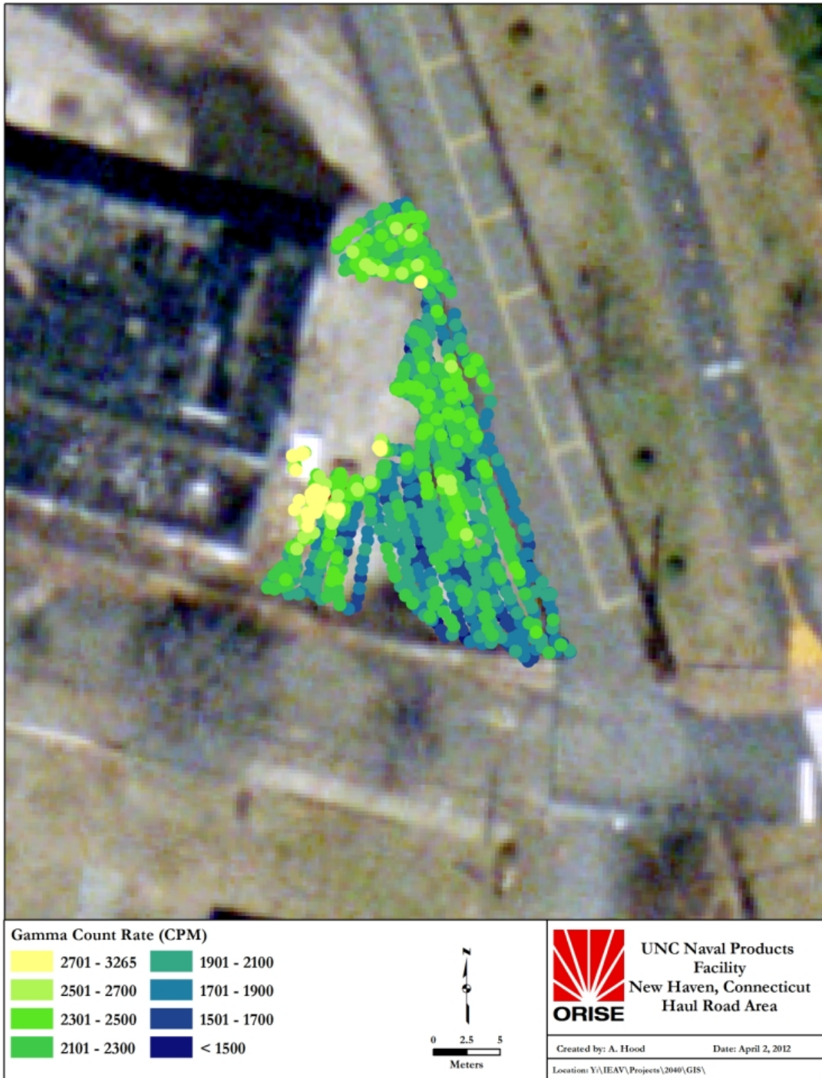
Fig. 5. Haul Road Area- Gamma Walkover Scan
