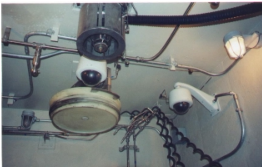
FIGURE 9 SOLID PRODUCT PACKAGING STATION – FILLPORT AND CONTAINER CAPPER
