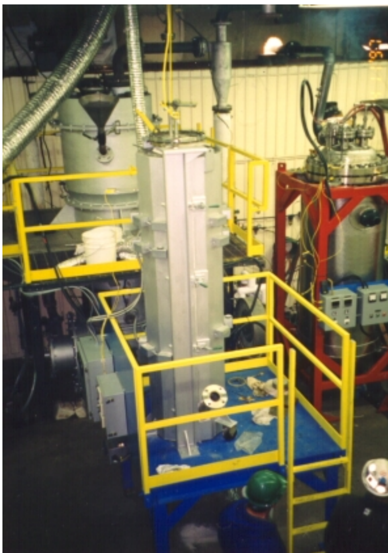
FIGURE 10 PILOT-SCALE FLUID BED REFORMER DEMONSTRATION SYSTEM ASSEMBLY
