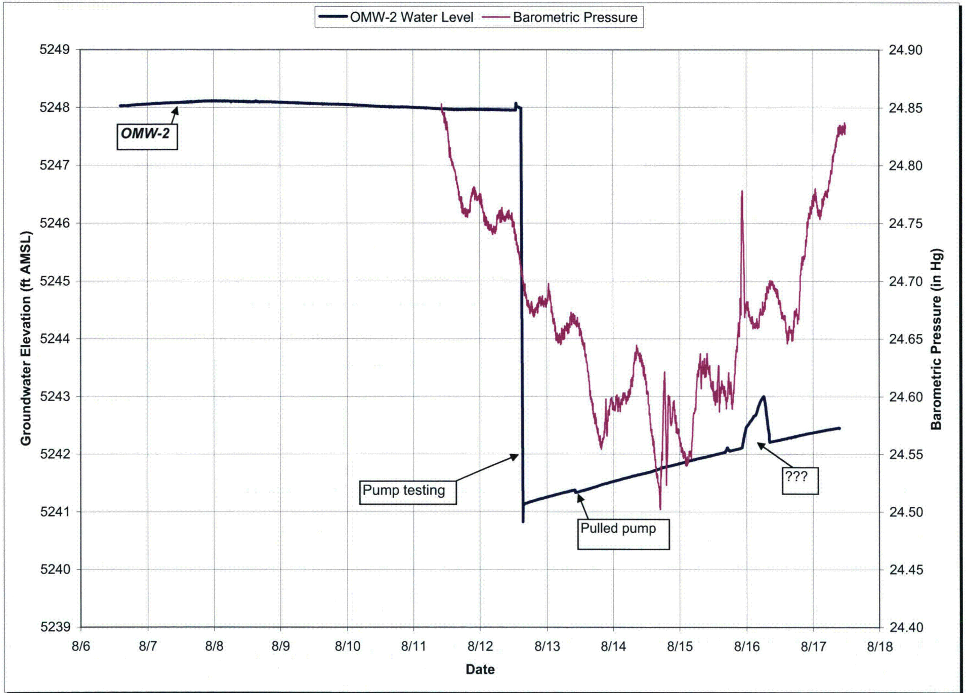
Figure 6-4. OMW-2 Water Level vs Barometric Pressure, 72 Sand
