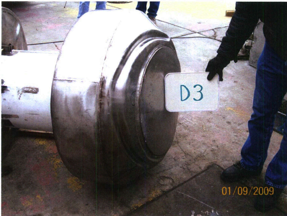
Figure 2.12.3-26 - Free Drop Test D3 Deformation
