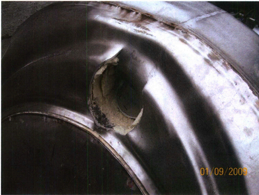
Figure 2.12.3-29 - Puncture Test P4 Damage
