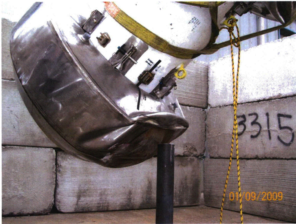
Figure 2.12.3-30 - Puncture Test P5 Orientation
