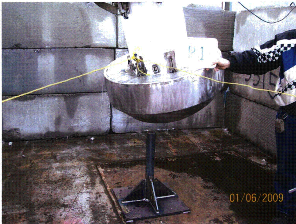
Figure 2.12.3-10 - Puncture Test P1 Orientation
