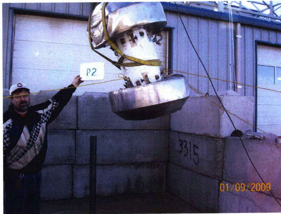
Figure 2.12.3-23 - Puncture Test P2 Orientation
