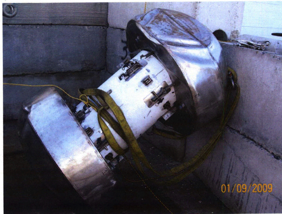
Figure 2.12.3-24 - Puncture Test P2 Result
