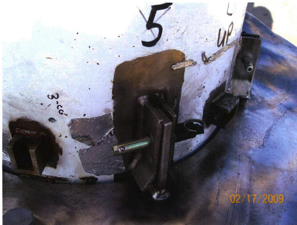
Figure 2.12.3-37 - Attachment Location #5 After Free Drop D2C
