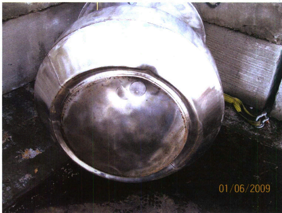
Figure 2.12.3-11 - Puncture Test P1 Deformation
