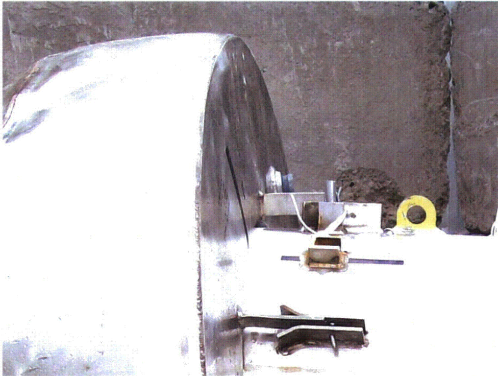
Figure 2.12.3-16 - Free Drop Test D2, Close-up View of Failed Attachments
