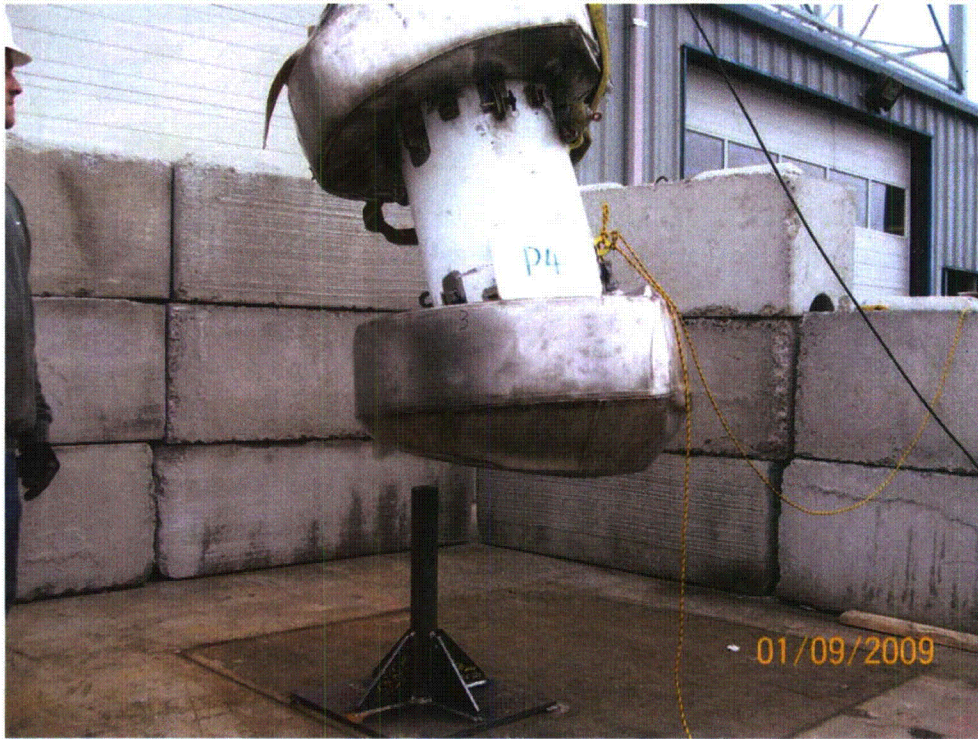
Figure 2.12.3-28 - Puncture Test P4 Orientation
