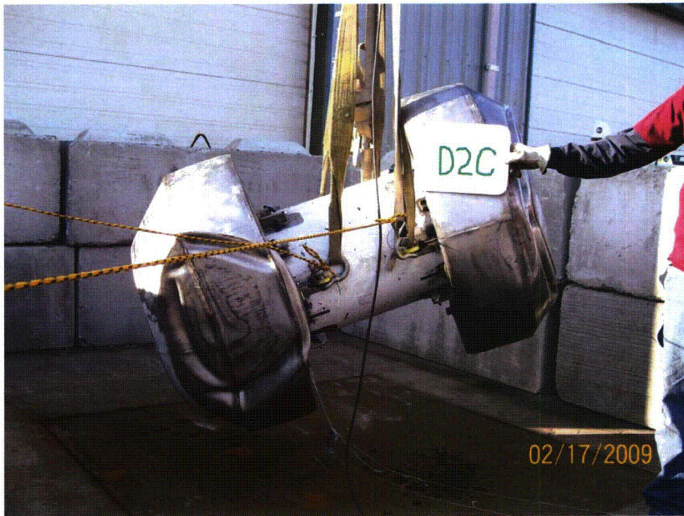
Figure 2.12.3-36 - Free Drop Test D2C Orientation
