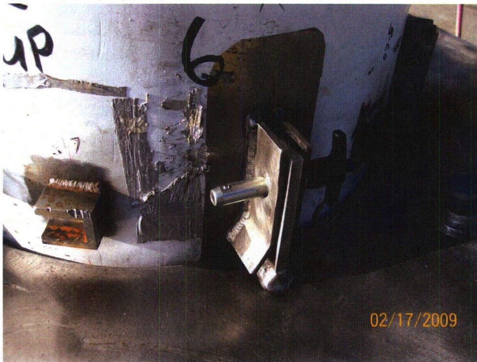
Figure 2.12.3-38 - Attachment Location #6 After Free Drop D2C
