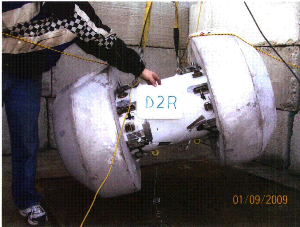
Figure 2.12.3-18 - Free Drop Test D2R Orientation
