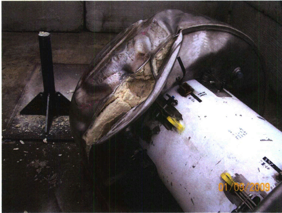
Figure 2.12.3-32 - Puncture Test P5 Damage
