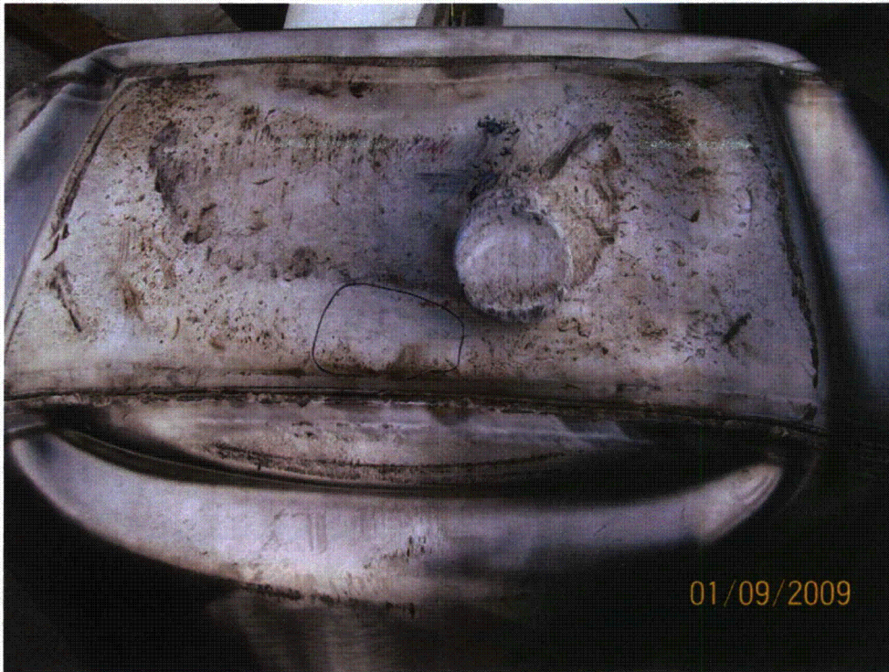
Figure 2.12.3-34 - Puncture Test P3 Damage
