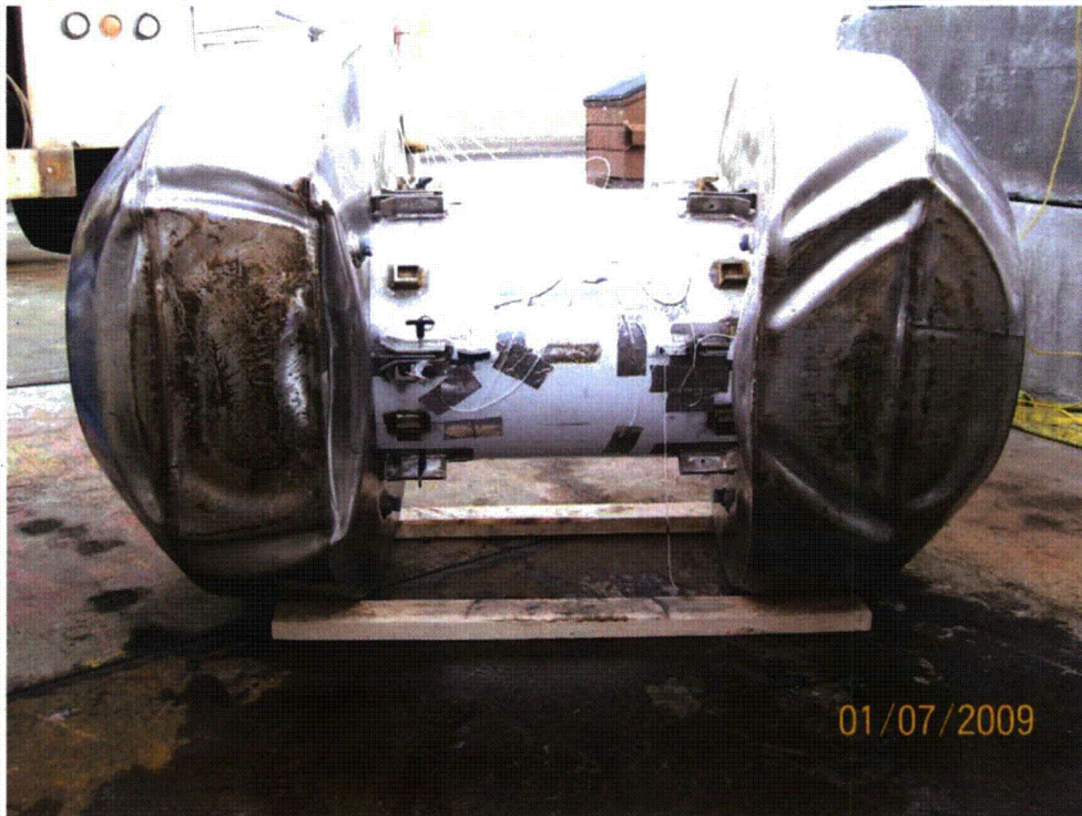
Figure 2.12.3-17 - Free Drop Test D2 Impact Deformation Surfaces
