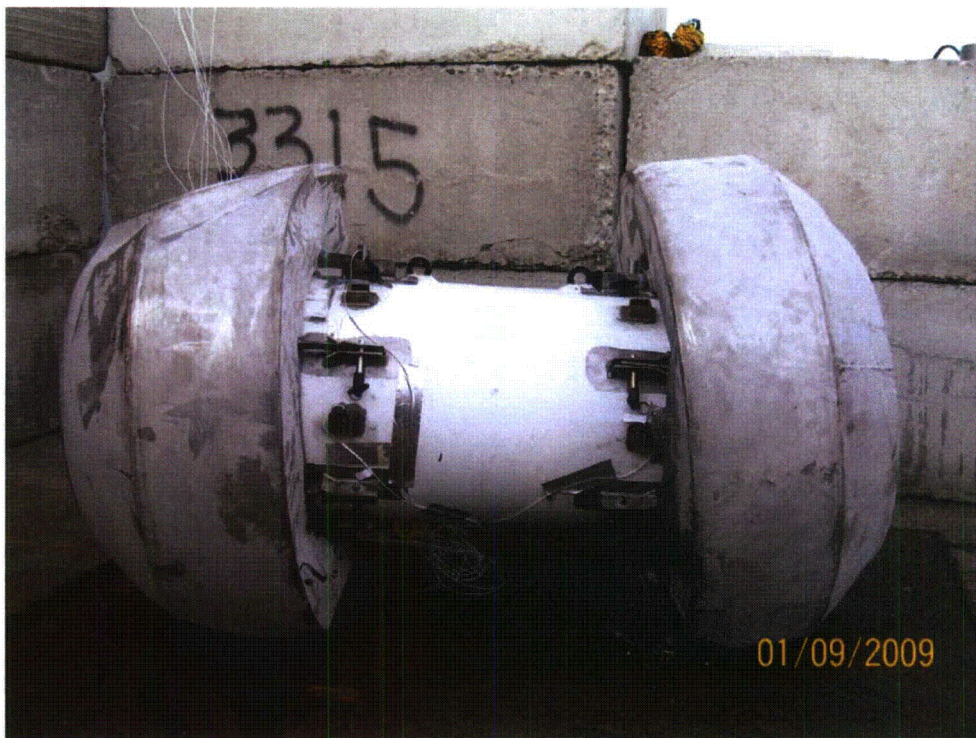
Figure 2.12.3-19 - Free Drop Test D2R Post-test Configuration
