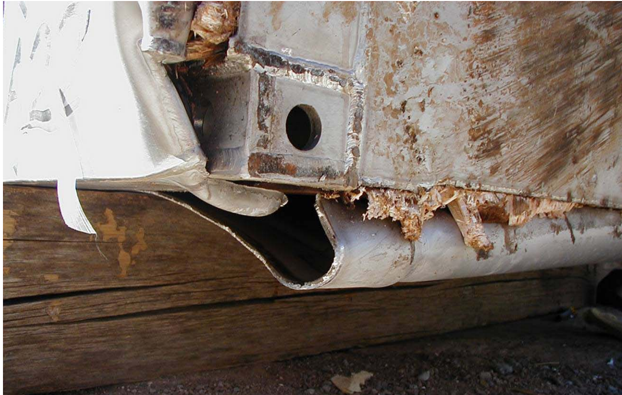
Figure 2.12.1-35 – Free Drop Test FD1: Close-up View of ISO Fitting Damage
