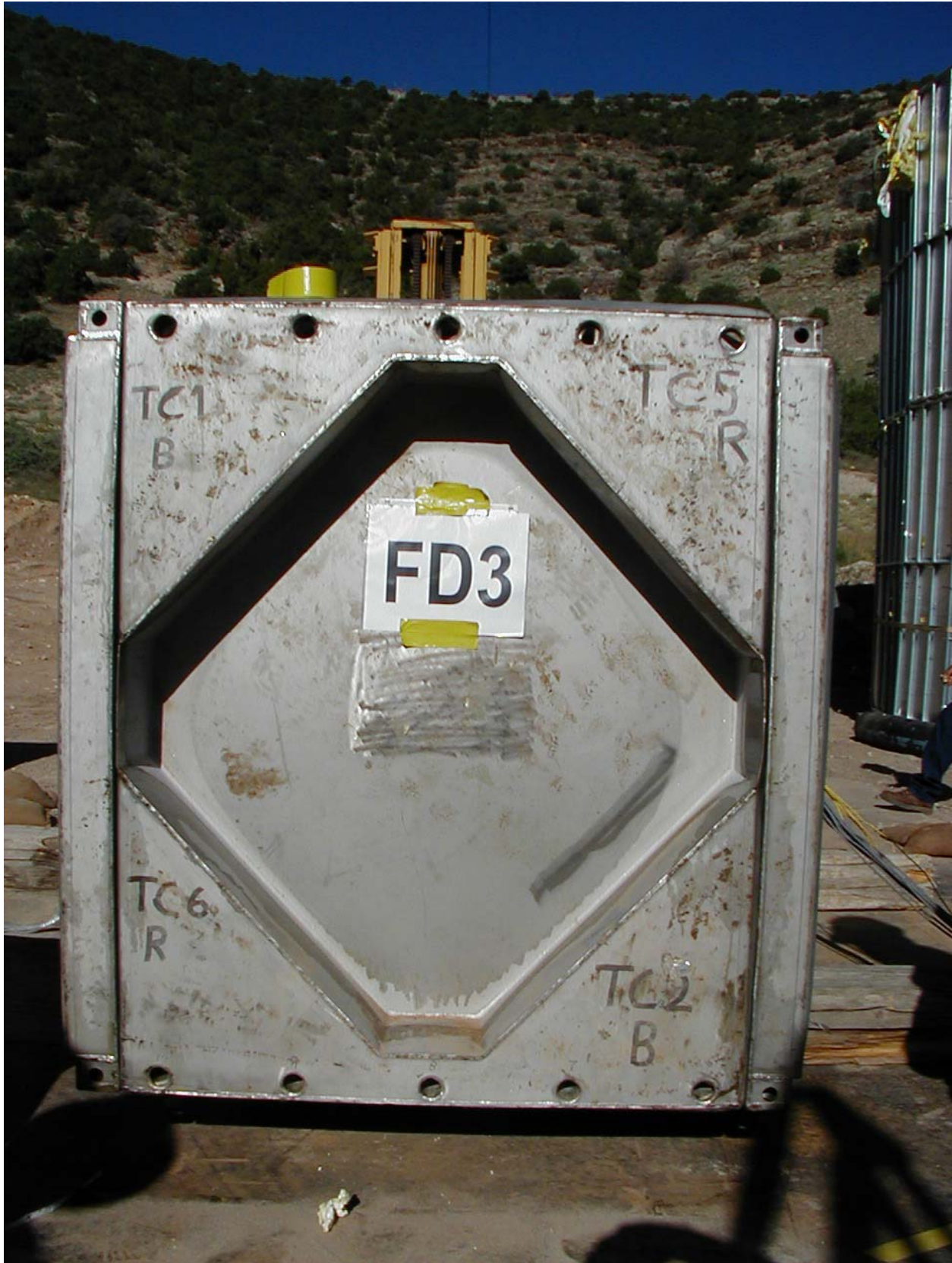
Figure 2.12.1-37 – Free Drop Test FD3: Overall View of Overpack Cover Damage
