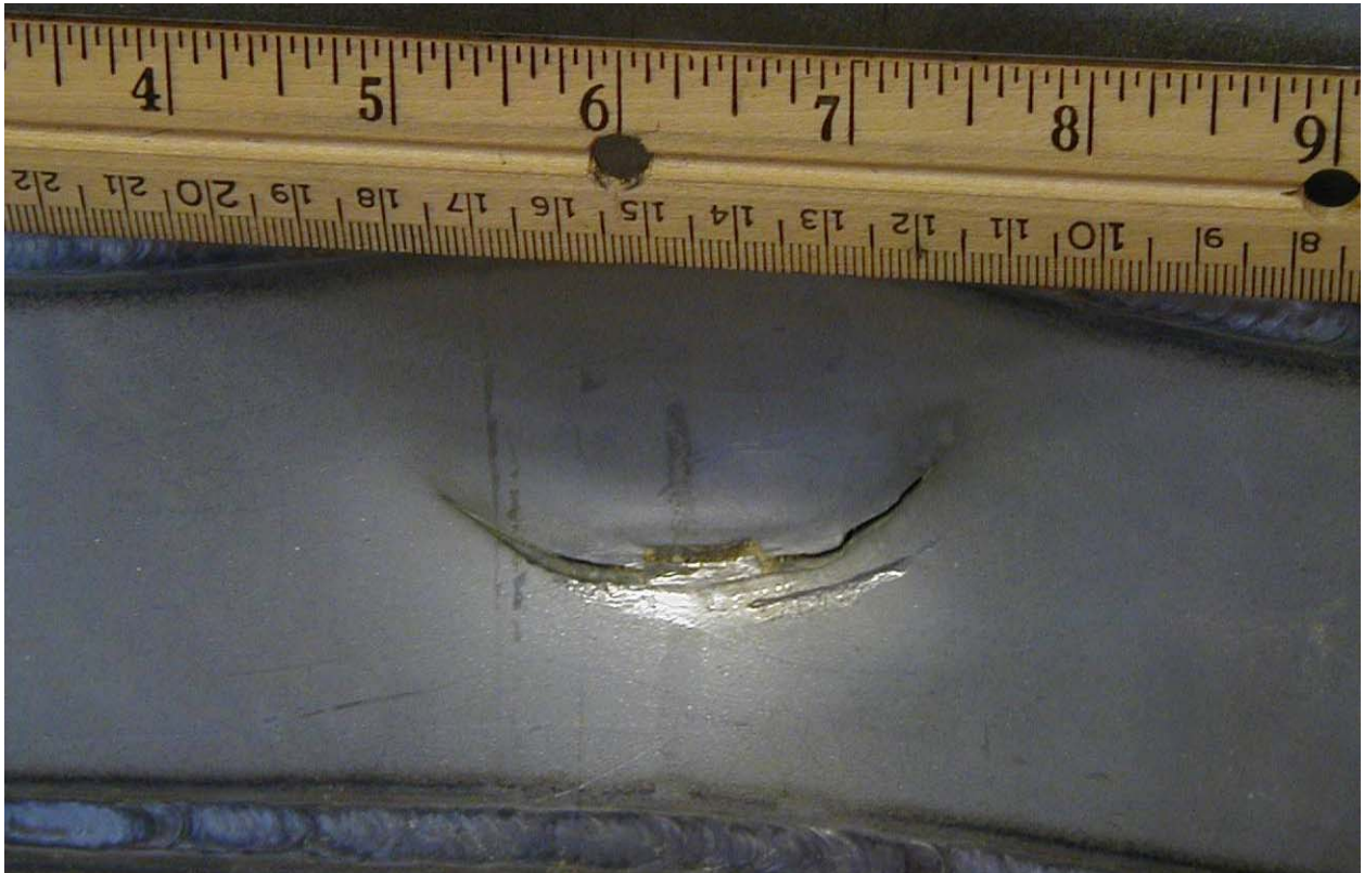
Figure 2.12.1-52 – Puncture Drop Test P4: Close-up of CSA Structural Sheet Damage
