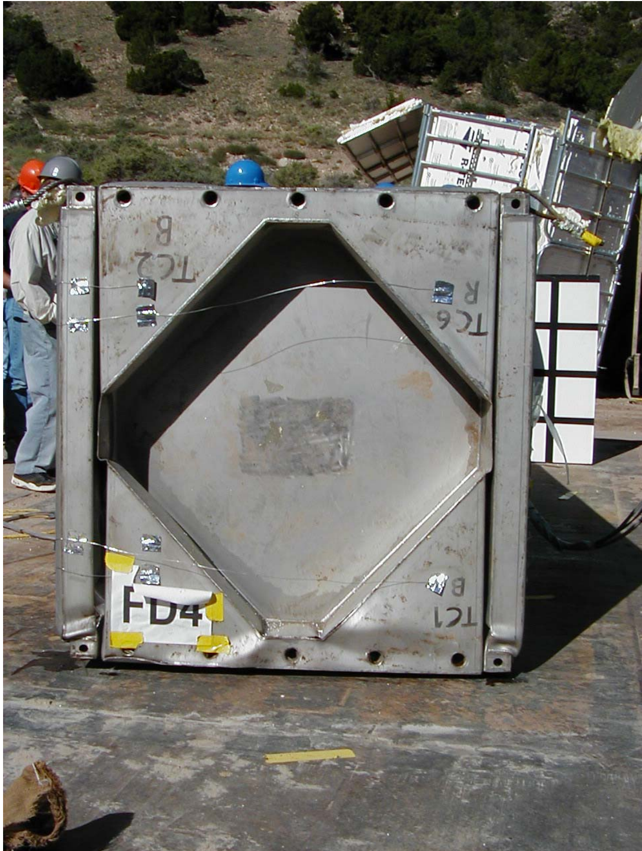
Figure 2.12.1-41 – Free Drop Test FD4: Overall View of Secondary Impact Damage
