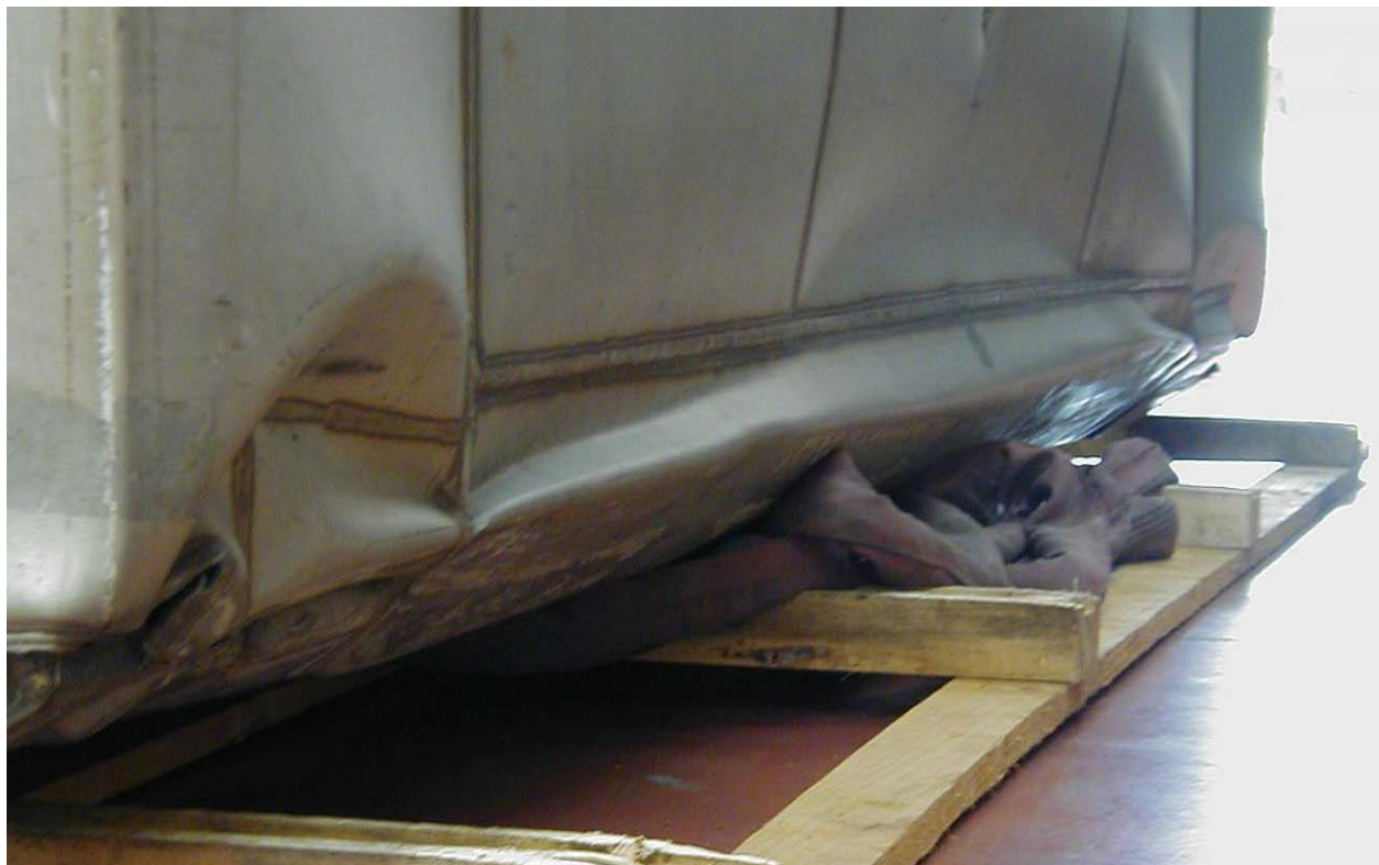
Figure 2.12.1-30 – Free Drop Test A6: Overall View of Long-Edge Damage
