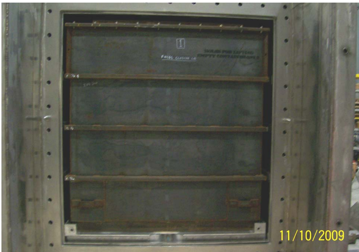
Figure 2.12.6-8 – SLB2 and Pallet Installed in the Payload Cavity
