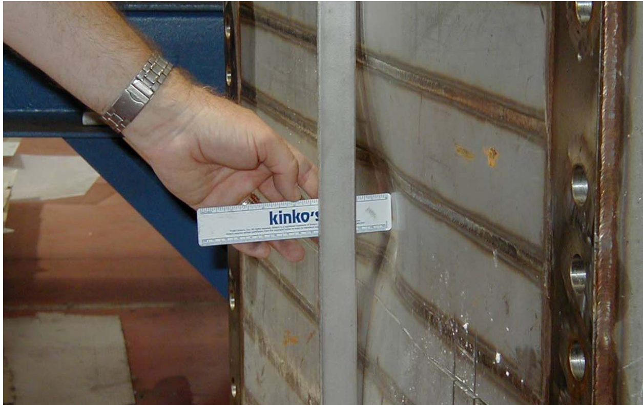
Figure 2.12.1-33 – Post-Test Disassembly: Close-up View of Closure Lid Puncture Damage
