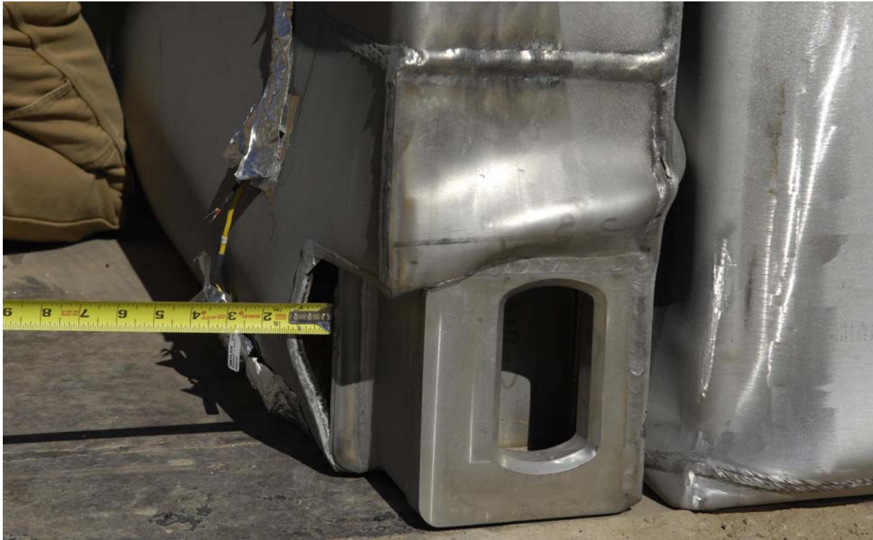
Figure 2.12.3-12 – Test LD2, Close-up of Deformation and Torn Welds Around ISO Fitting
