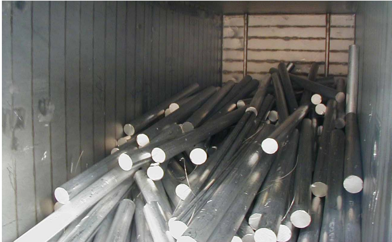
Figure 2.12.1-53 – Post-Test Disassembly: View of Loose Simulated Payload in Cavity
