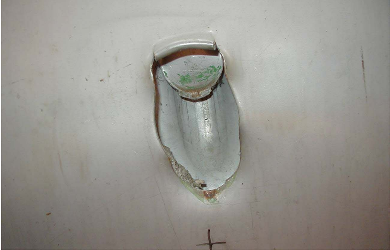
Figure 2.12.1-27 – Puncture Drop Test F9: Close-up View of Damage
