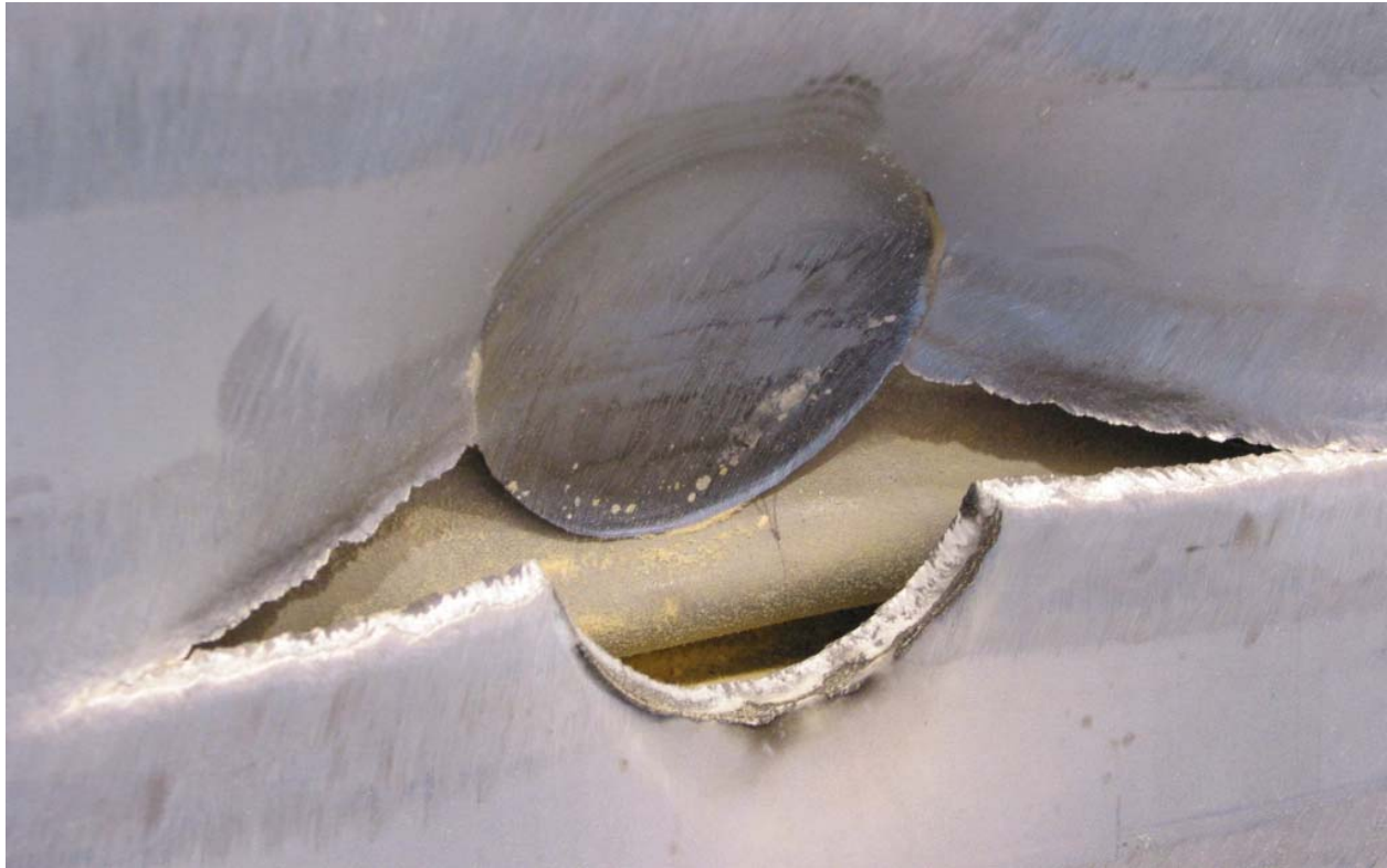
Figure 2.12.1-45 – Puncture Drop Test P1: Close-up View of Closure Lid Damage
