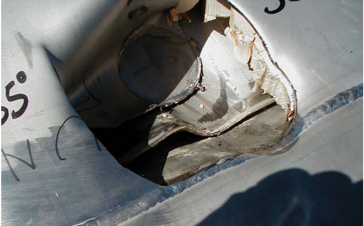
Figure 2.12.1-57 – Puncture Drop Test P105 at 35°
