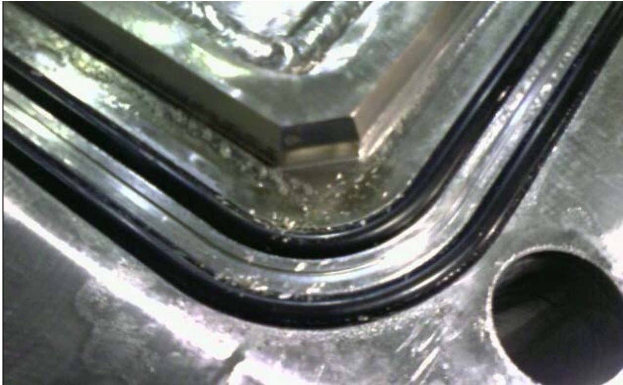
Figure 2.12.3-34 – Debris on Closure Lid Seals (Lower Left Corner of Lid)
