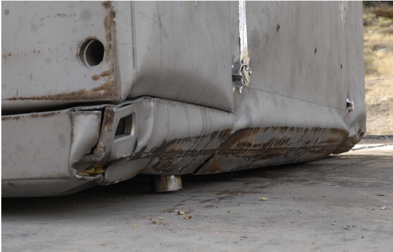
Figure 2.12.3-16 – Test LD5, Typical Deformation
