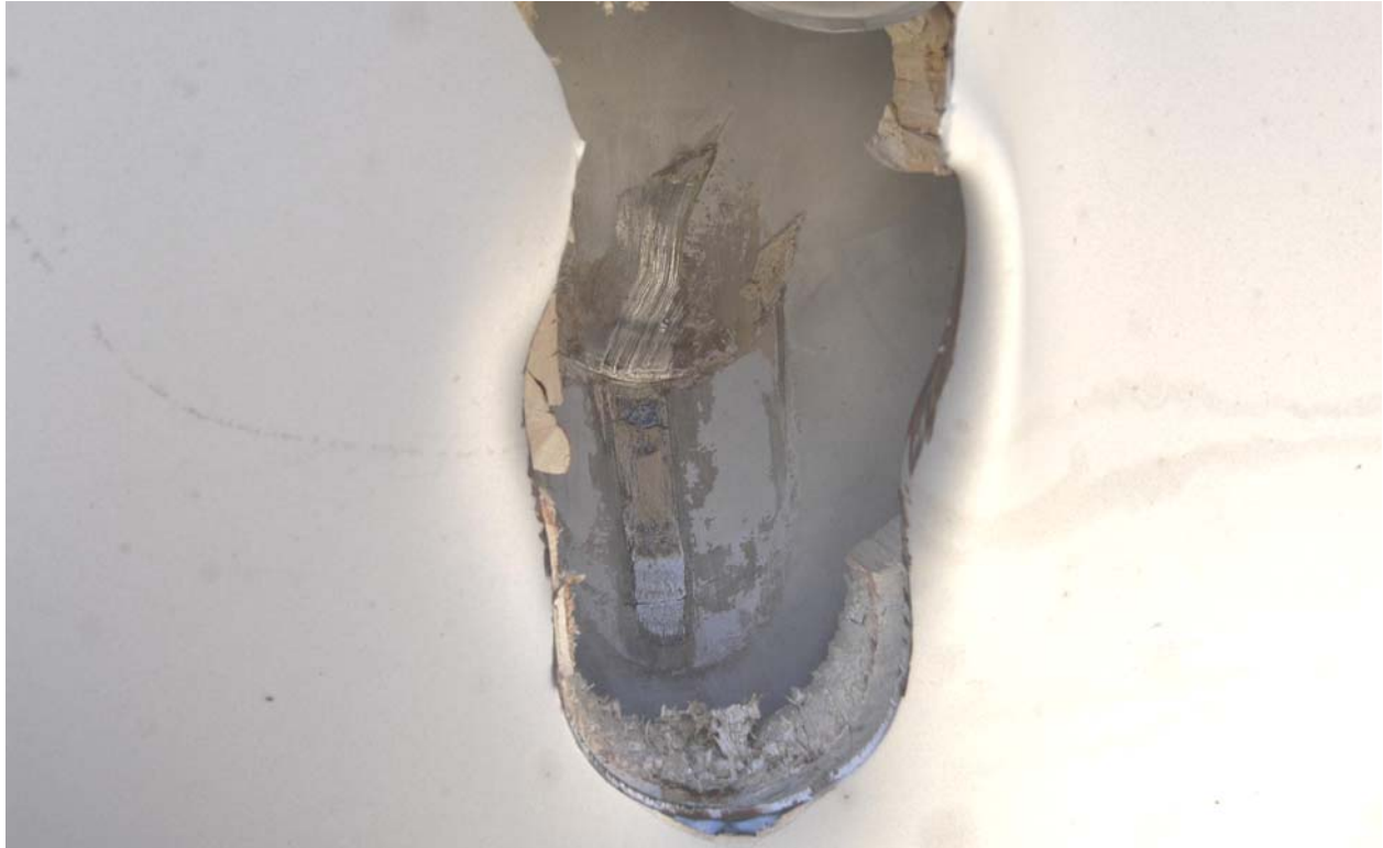
Figure 2.12.3-28 – Test LP2, Close-up of Damage. Bottom of Hole is Puncture-Resistant Plate
