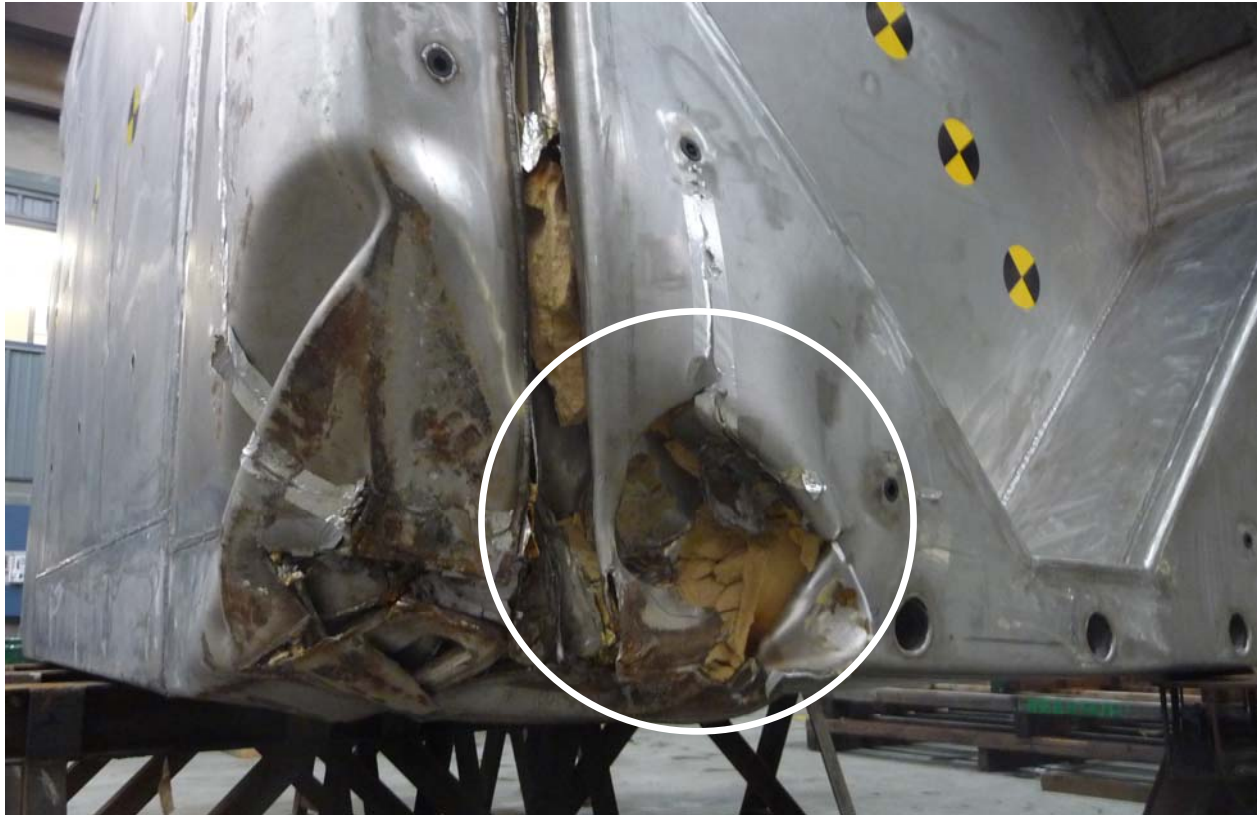
Figure 2.12.6-13 – Test LP91, CG-Over-Corner Puncture Damage
