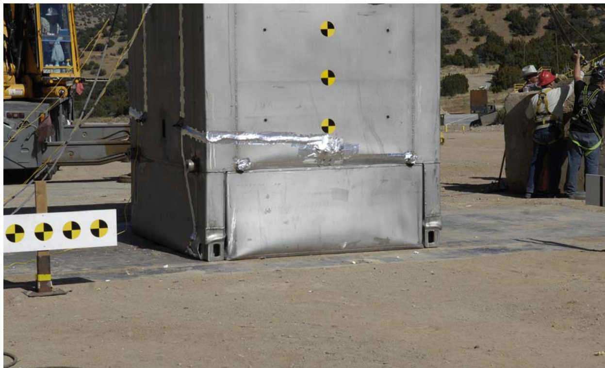
Figure 2.12.3-10 – Test LD2, Typical Deformations at Closure End
