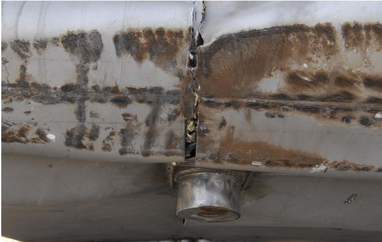
Figure 2.12.3-18 – Test LD5, Weld Tear Between Cheek (left half) and Body Edge (right half)
