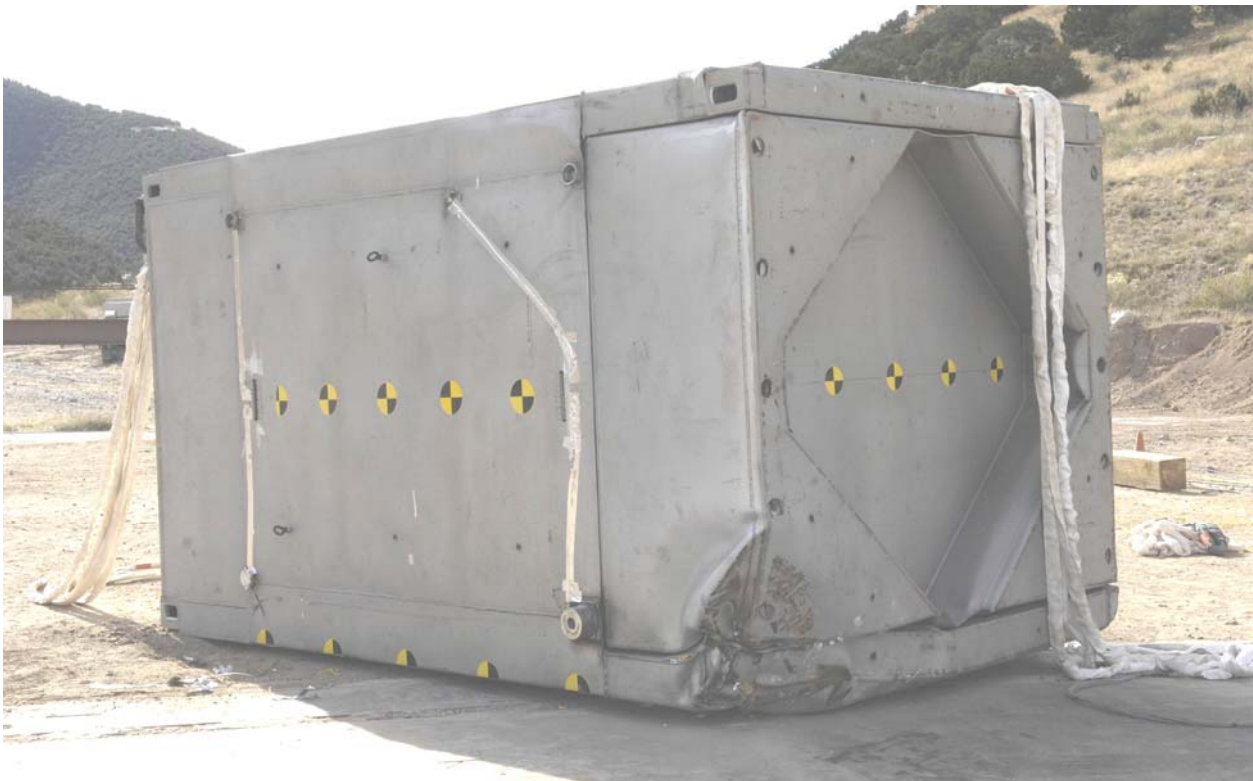
Figure 2.12.3-19 – Test LD4, Typical Deformations
