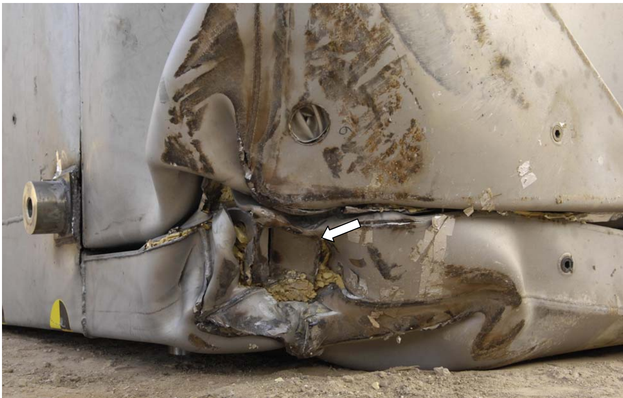
Figure 2.12.3-21 – Test LP3. Puncture Bar Damage Indicated by Arrow
