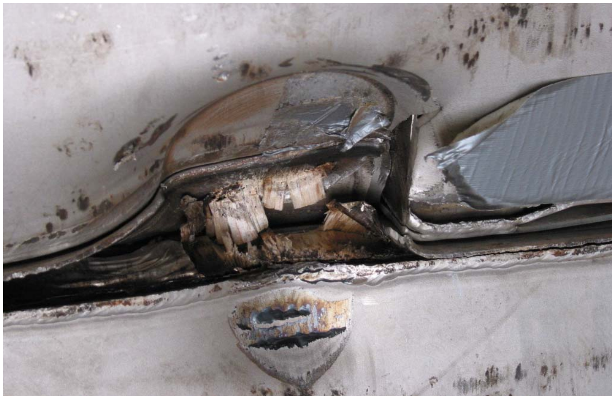
Figure 2.12.1-49 – Puncture Drop Test P3: Close-up of Damage to Overpack Cover-Body Joint
