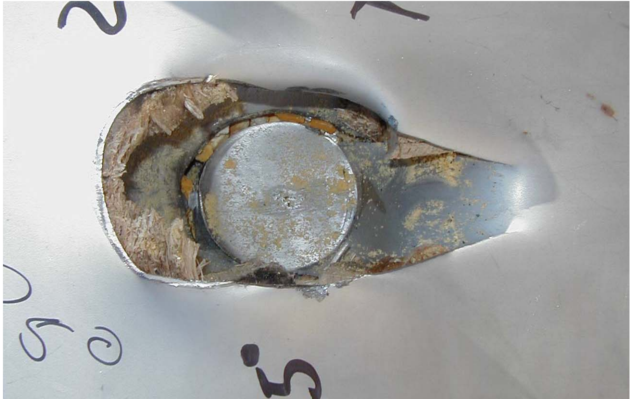
Figure 2.12.1-59 – Puncture Drop Test P305 at 25°
