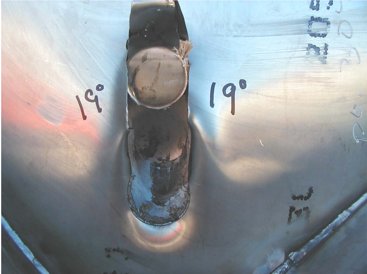
Figure 2.12.1-61 – Puncture Drop Test P505 at 19° (ETU longitudinal axis 71°)
