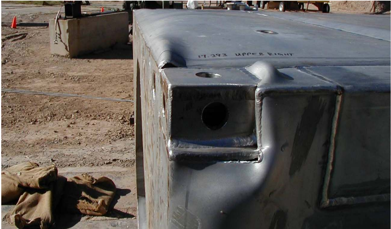
Figure 2.12.1-38 – Free Drop Test FD3: Close-up View of ISO Fitting Damage
