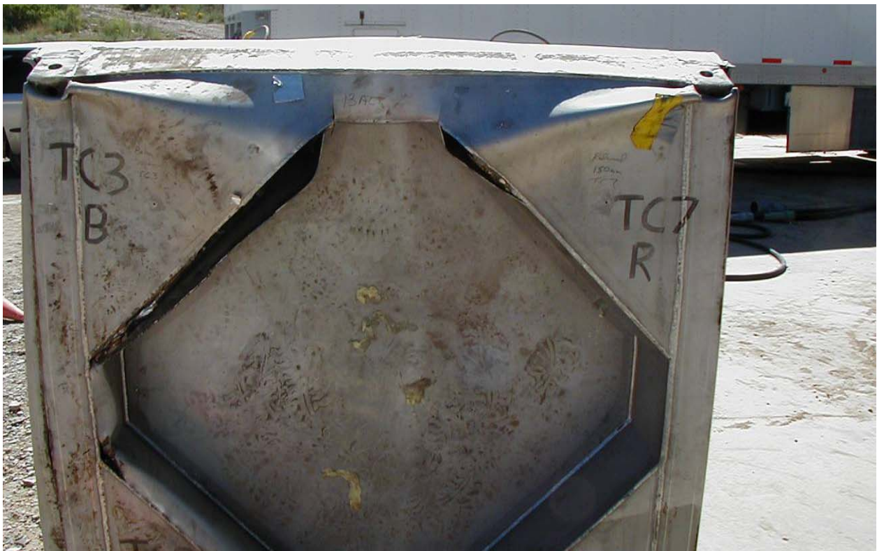
Figure 2.12.1-39 – Free Drop Test FD4: Overall View of Primary Impact Damage
