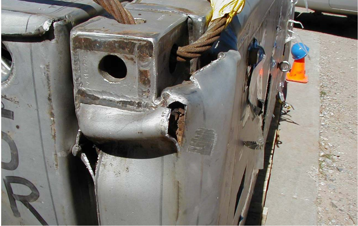
Figure 2.12.1-42 – Free Drop Test 4: View of ISO Fitting Damage, Secondary Impact
