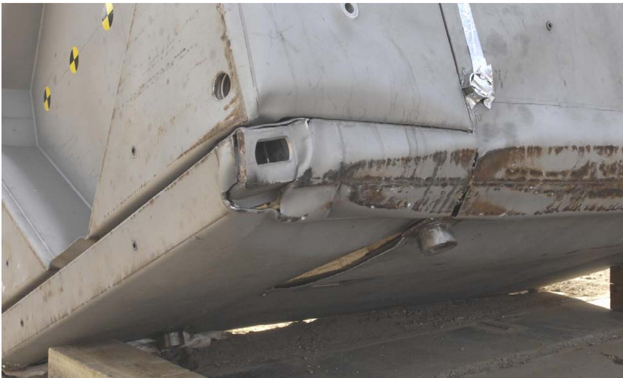
Figure 2.12.3-17 – Test LD5, Weld Tear Along Forward Edge of Side Outer Sheet (2-inch gap)
