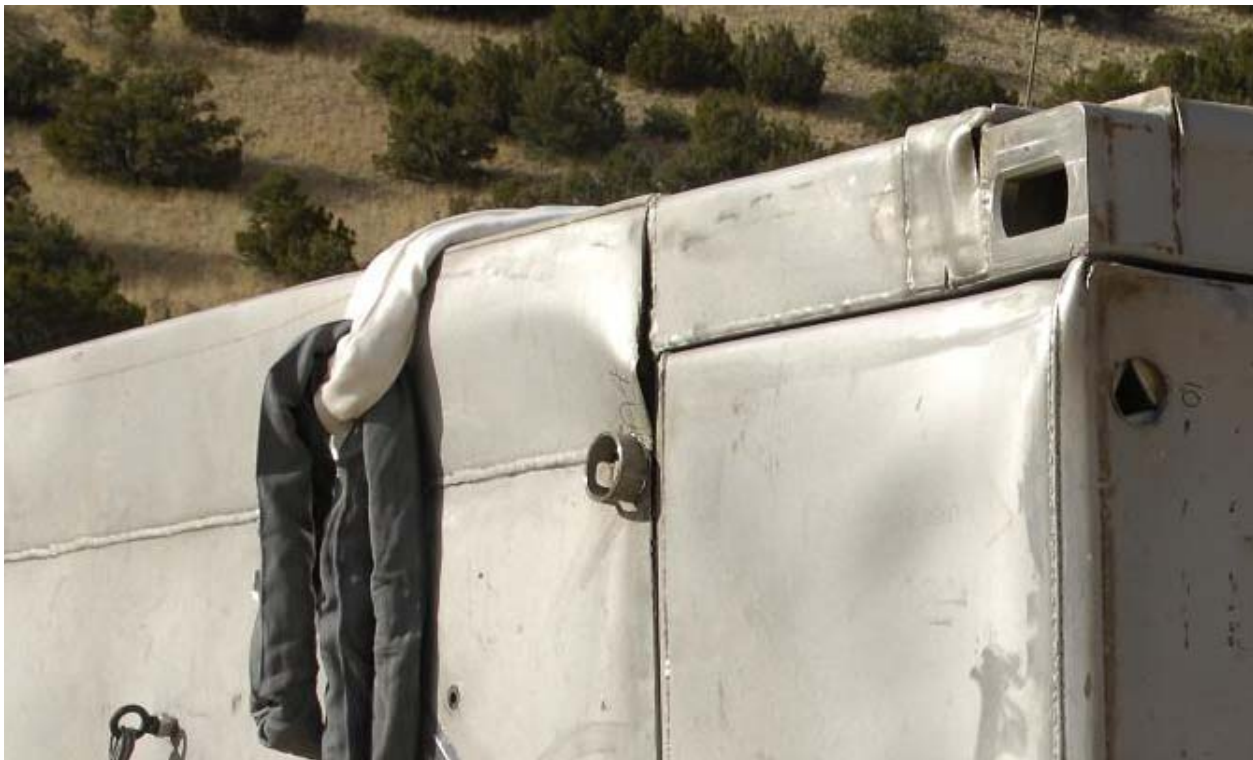
Figure 2.12.3-15 – Test LD3, Weld Tear Near Bottom of Left Cheek
