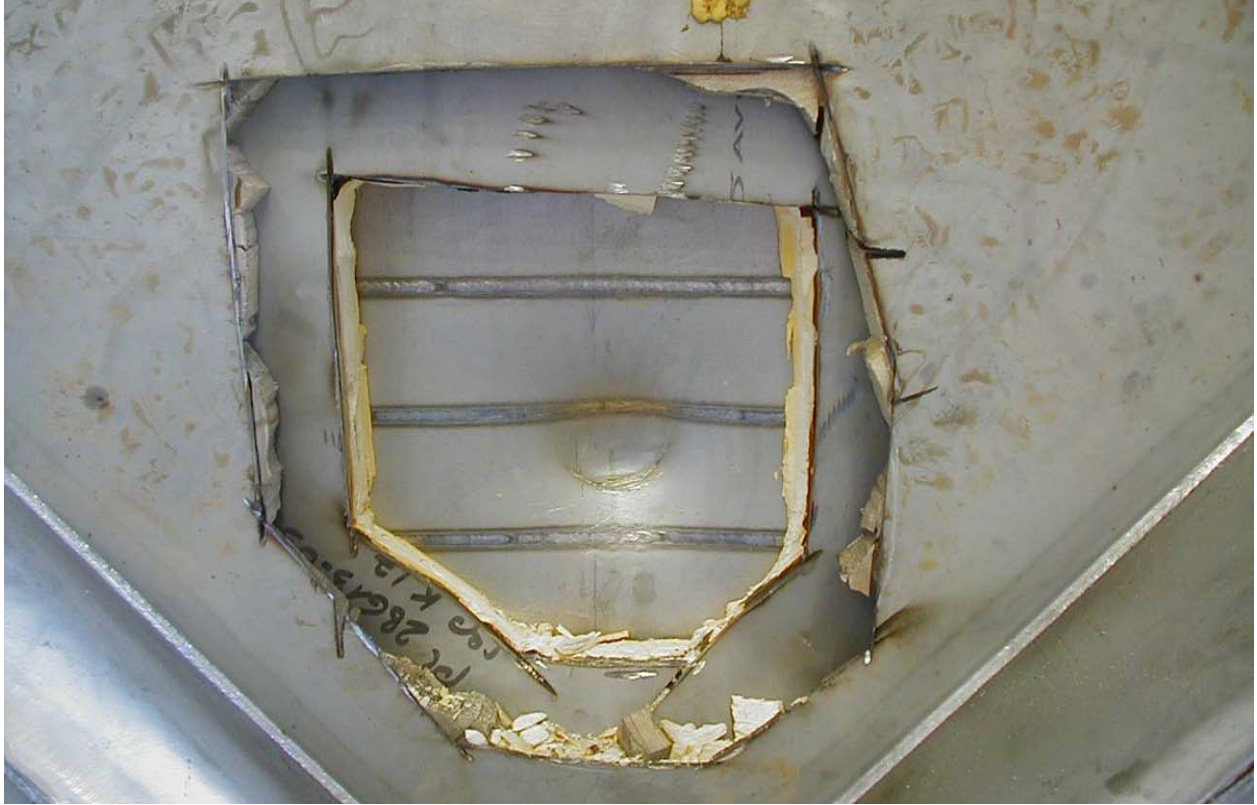
Figure 2.12.1-51 – Puncture Drop Test P4: View of Damage to CSA Structural Sheet
