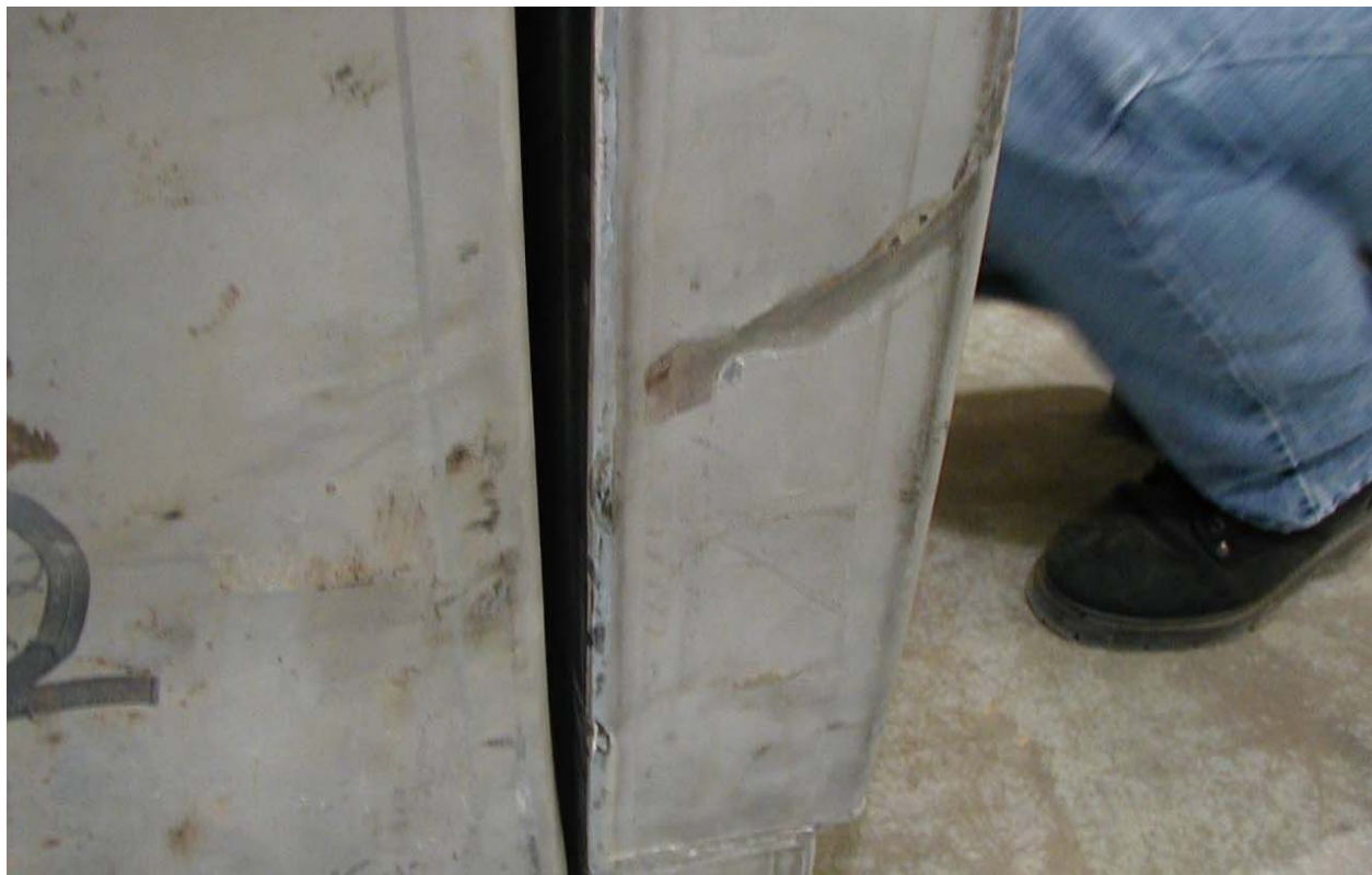
Figure 2.12.1-46 – Puncture Drop Test P2: Overall View of Cheek Damage
