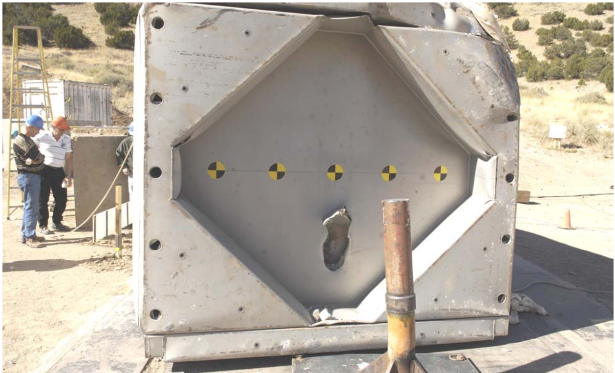
Figure 2.12.3-27 – Test LP2 Puncture Damage
