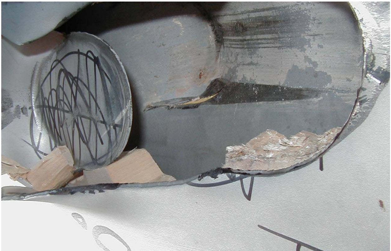
Figure 2.12.1-58 – Puncture Drop Test P205 at 30°
