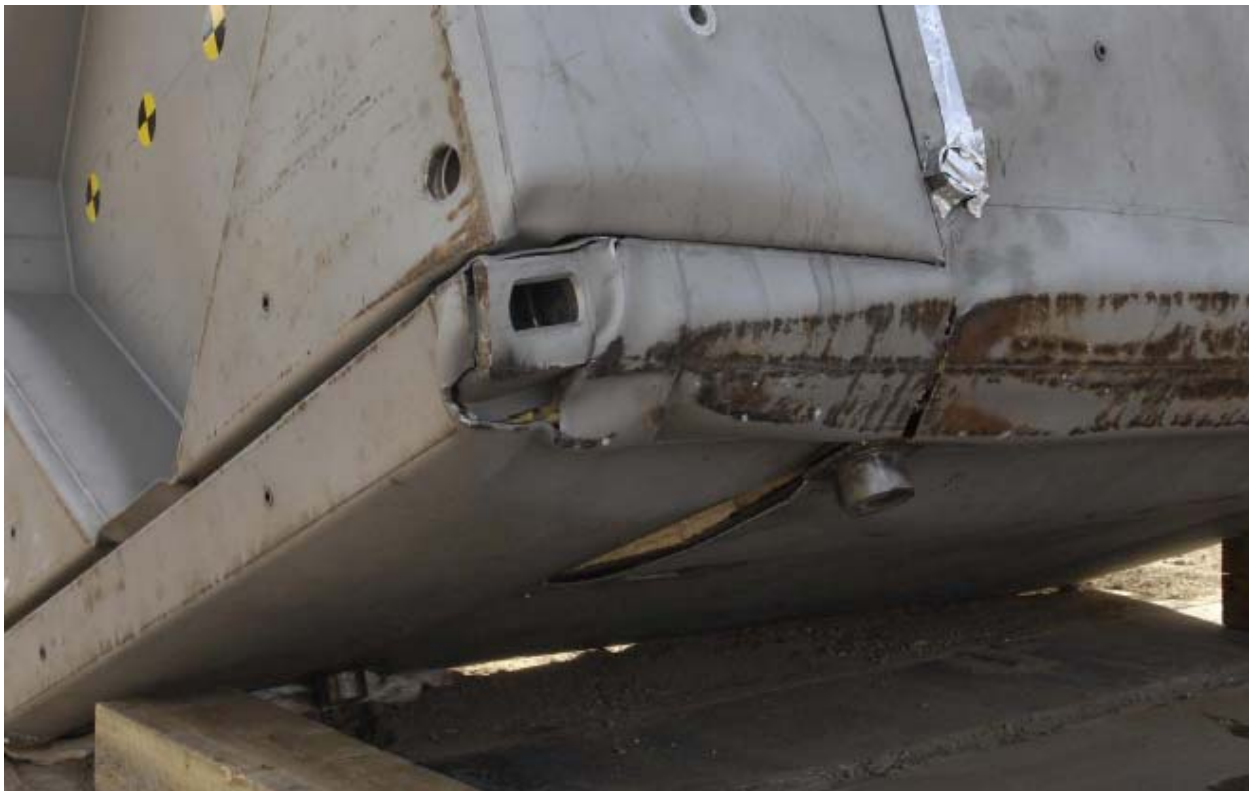
Figure 3.5-20 – Weld Tear from LD-5 Free Drop Orientation
