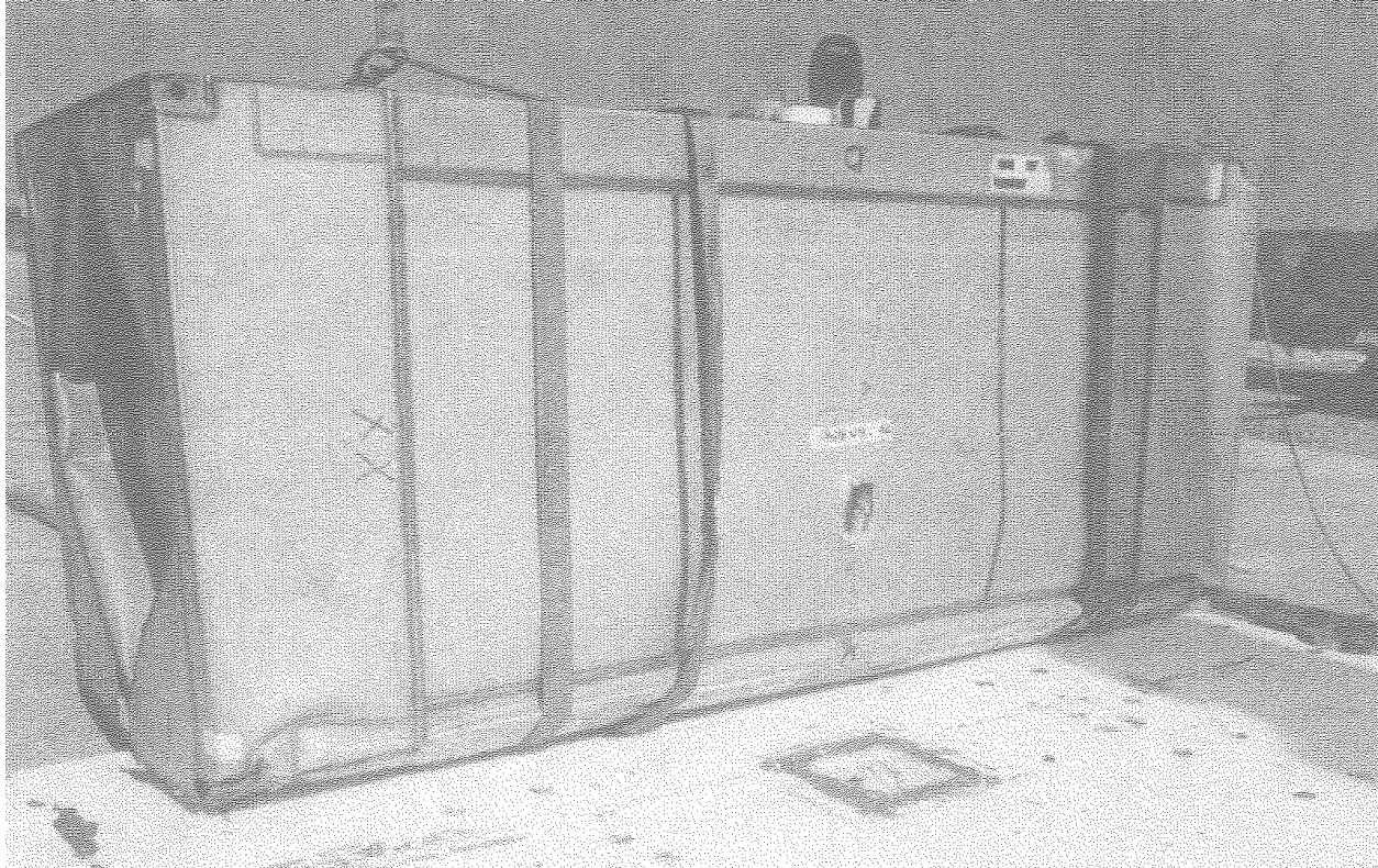
Figure 2.12.1-29 – Free Drop Test A6: Overall View of Damage Following Impact
