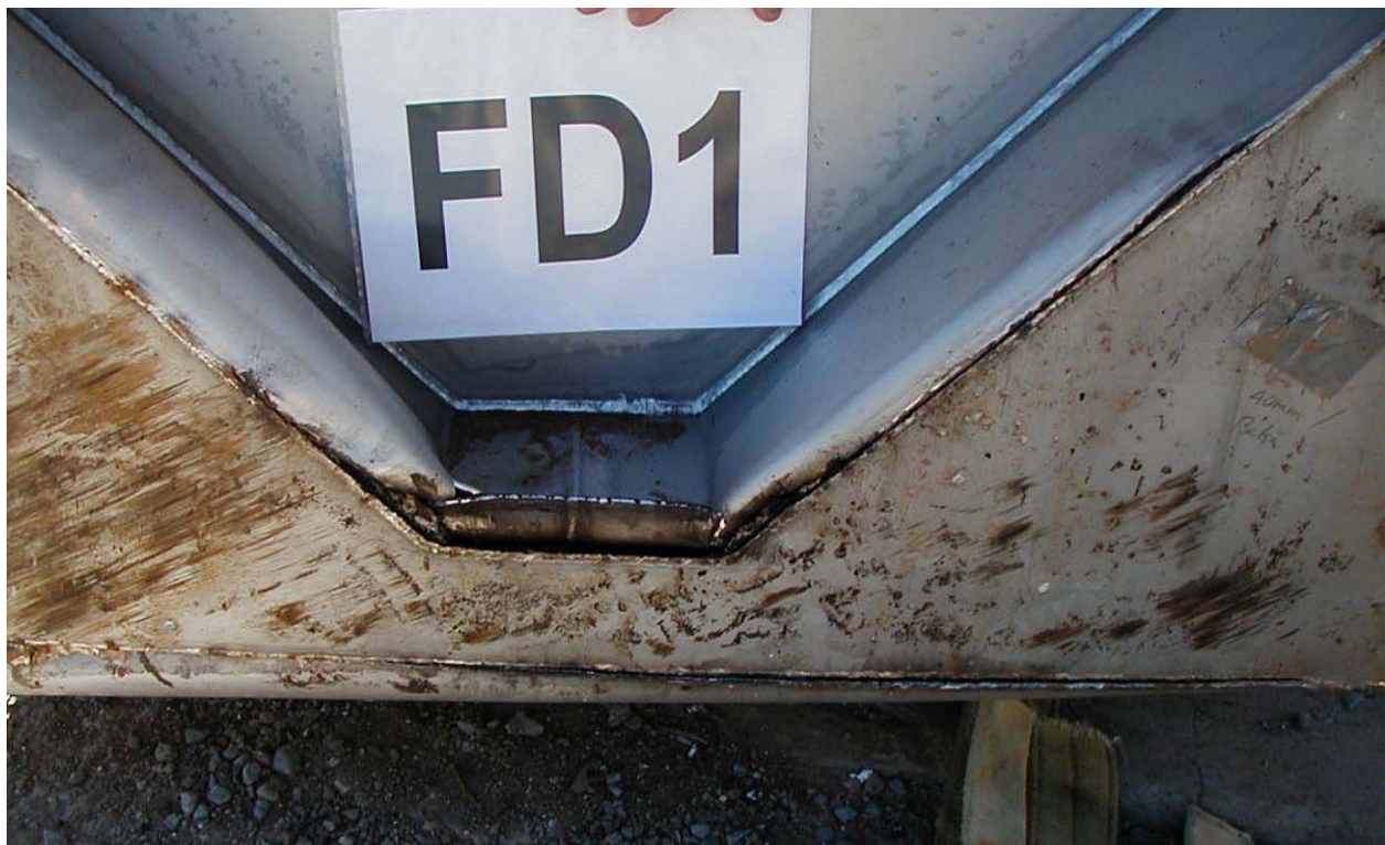
Figure 2.12.1-34 – Free Drop Test FD1: Close-up View of Weld Joint Damage
