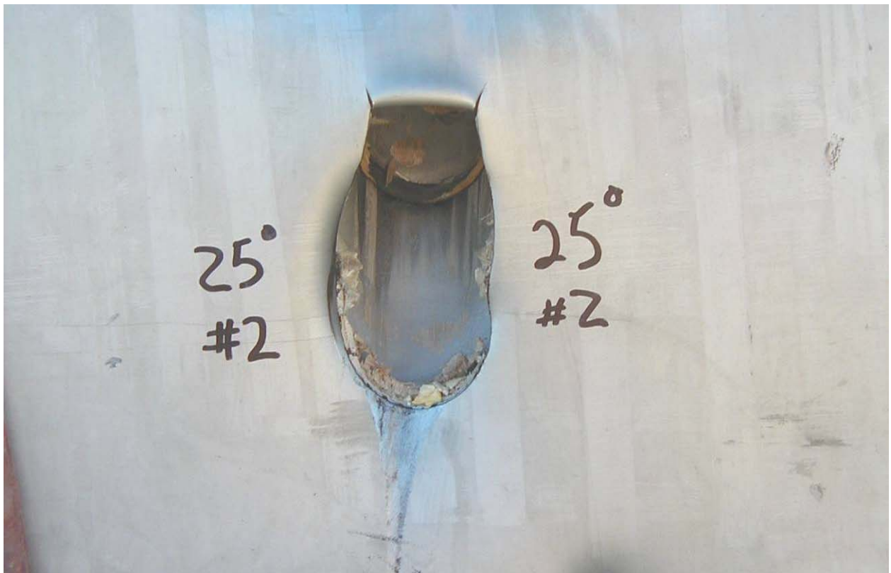
Figure 2.12.1-60 – Puncture Drop Test P405 at 25°
