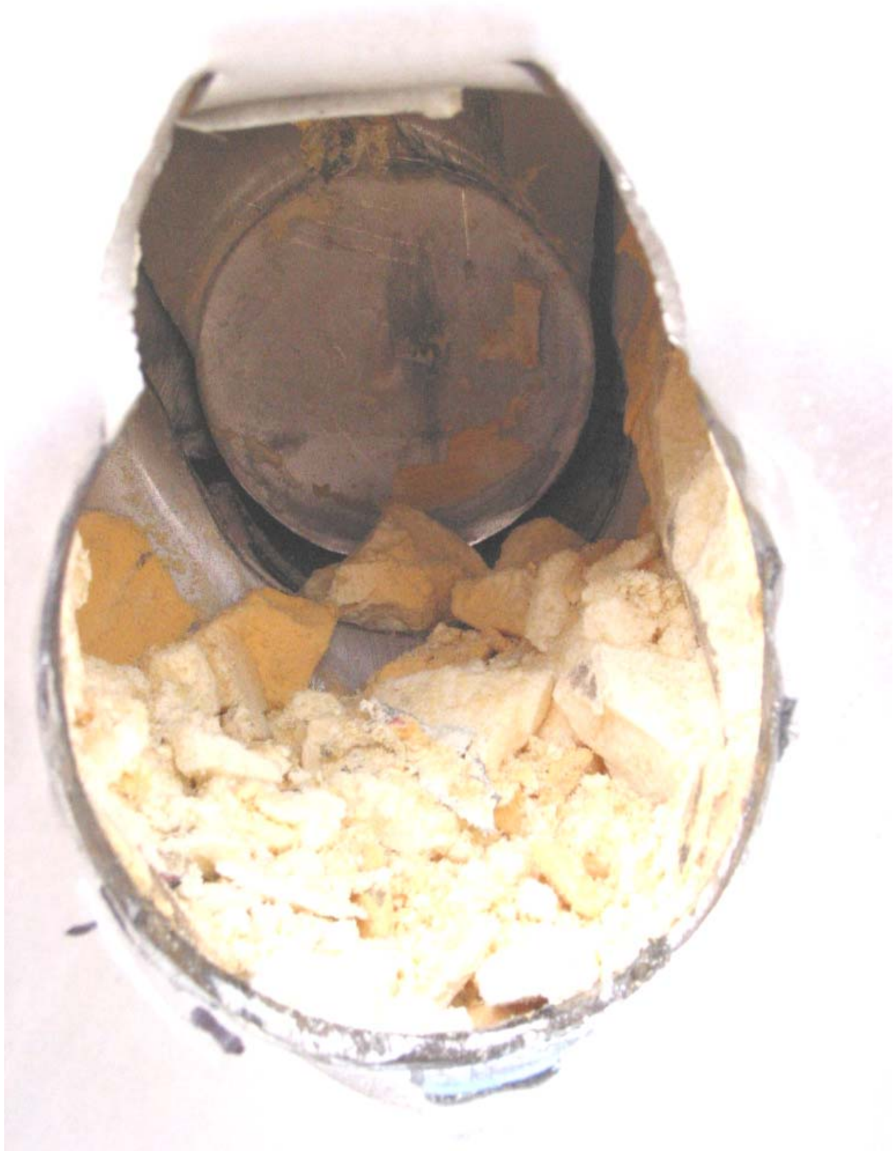
Figure 2.12.1-44 – Puncture Drop Test P1: Close-up View of Overpack Cover Damage
