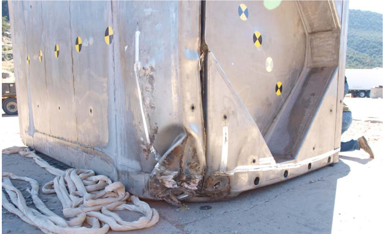
Figure 2.12.6-11 – Test LD91, CG-Over-Corner Free Drop Damage
