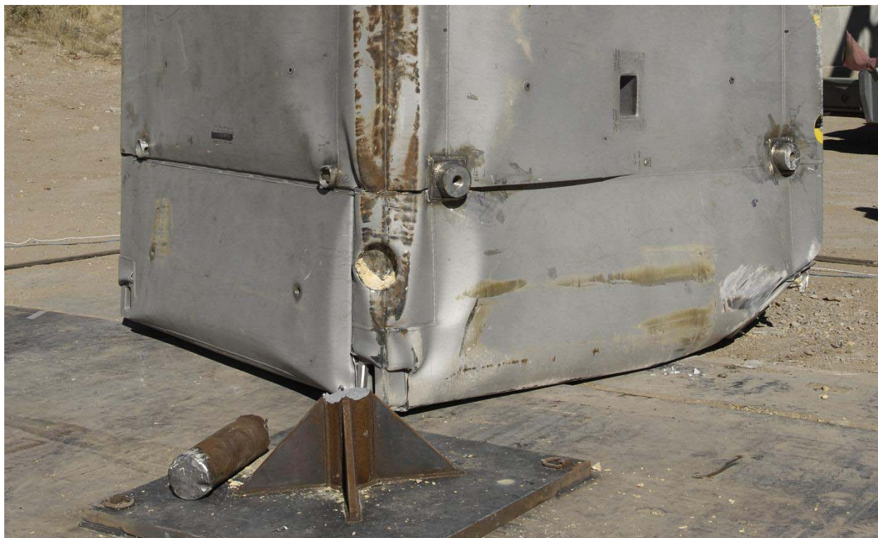
Figure 2.12.3-22 – Test LP4 Puncture Damage. Note Broken Puncture Bar
