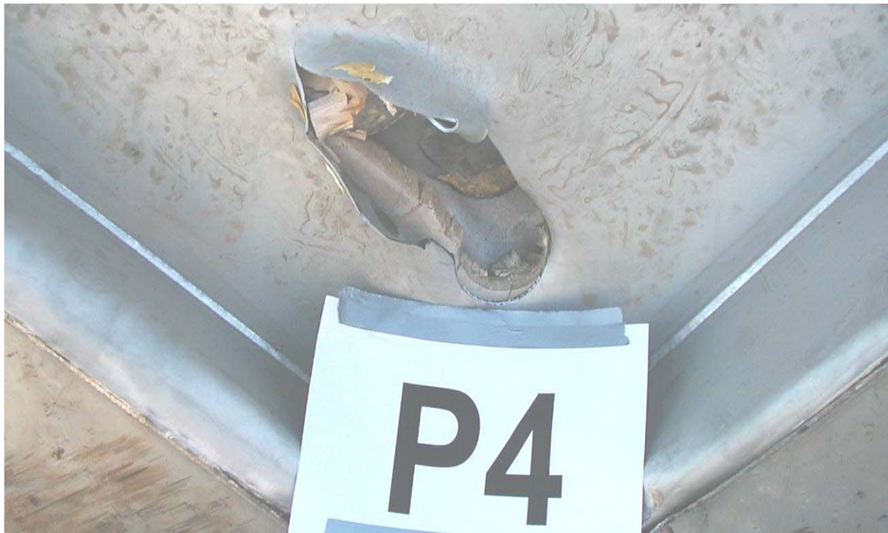
Figure 2.12.1-50 – Puncture Drop Test P4: Overall View of Damage to Closed End
