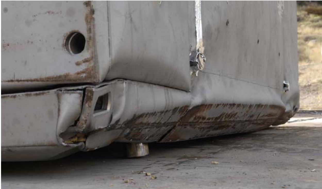
Figure 3.5-19 – Edge Deformation from LD-5 Free Drop Orientation
