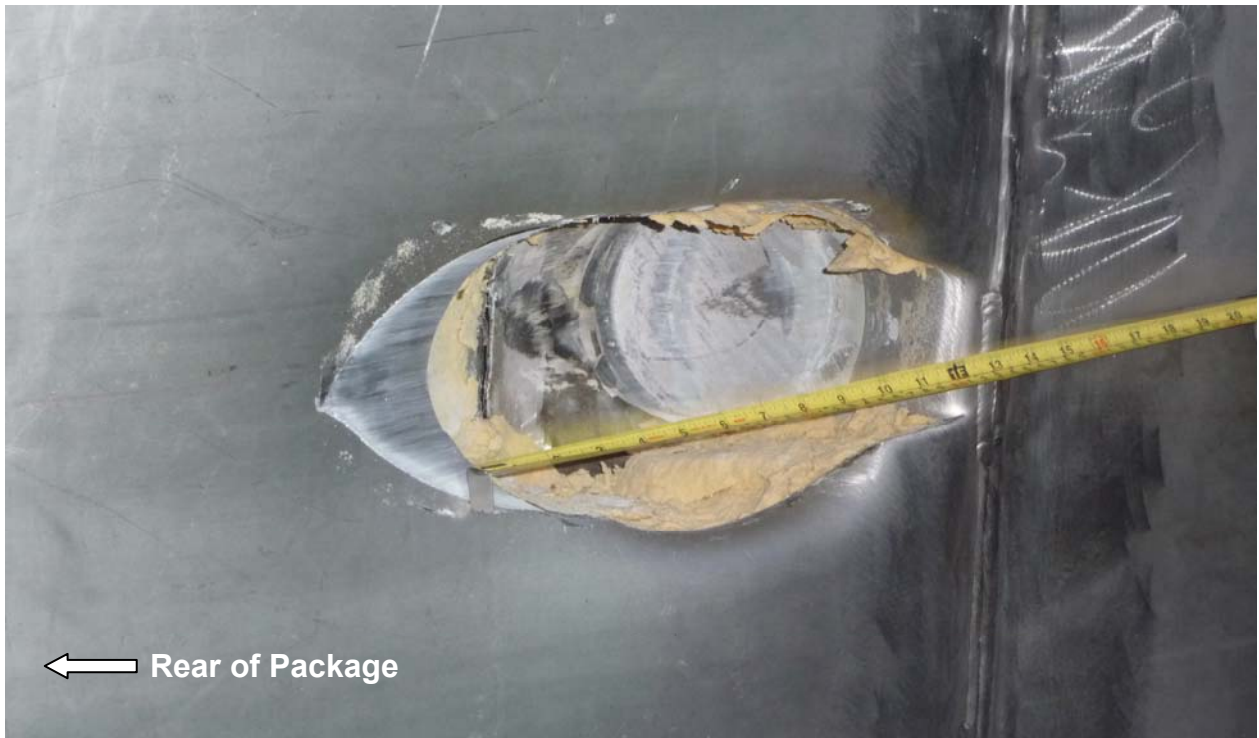
Figure 2.12.6-14 – Test LP92, Puncture on Bottom Wall Damage
