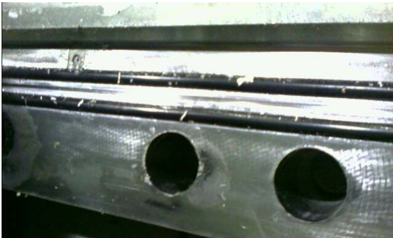
Figure 2.12.3-33 – Debris on Closure Lid Seals (Showing Large Chips)
