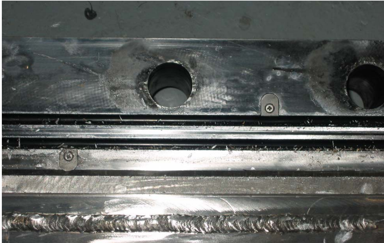
Figure 2.12.3-32 – Debris on Closure Lid Seals (Right Side, Bolt Hole #15 in Center)
