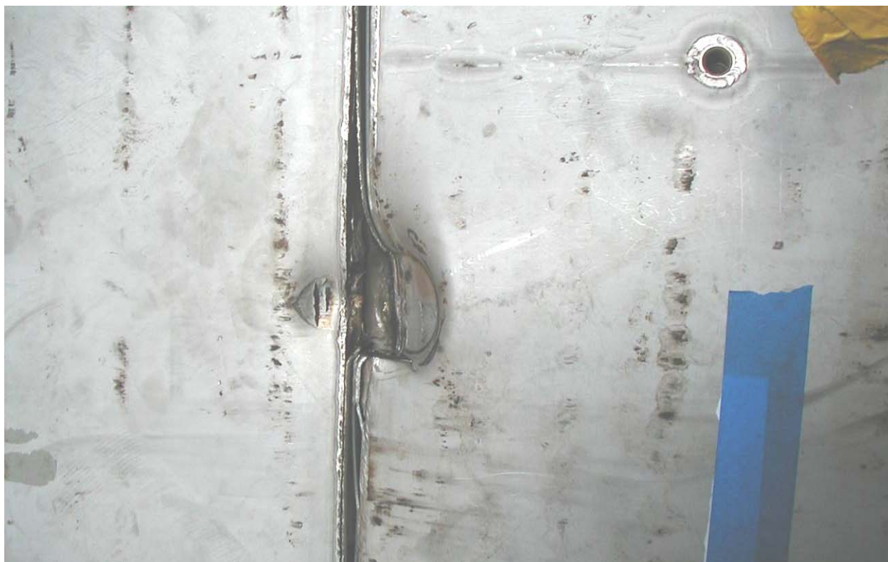
Figure 2.12.1-48 – Puncture Drop Test P3: Overall View of Damage to Overpack Cover-Body Joint
