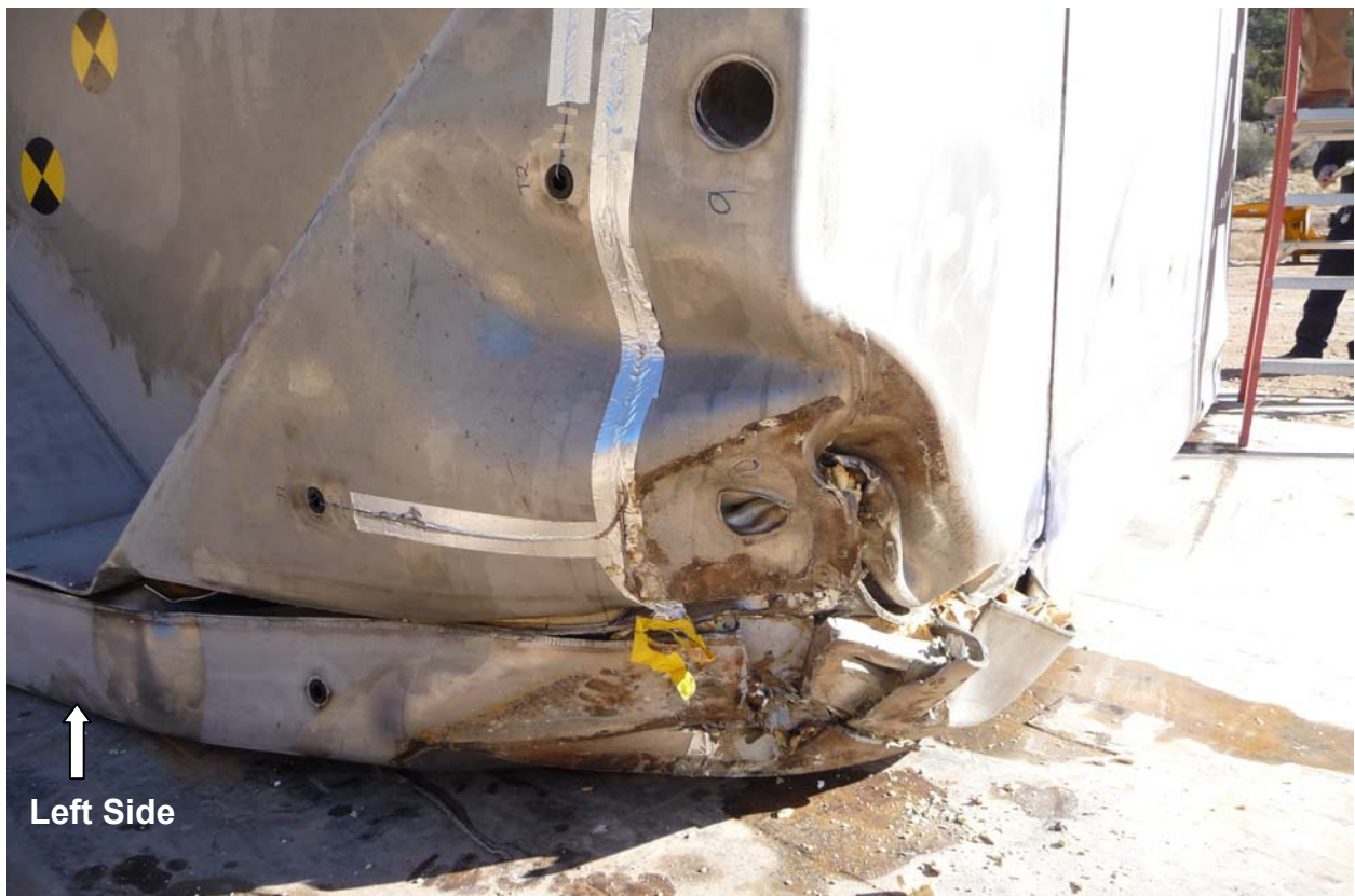
Figure 2.12.6-12 – Test LD91, CG-Over-Corner Free Drop Damage, Detail
