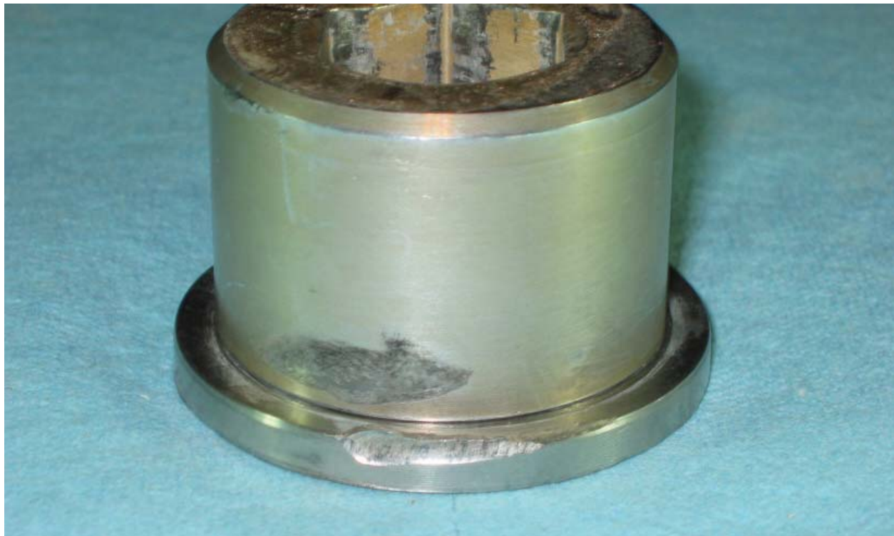
Figure 2.12.3-31 – View of Contact on Closure Bolt Head and Washer (Typical)
