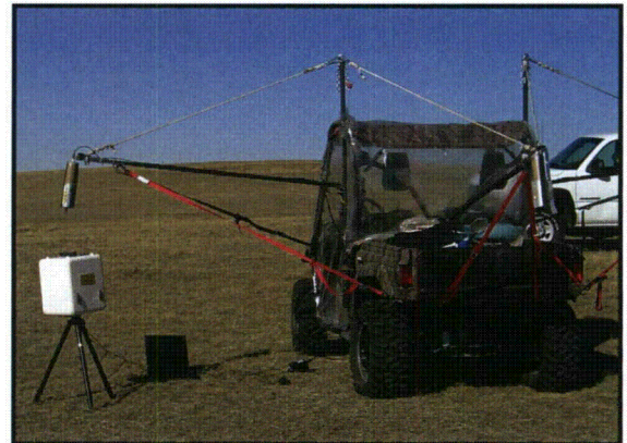
Figure 6.1-3: Measurements for cross-calibration of NaI detectors against the HPIC at a 4.5-foot NaI detector height.
