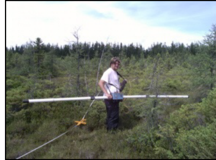
Geonics EM31 instrument used in this survey
