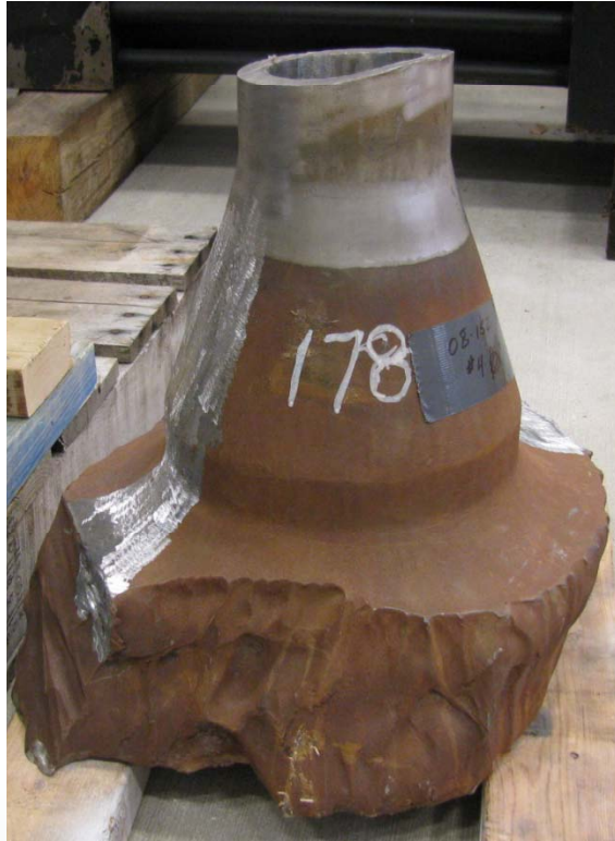
Spray nozzle - SA-508 Cl 2 forged alloy steel with type 304 SS cladding and fitted with an SA-182 F-316 SS safe end
