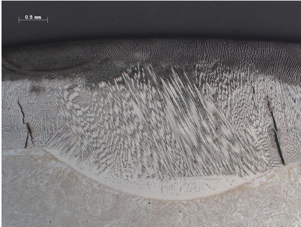
Solidification Cracks @ 25X 52M (NX74W8TW) Bead on CF8A (1.95% Si – 0.0017% S – 0.0230% P) (Courtesy of Mary Kay Havens)
