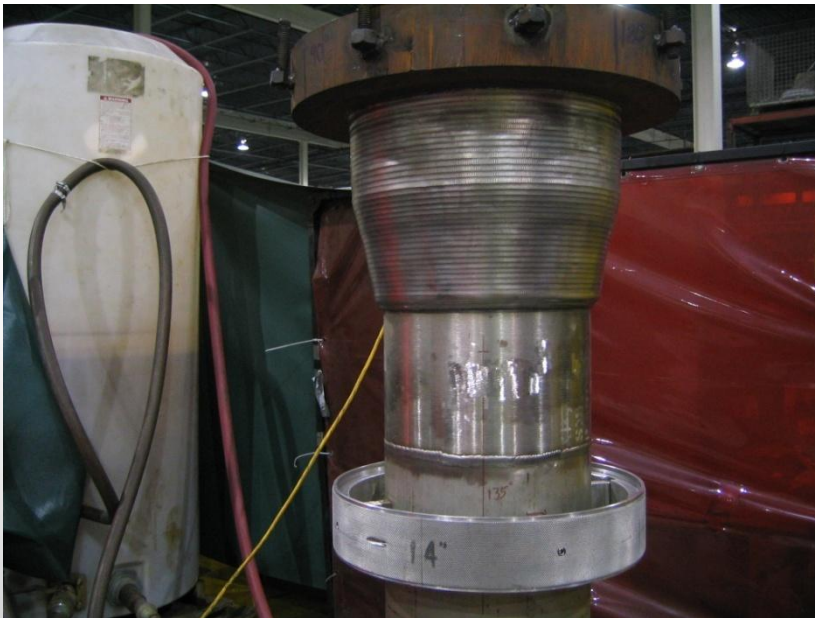
14" Surge Nozzle WOL Mockup
