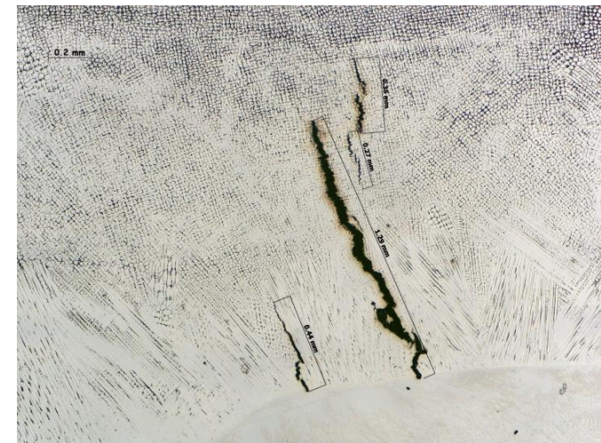
50x Micrograph of Sample #63
