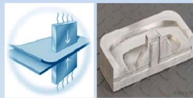
Ultrasonic welding: 20~50 kHz vibration
