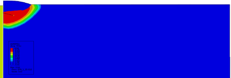
\varepsilon_w - \varepsilon_f = 0.83 > 0 , cracking
