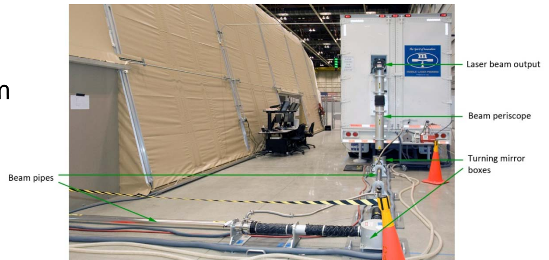
Concept of laser system trailer and beam transport pipes routed into reactor building
