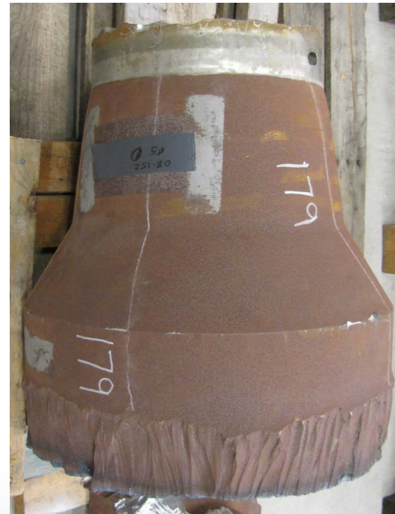
Surge nozzle - SA-508 Cl. 2 forged alloy steel with type 304 SS cladding and fitted with an SA-351 GR CF8M SS safe end.
