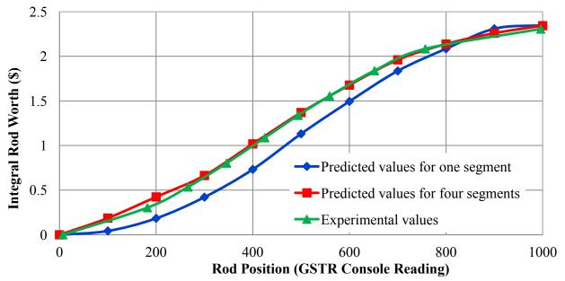
Figure 1. Shim1 rod reactivity worth curve showing the improvement in the model's predictive capability
