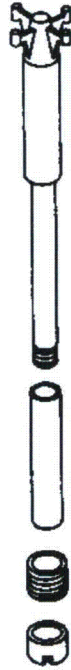
Figure 4-34 Typical Westinghouse core support column. Core support column bolts fasten the top of the support column to the lower core plate
