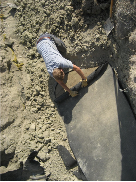
Fig. A.18. Removing lysimeter GDL for laboratory analysis.
