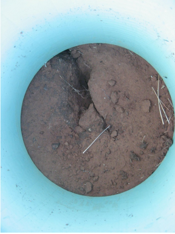
Fig. A.89. Macroscopic flow path visible at bottom of TSB.
