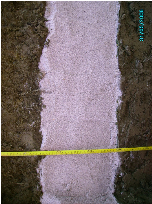
Fig. A.55. Close up of capillary barrier in AO1.
