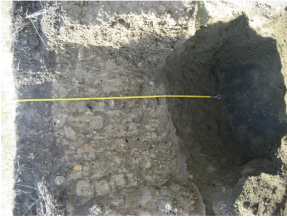
Fig. A.70. Thicker (3 ft) CCL profile (desiccated across profile).
