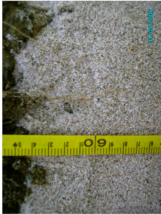
Fig. A.55. Close up of capillary barrier in AO1.
