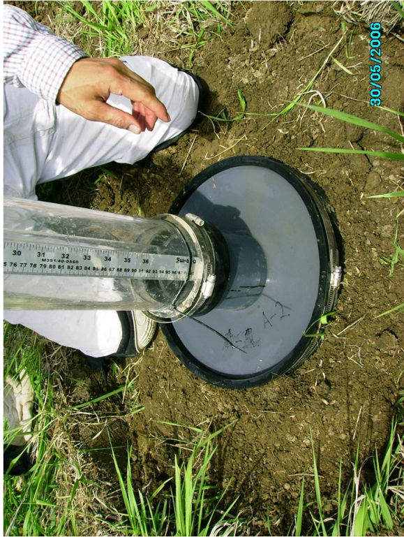
Fig. A.43. Installing TSB, rough bottom to avoid smearing.
