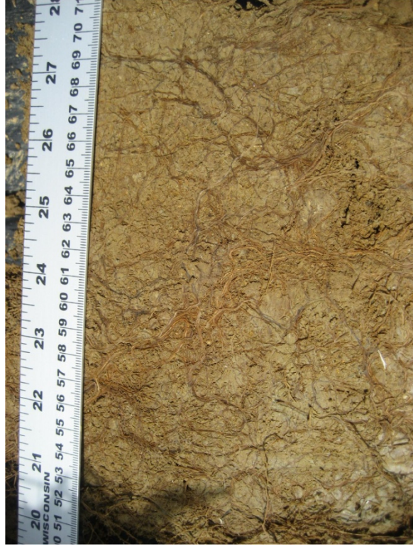
Fig. A.48. Conventional cover profile (CCL below GM).
