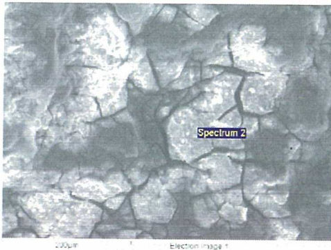
Figure 3-22: Representative Image of P-7A Coupling Showing No Pitting
