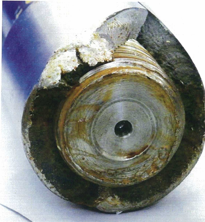
Half of coupling 11-P7C-6F remaining on shaft No. 6 exhibited damage on its fracture surface from contact with the mating coupling half and shaft 5, which likely occurred after fracture event.
