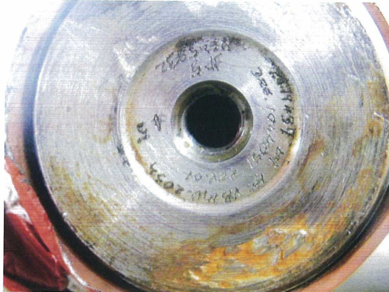
End of shaft No. 5 exhibited gouging damage likely from post 11-P7C-6F final failure.
