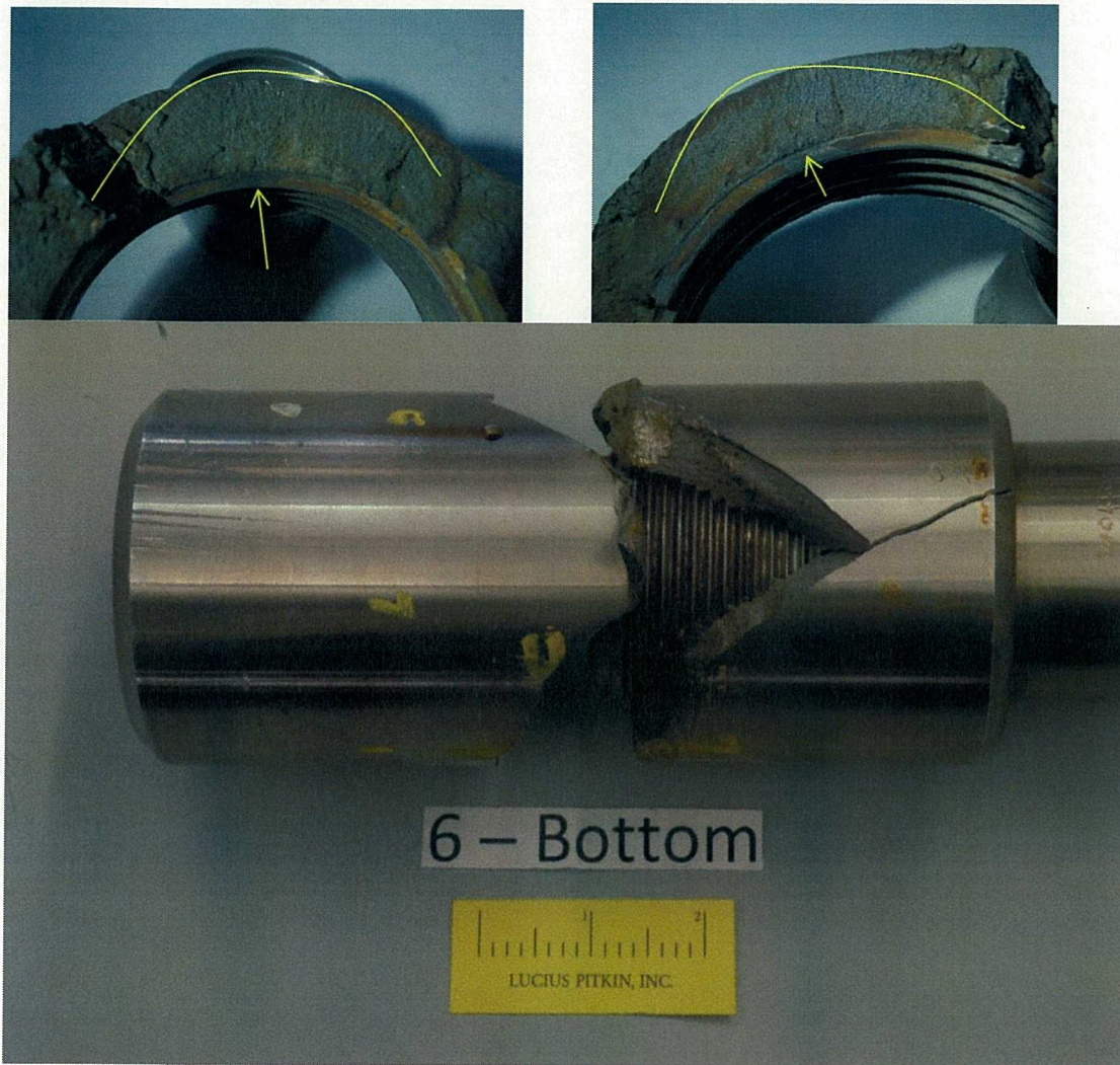
Figure 3: Failed Coupling #6 from P-7C Service Water Pump, Fracture Surfaces
