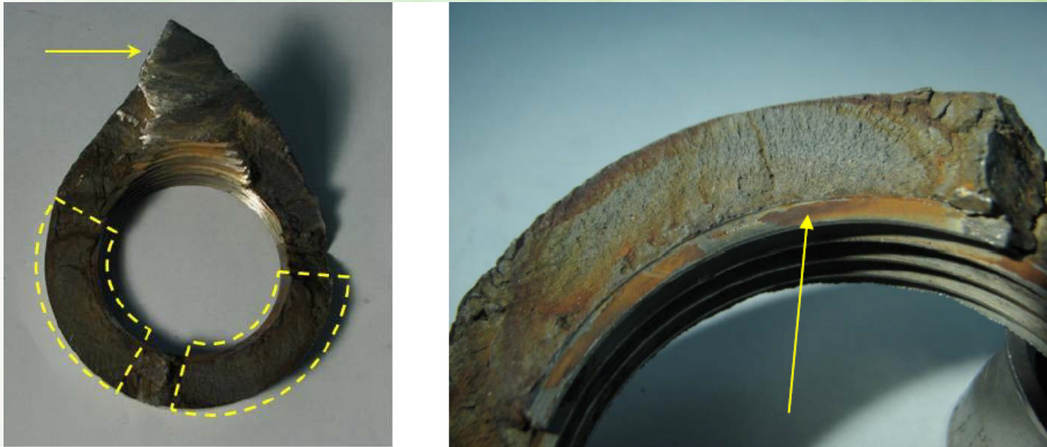
Fracture Surface of 2011 Failed Coupling No. 6 in P-7C
