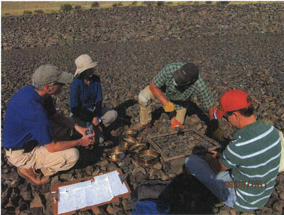
LKV 9/2011. PL-5. DOE representatives watching rock monitoring on west side slope. A grid is used to mark rocks for gradation and durability monitoring. Marked rocks are first sized using a series of sieves and then identified by rock type and durability class.
