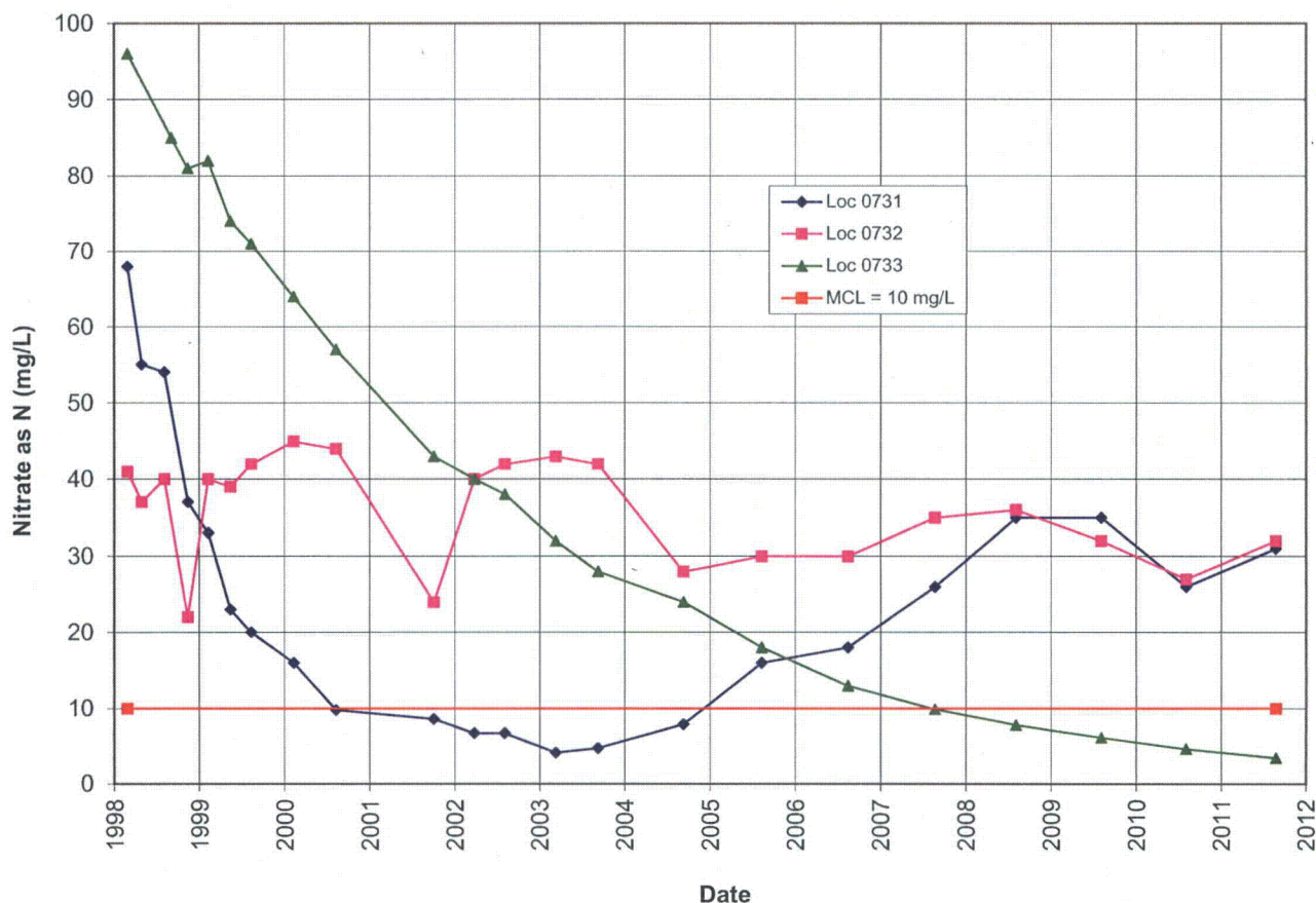
Figure 6-3. Time-Concentration Plots of Nitrate (as Nitrogen) in Groundwater at the Grand Junction Disposal Site
