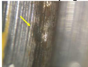
Pitting near root at middle of Coupling No. 5 (Stereomicroscopy 40X)
