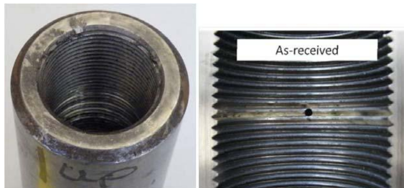
Figure 3-2: Contrast Thread Coating (As-Received) on P-7C Failed and Cracked Couplings to P-7A Coupling
