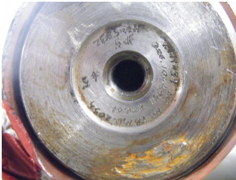
End of shaft No. 5 exhibited gouging damage post 11-P7C-6F final failure.
