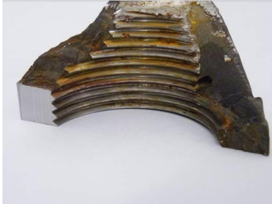
Figure 0-3: Visual of Fracture Surface on Coupling 11-P7C-6F
