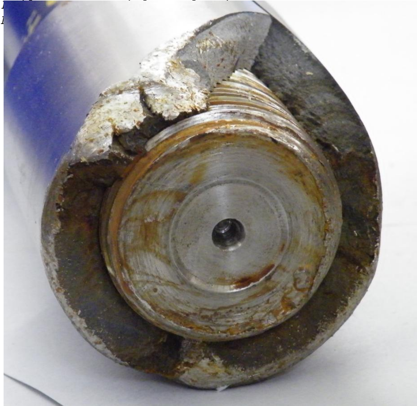
Half of coupling 11-P7C-6F remaining on shaft No. 6 exhibited damage on its fracture surface from contact with the mating coupling half and shaft 5, which occurred after fracture event.
