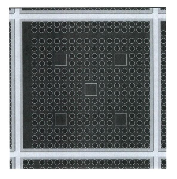
Figure B.6.6-19 Square Guide Tube – KENO Model
