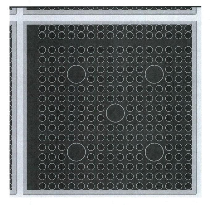
Figure B.6.6-21 Design Basis Damaged Fuel KENO Model – Fuel Compartment View
