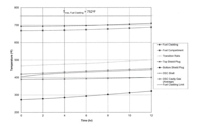
Figure B.4.6-18 Temperature Time History for 32PTH2 DSC with 37.2 kW in OS200FC TC, Air Circulation turned off/ Air Circulation Failure during Transfer Operations (Load Case # T10)
