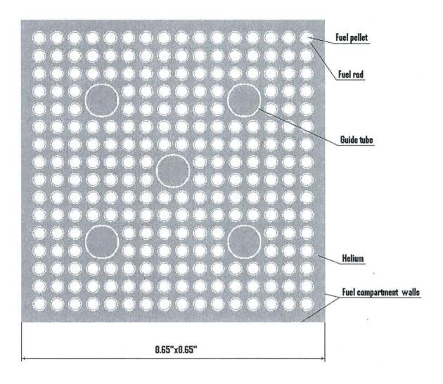
Figure B.4.9-1 Cross-section of CE 16×16 Class Fuel Assembly in a Fuel Compartment
