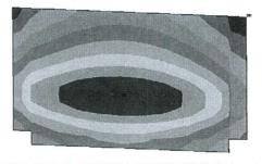
$\frac{329.943}{346.886}$   $\frac{363.83}{340.773}\frac{397.717}{414.66}$   $\frac{431.604}{448.547}\frac{465.491}{482.434}$  Side heat shield temperature profile
