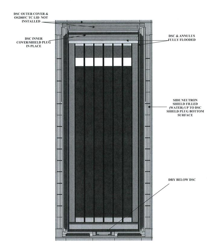
Figure B.5.5-21 32PTH2 DSC in OS200FC TC MCNP5 Model, Decontamination Configuration
