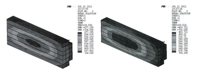
32PTH2 DSC in TC Vertical-Normal-Steady-State, 120F, 31 kW(HL2C#4)  $Fuel\ Cladding$
