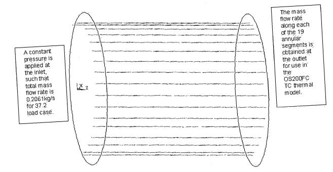
Figure B.4.5-1 Finite Element Mesh of Flow Rate Model with FLUID116 Elements
