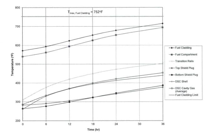
Figure B.4.6-16 Temperature Time History for 32PTH2 DSC with 37.2 kW in OS200FC TC, without Air Circulation, Normal Hot, Vertical Transient Operations (Load Case T6)
