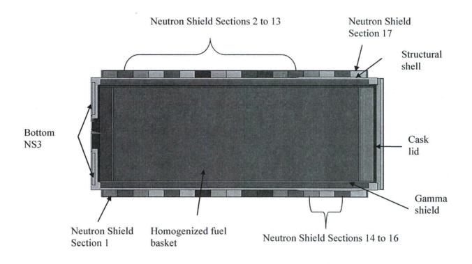
Figure B.4.5-2 Finite Element Model of the OS200FC TC with the 32PTH2 DSC
