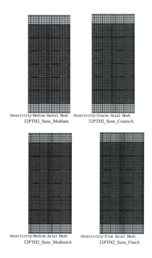
Figure B.4.6-8 Mesh Densities of 32PTH2 DSC Model in Axial Direction
