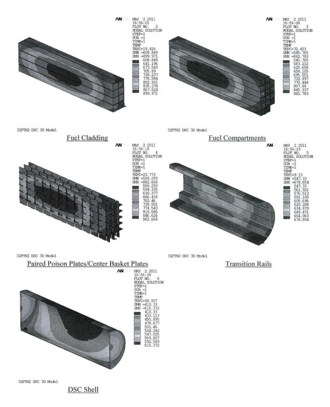
Figure B.4.6-19 Temperature Distribution for 32PTH2 DSC with 37.2 kW with Damaged FAs in OS200FC TC, Accident, Loss of Neutron Shield with Loss of Air Circulation Accident Condition
