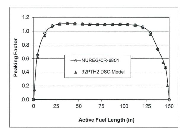
Figure B.4.6-6 Peaking Factor Curve for PWR Fuel Assemblies
