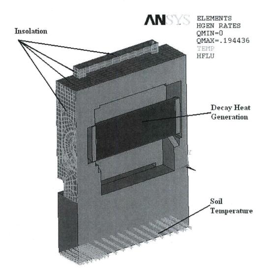
Figure B.4.4-3 Heat Load, Insolation, and Fixed Temperature Boundary Conditions in AHSM-HS Model
