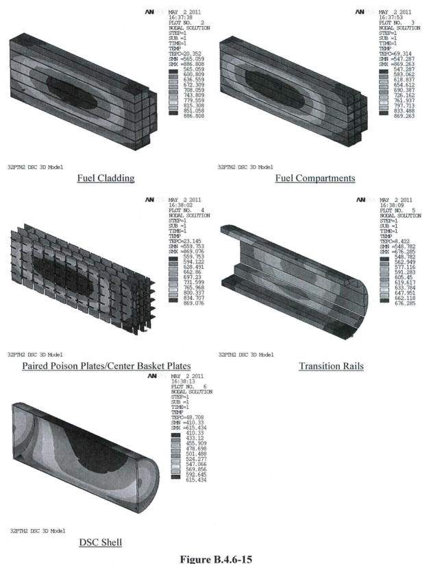
Temperature Distribution for 32PTH2 DSC with 37.2 kW in OS200FC TC, Accident, Loss of Neutron Shield with Loss of Air Circulation Accident Condition (Load Case T9)
