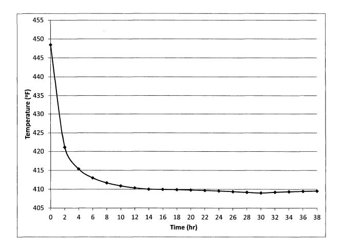
Figure B.4.5-8 Maximum DSC Shell Temperature versus Time with Air Circulation starting at End of Time limit for Load Case T7 with 37.2 kW and 117°F Ambient
