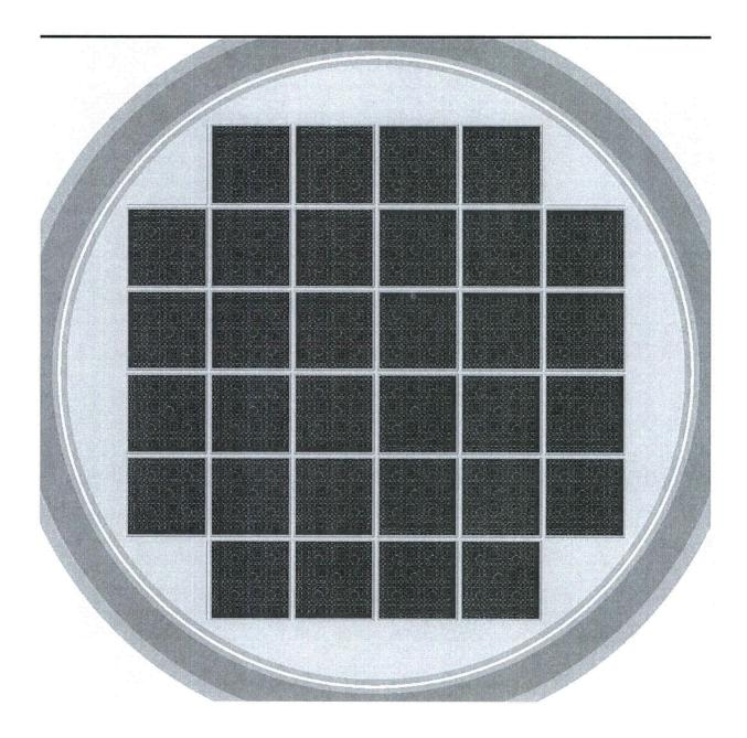
Figure B.6.6-20 Design Basis Damaged Fuel KENO Model
