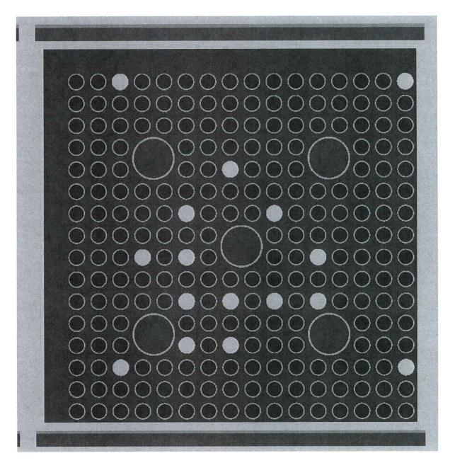
Figure B.6.6-11 Example of Reconstituted Fuel Rod Locations, 16 shown
