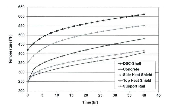
Figure B.4.4-8 AHSM-HS with 32PTH2 DSC, Component Temperature History for Accident Blocked Vent Condition, 37.2 kW
