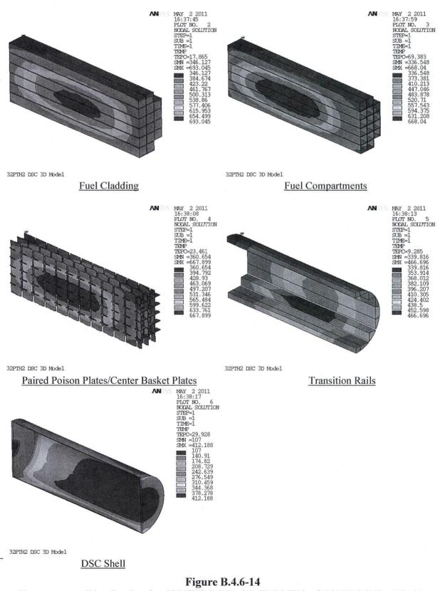
Temperature Distribution for 32PTH2 DSC with 37.2 kW in OS200FC TC, with Air Circulation, Off-Normal Hot, Horizontal Steady-State Operations (Load Case T8)
