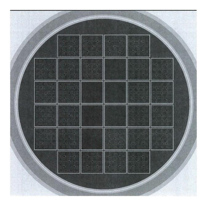
Figure B.6.6-12 Example of Empty Fuel Compartment Location, 6 shown
