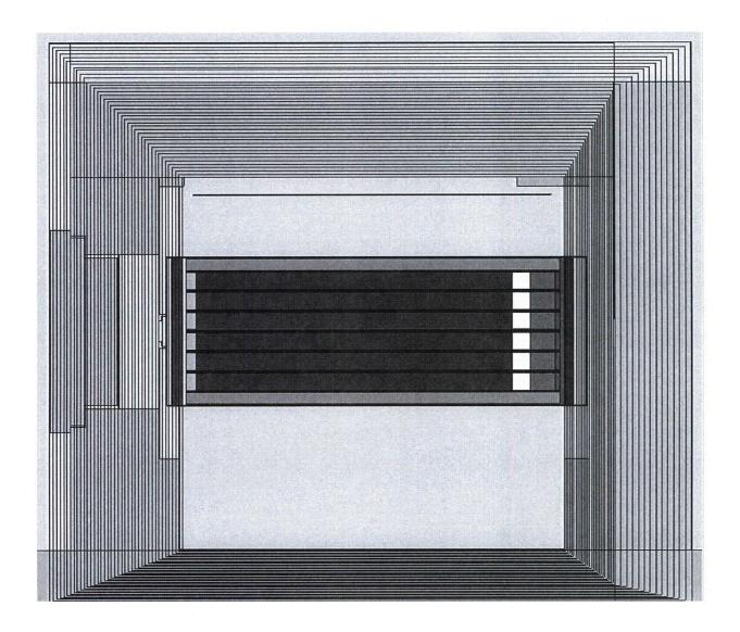
Figure B.5.5-19 32PTH2 DSC within AHSM-HS MCNP5 Model, z-y View, Cut-through at x = 2 cm
