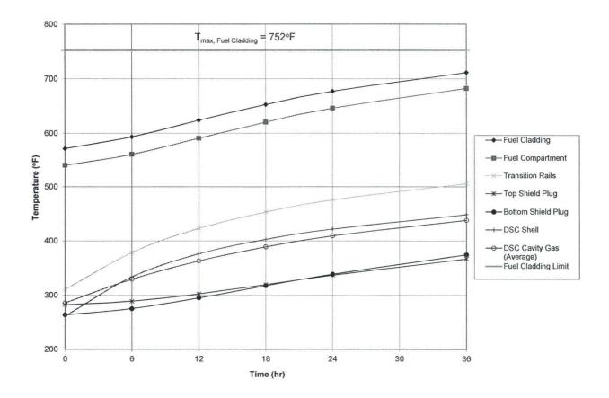
Figure B.4.6-17 Temperature Time History for 32PTH2 DSC with 37.2 kW in OS200FC TC, without Air Circulation, Off-Normal Hot, Horizontal, Transient Operations (Load Case T7)
