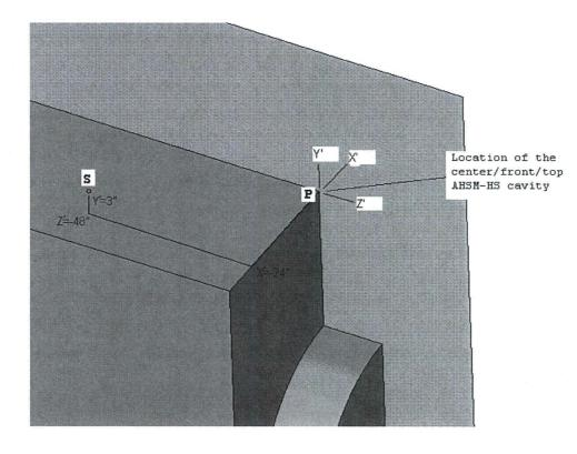
Figure B.4.4-9 Temperature Sensor Location in AHSM-HS Model
