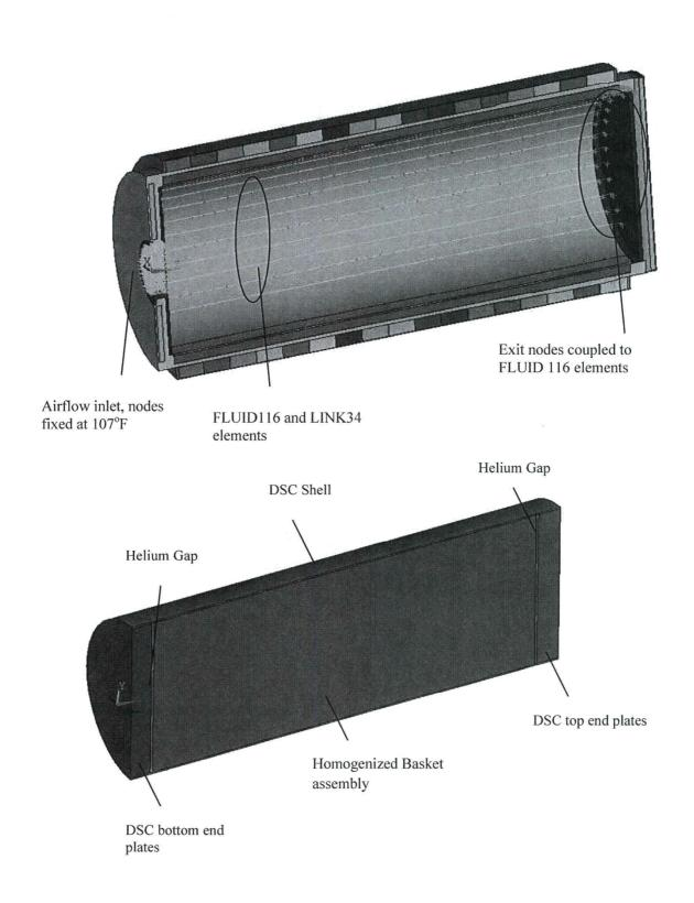
Figure B.4.5-3 OS200FC TC Finite Element Model, Components
