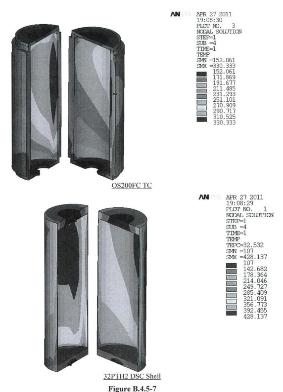
Temperature Distribution for OS200FC TC with 32PTH2 DSC @ 37.2 kW, With Air Circulation, Off-Normal Hot, Horizontal Steady-State Operations (Load Case T8)
