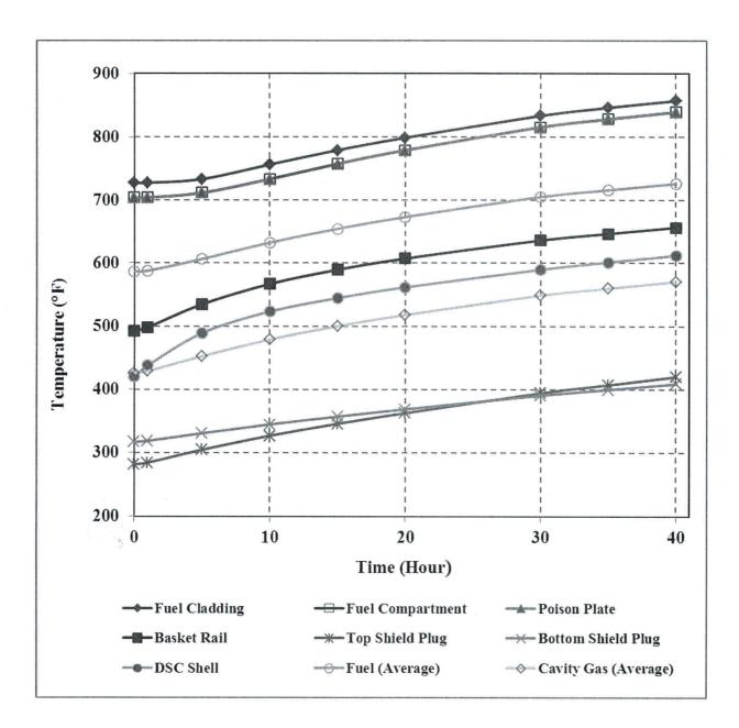
Figure B.4.6-11 Time-Temperature Histories for 32PTH2 DSC, Blocked Vent, 37.2 kW/HLZC#1 (Load Case S7)
