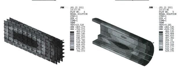
32PTH2 DSC in TC Vertical-Normal-Steady-State,120F,31 kW(HLZC#4)
