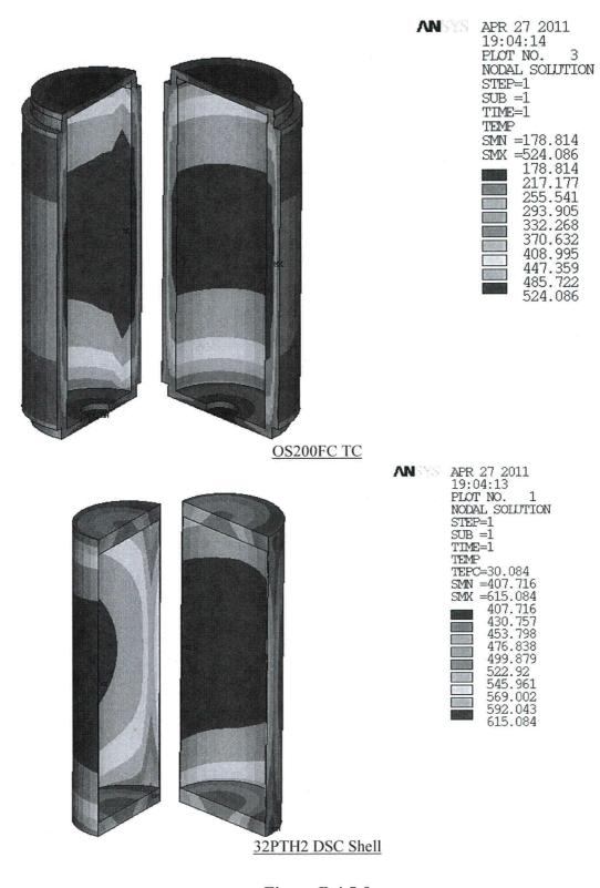
Figure B.4.5-9 Temperature Distribution for OS200FC TC with 32PTH2 DSC @ 37.2 kW, Accident Loss of Neutron Shield with Loss of Air Circulation Accident Condition, Horizontal (Load Case T9)
