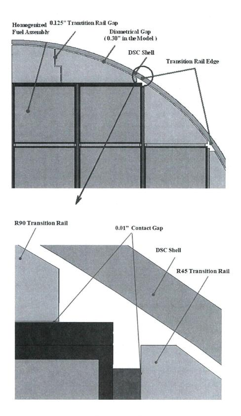
Figure B.4.6-3 32PTH2 DSC Model – Gaps in the Basket Assembly
