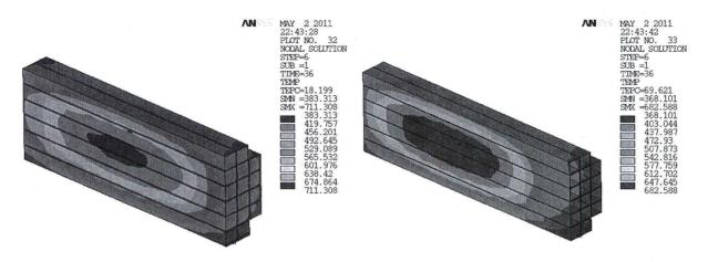
32PTH2 DSC in TC Off-Normal-Transient,107F, 37.2 kW (HLZC#1)  $Fuel \ Cladding$
