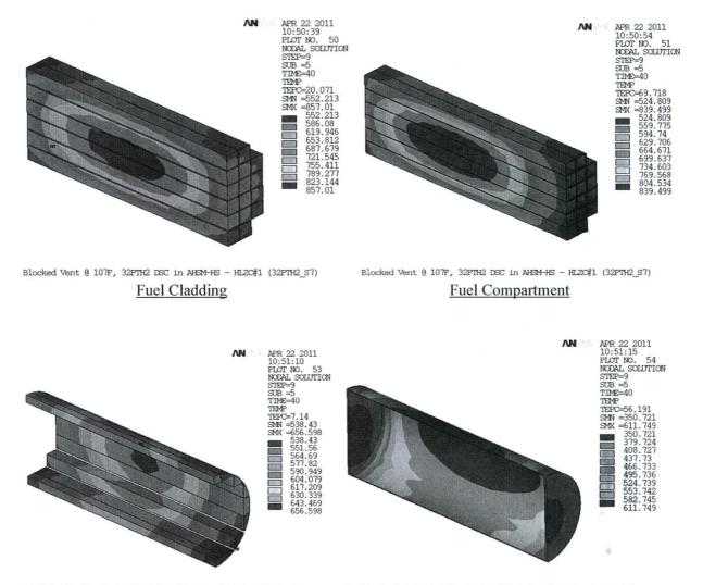
(32PTH2\_S7) Blocked Vent @ 107F, 32PTH2 DSC in AHSM-HS - HL2C#1 (32PTH2\_S7) <u>32PTH2 DSC Shell</u>
