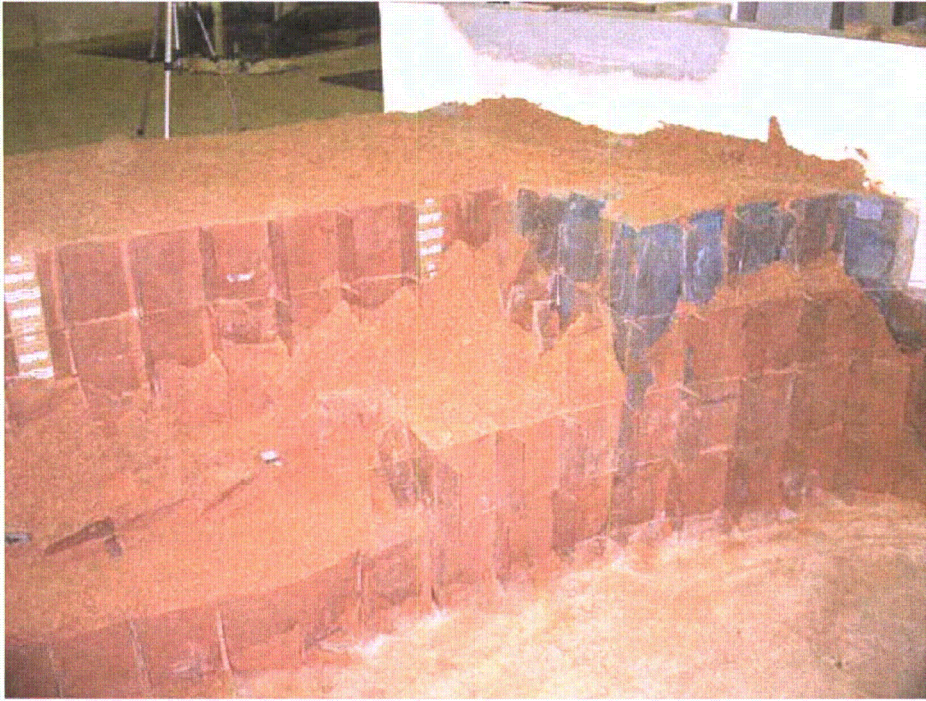
Figure 2-118. Completed sand and mixture fill, left concrete wall abutment
