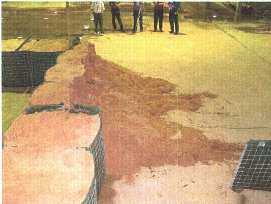
Figure 2-94. Outer wall removed from one unit on right wall
