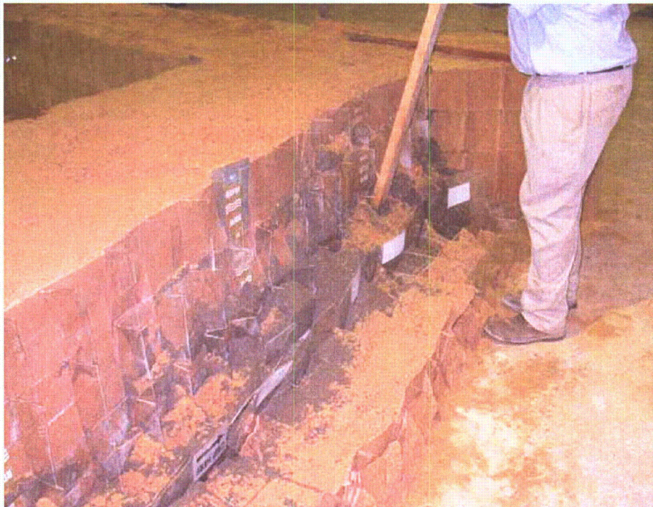
Figure 2-121. Mixture fill and tamping in center wall toe grid
