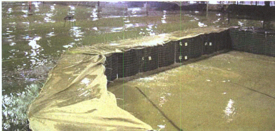
Figure 2-81. Wave overtopping along center wall
