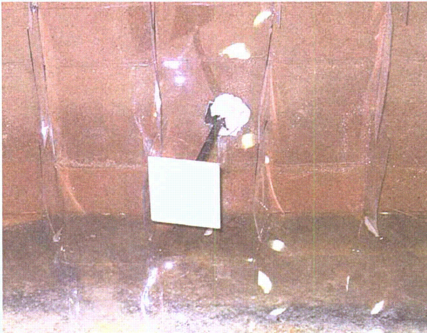
Figure 2-124. Typical laser target installation
