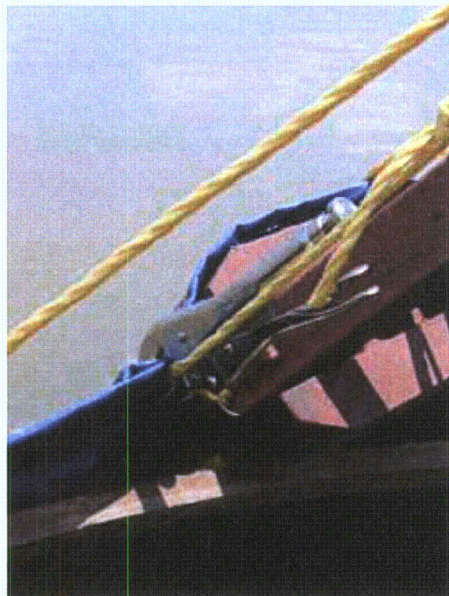
Figure 3-168. Sagging liner repair (repair 1)
