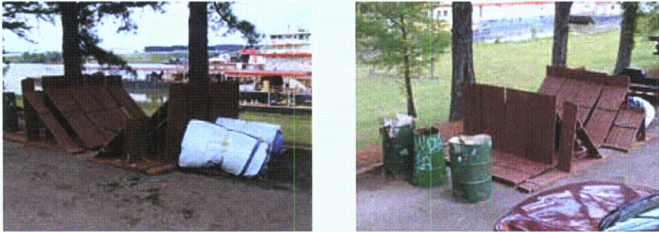
Figure 3-145. Portadam as delivered to Vicksburg
