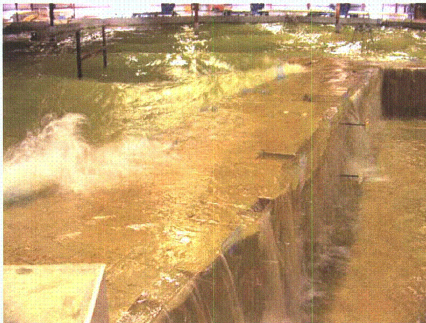
Figure 2-151. Waves overtopping left wall
