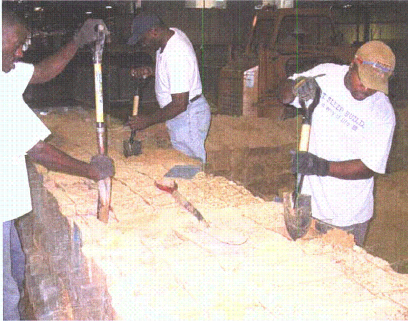
Figure 2-169. Removing sand using shovels
