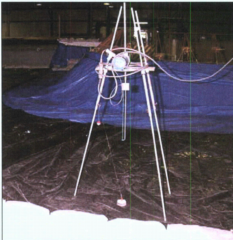
Figure 2-214. Pool elevation sensor placed on center apron
