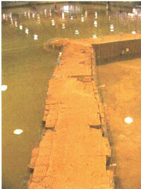
Figure 2-149. Surface erosion on left wall at conclusion of test
