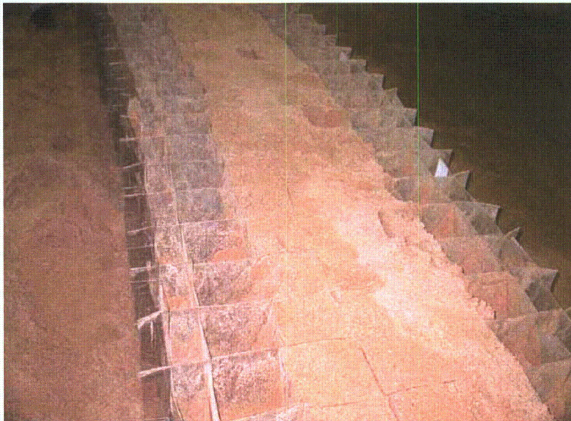
Figure 2-170. Removed sand from outer grid cells
