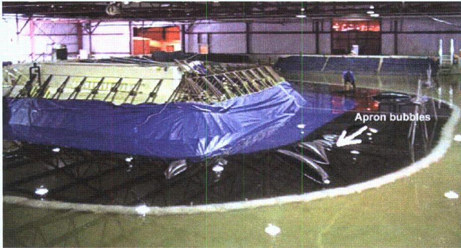
Figure 2-215. Air bubbles beneath apron
