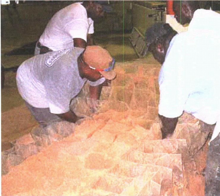
Figure 2-171. Loosening grid unit to reduce frictional resistance from sand
