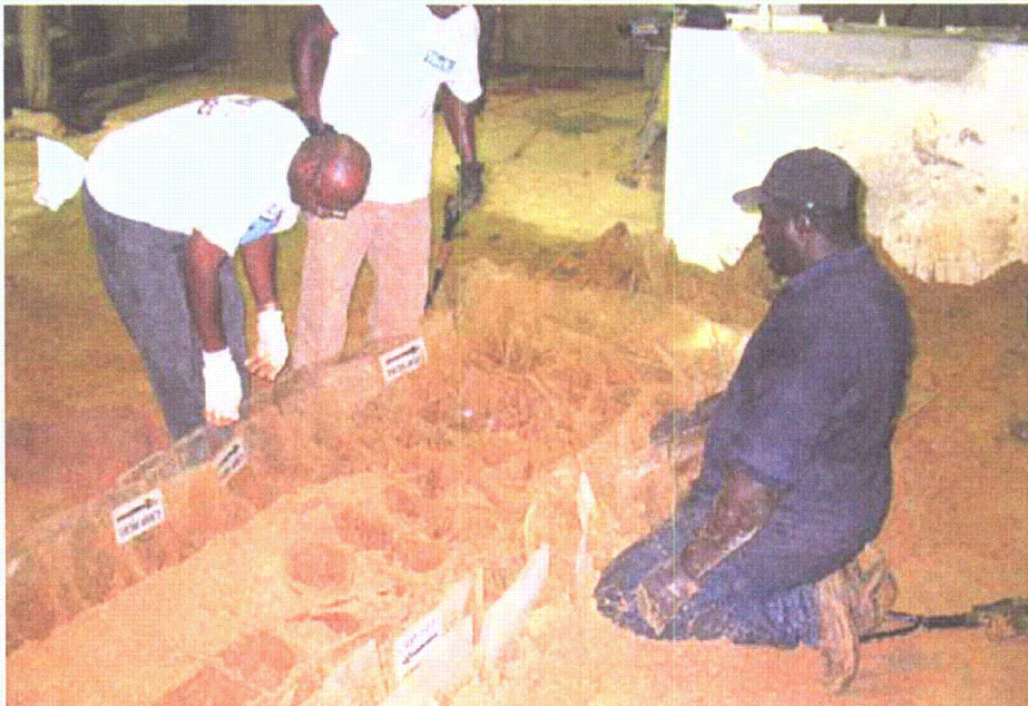
Figure 2-179. Preparing to remove one of second layer grid units. Note bandaged wrists to prevent cuts and scrapes from grid units
