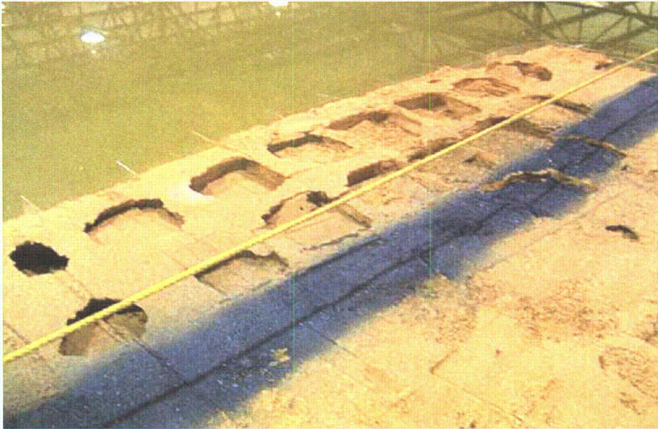
Figure 2-131. Sand subsidence in outer grid cells along center wall
