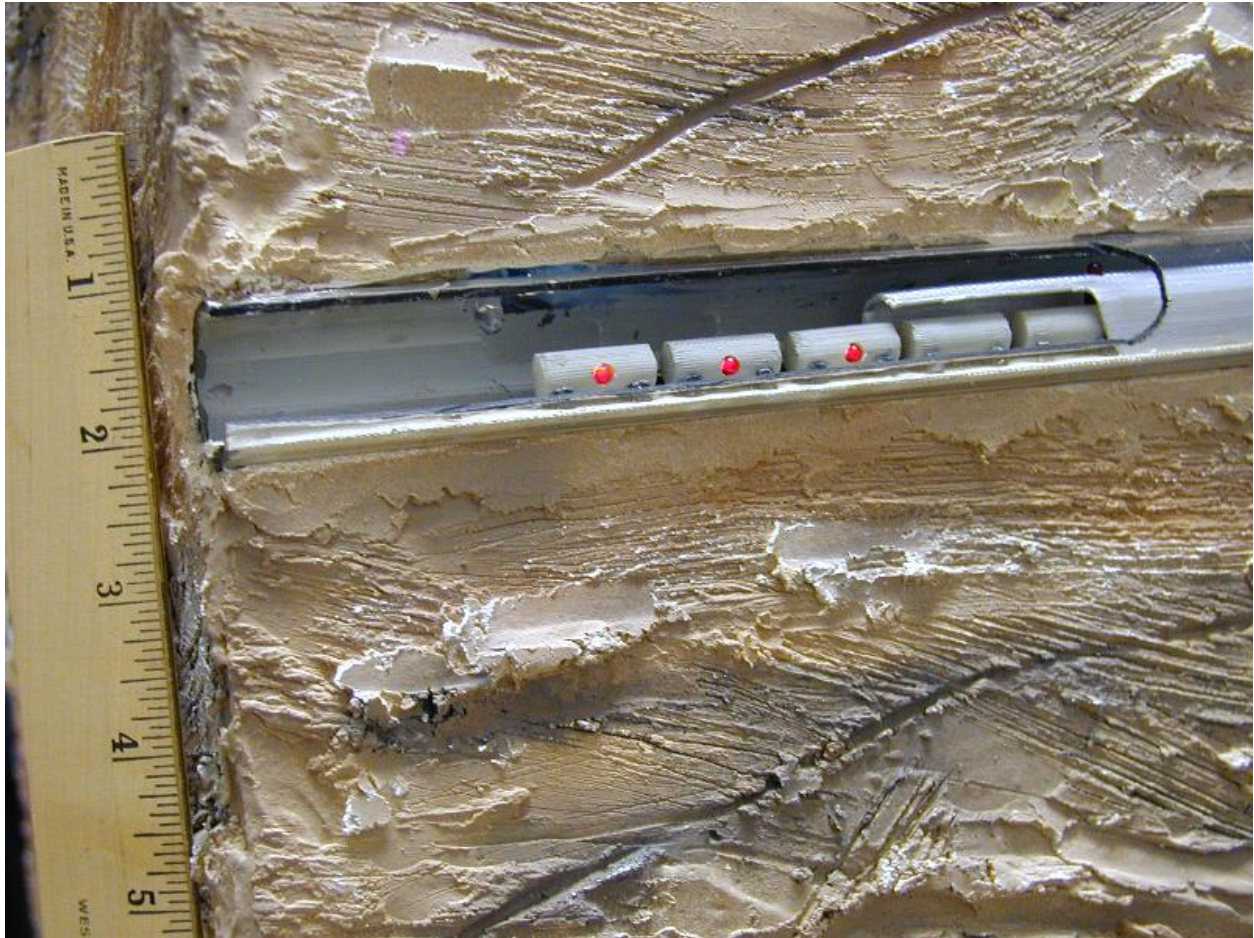
Figure 13. A Cutaway Area of a “Drift” on the 3D Model Showing Model Waste Packages and the LED Indicator Lights
