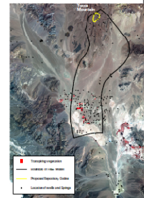
Geological, hydrological, and biological data are converted to numerical form and merged with information on manmade features to allow site characteristics analysis. High-precision data integration supports robust CNWRA flow and transport interpretations.
