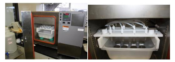
Figure 2-1. Experimental Setup for Dripping Test
