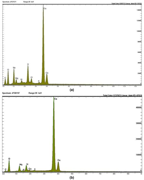
Figure 3-5. Energy-Dispersive X-ray Spectroscopy of the Salts Deposited on the 316L Stainless Steel Specimen Tested (a) at 80 °C [176 °F] and 85 Percent Relative Humidity and (b) at 95 °C [203 °F] and 75 Percent Relative Humidity
