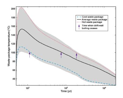
Figure 1-1. Range of Waste Package Temperature Versus Time Modeled for the Proposed Yuca Mountain Repository (Sandia National Laboratories, 2008)
