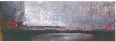
Weld separation from axial overload
