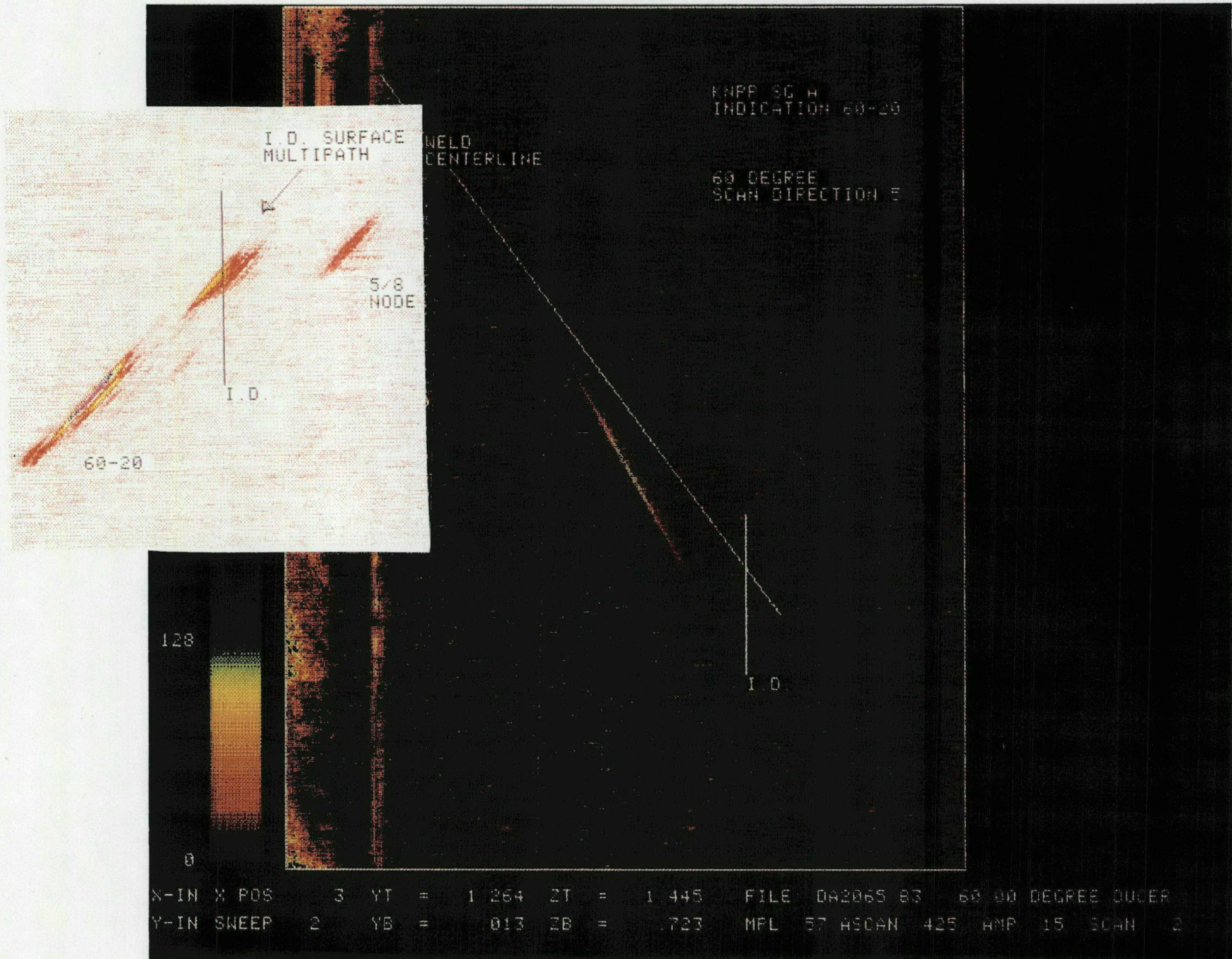
FIGURE A-25 S.G. A INDICATION 60-20, 60 DEGREE SCAN WITH 45 DEGREE HI-RES SCAN (INSERT)
