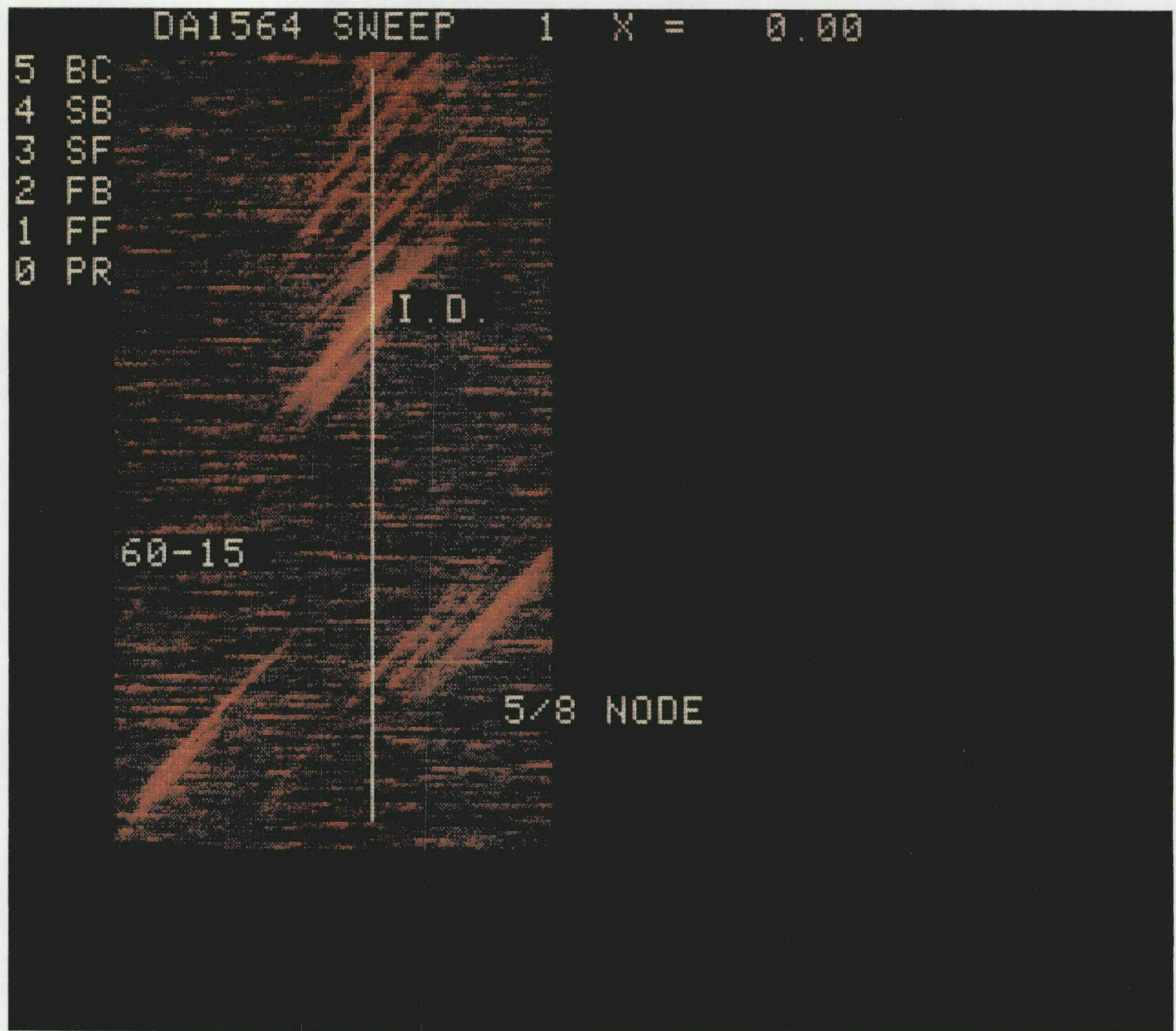
FIGURE A-21.2 S.G. A INDICATION 60-15, 45 DEGREE HI-RES SCAN
