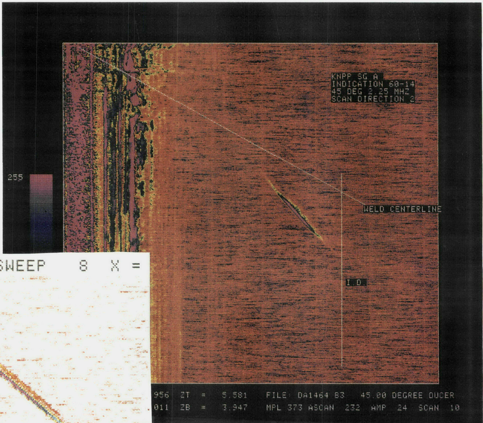
FIGURE A-20 S.G. A INDICATION 60-14, 45 DEGREE SCAN WITH 45 DEGREE HI-RES SCAN (INSERT)
