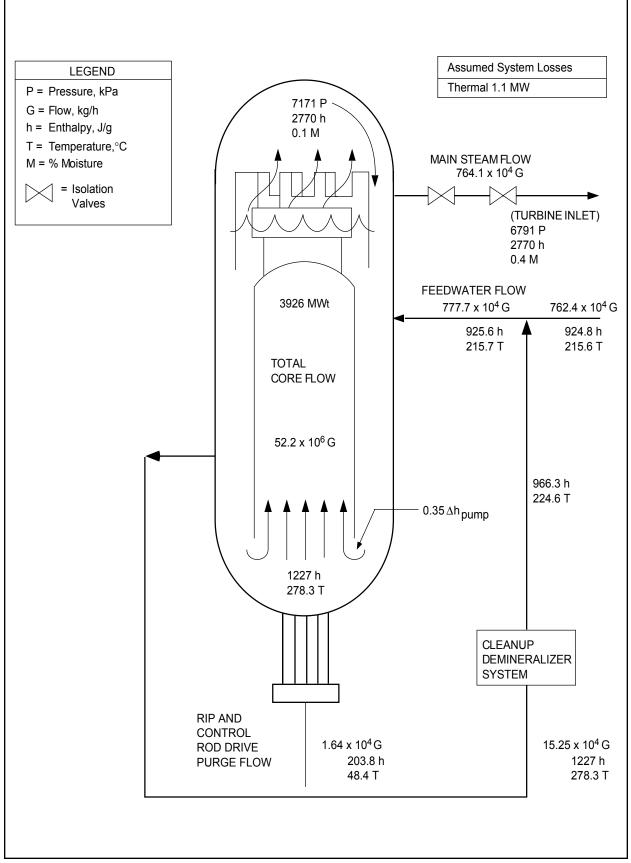
Figure 1.1-2 Heat Balance at Rated Power
