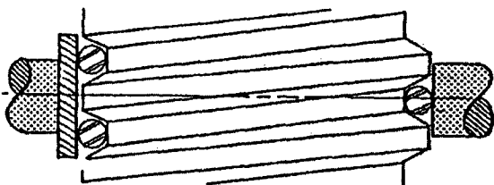
FIG. 3 EXTERNAL MINOR DIAMETER (NOTE WIRES REST ON ROOT AND PROTRUDE BEYOND CREST)
