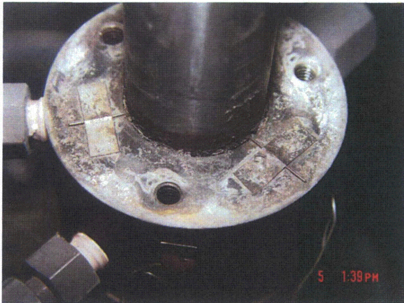
Figure 85. Top view of 20-mil gap crevice after removal of Ni foam and retaining ring, showing the magnetite powder in the crevice after the NaCl-03 and -04 tests.
