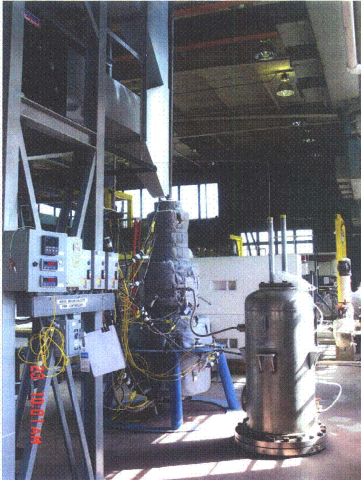
Figure 5. Photograph showing the MB equipped with insulation and instrumentation and a discharge collection tank.
