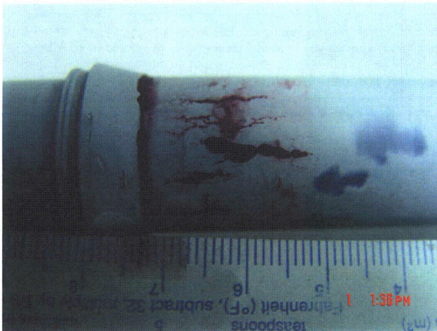
Figure 106. Axial cracks developed inside the unpacked crevice region and visually enhanced by dye penetration.
