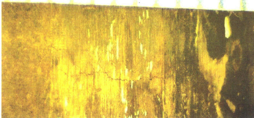
Figure A25. Photograph of crevice SCC OD flaw MB1-3 after leak testing at 8.3 MPa (1200 psi).
